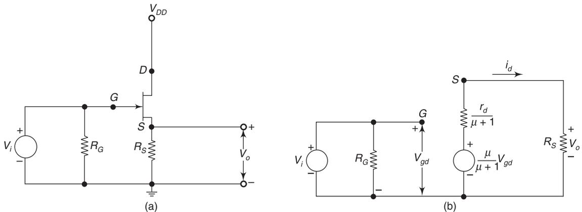
Fig. 3.3 (a) Common drain amplifier (b) Small-signal equivalent circuit of a CD amplifier
