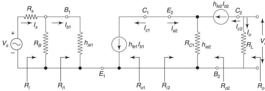
Fig. 2.28 Simplified h-parameter equivalent circuit of cascode amplifier
