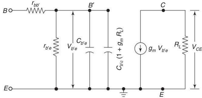
Fig. 4.26 Modified equivalent circuit
