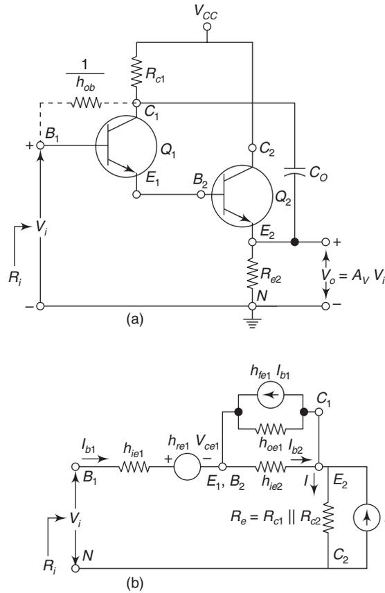
Fig. 2.34 (a) Bootstrapped Darlington circuit (b) Its equivalent circuit
