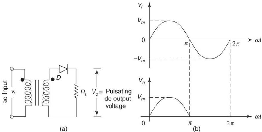
**Fig. 5.3** (a) Basic structure of a half-wave rectifier (b) Input output waveforms of half-wave rectifier
