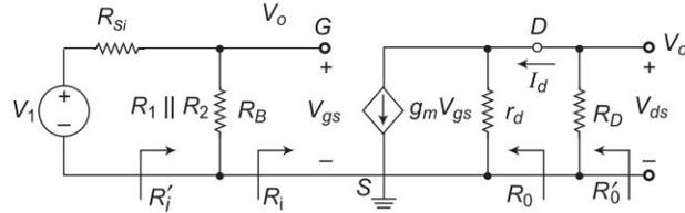
Fig. 3.17 Small signal equivalent circuit of common source amplifier
