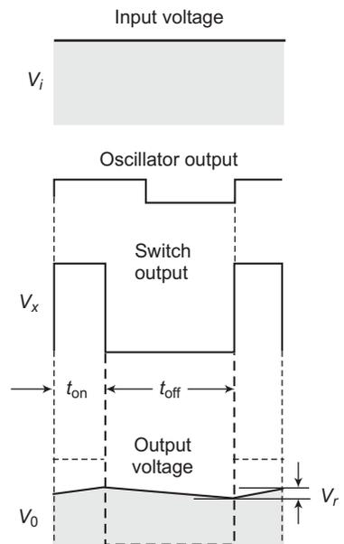
Fig. 5.33 Switching voltage waveforms
