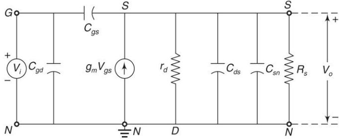
Fig. 4.40 Small-signal high-frequency equivalent circuit of common-drain amplifier
