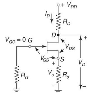
**Fig. 1.30** Self-bias circuit for an *N*-channel JFET
