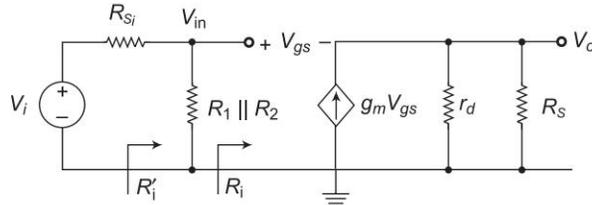
Fig. 3.19 (b) Equivalent circuit with all signal grounds connected to a common point
