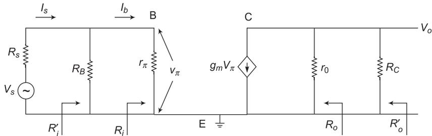
**Fig. 2.2** Small signal hybrid- $\pi$  equivalent circuit for CE amplifier
