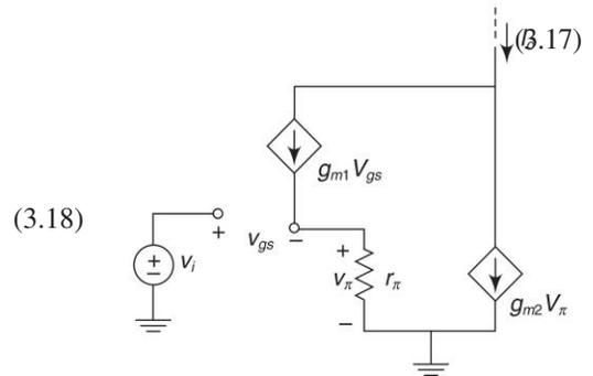
Fig. 3.31 Small signal equivalent circuit, BiCMOS Darlington pair configuration
