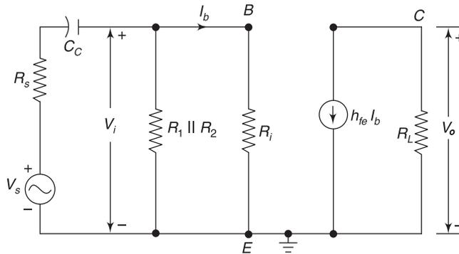
**Fig. 4.20** Low-frequency model for CE amplifier with coupling capacitor
