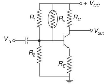
Fig. 1.22 Sensistor-bias compensation
