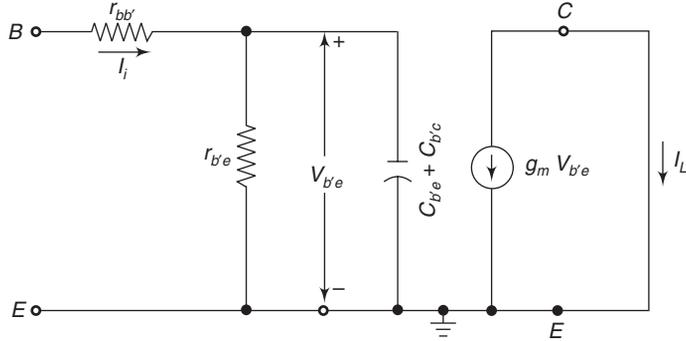
**Fig. 4.23** Approximate high-frequency circuit for determination of short-circuit current gain
