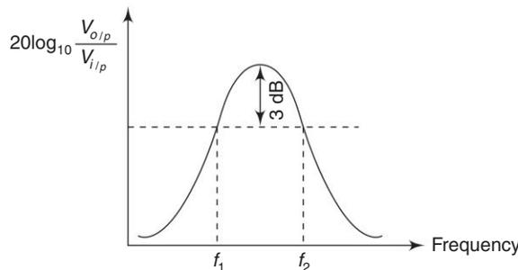
**Fig. 4.4** Power gain frequency to determine half-power bandwidth
