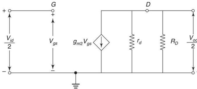
**Fig. 3.28** Half-circuit model with differential mode
