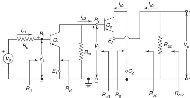
(a) ac equivalent circuit of CE-CC amplifier
