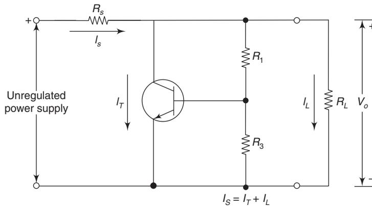
Fig. 5.26 Transistorized shunt regulator
