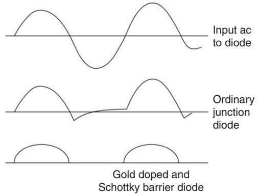
**Fig. 5.43** Behaviour of ordinary junction and gold-doped diodes at high frequency
