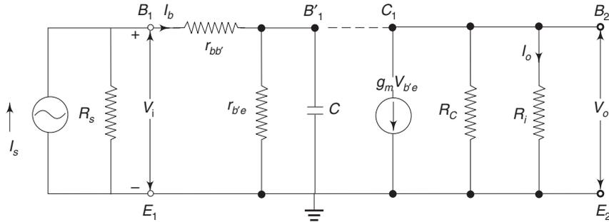
Fig. 2.24 Equivalent circuit of RC coupled amplifier in high-frequency range
