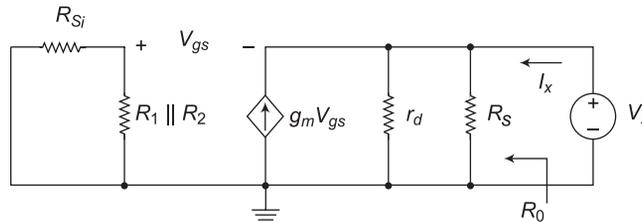
Fig. 3.20 Equivalent circuit of common drain amplifier to determine the output resistance
