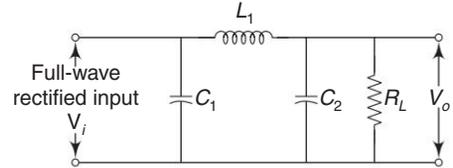
Fig. 5.12 CLC or  $\pi$ -type filter
