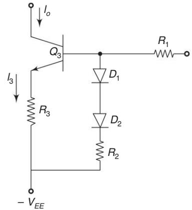
**Fig. 2.43** Modified constant current source using two diodes
