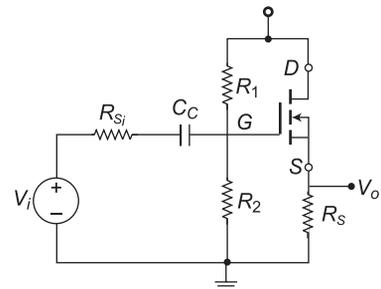
**Fig. 3.18** Common drain E-MOSFET amplifier
