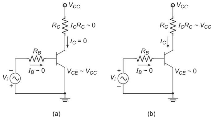
Fig.1.26 Direct-coupled BJT switching circuit in (a) OFF state and (b) ON state
