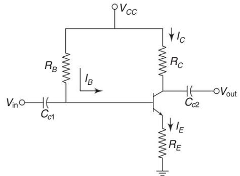
**Fig. 1.11** Emitter-feedback bias circuit
