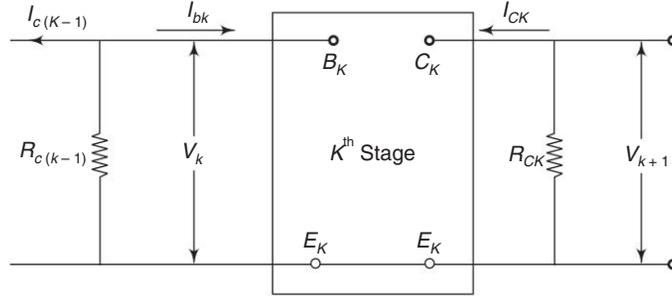
Fig. 2.12  $K^{\text{th}}$  stage of a cascaded amplifier
