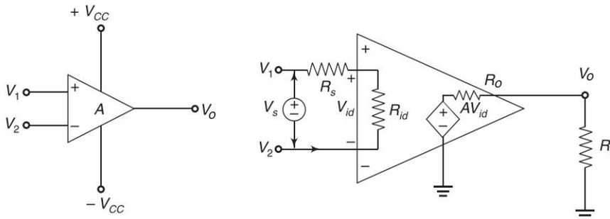
**Fig. 2.36** (a) Schematic form of basic differential amplifier (b) For signal analysis
