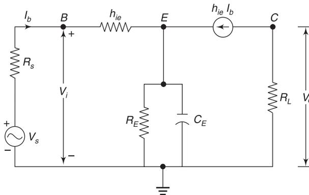
Fig. 4.19 Simplified  $h$ -parameter equivalent circuit for CE amplifier
