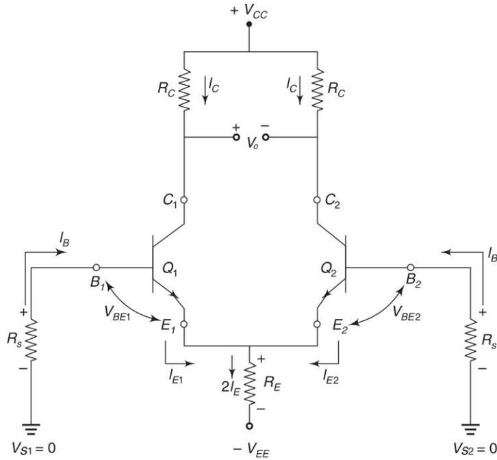
Fig. 2.38 dc equivalent circuit
