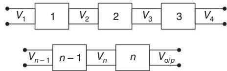
Fig. 4.3 n-stage cascaded system
