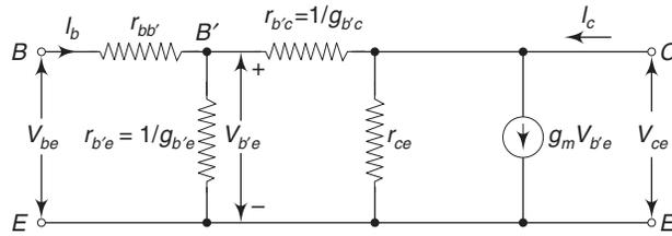
Fig. 4.22 (a) Hybrid- $\pi$  model for a common-emitter transistor at low-frequency
