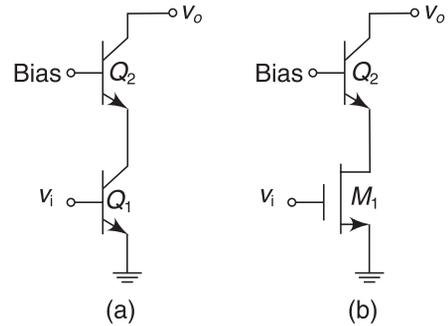
Fig. 3.32 (a) Bipolar cascode configuration (b) BiCMOS cascode configuration
