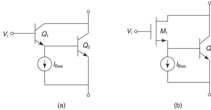
Fig. 3.30 (a) Darlington pair configuration using BJTs and (b) Darlington pair configuration of BiCMOS
