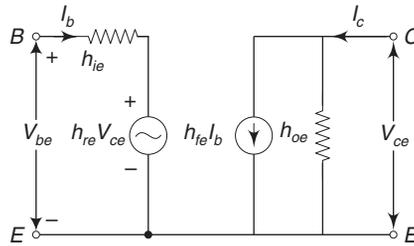
Fig. 4.22 (b)  $h$ -parameter model for a common-emitter transistor at low-frequency
