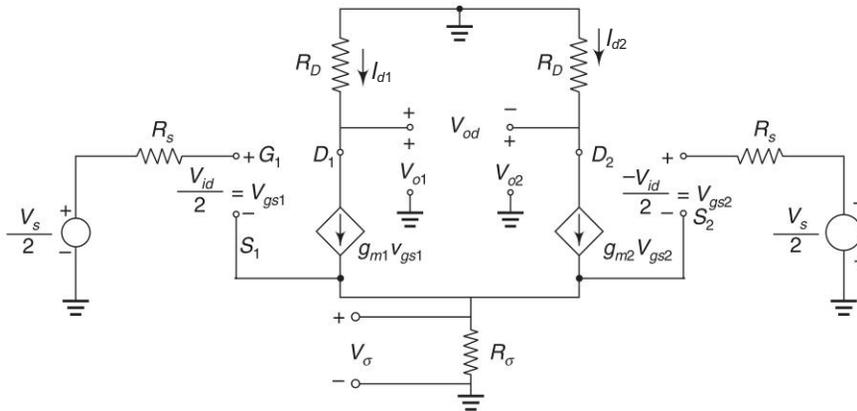
**Fig. 3.27** Small-signal mode with differential input
