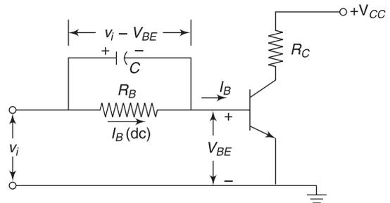
Fig. 4.43 Transistor circuit with the speed-up capacitor
