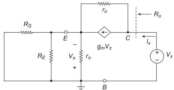
**Fig. 2.7** CB equivalent circuit for calculating output resistance
