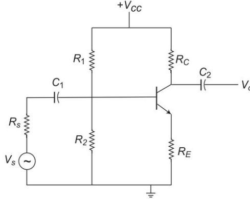
**Fig. 2.3** CE amplifier with unbypassed  $R_E$
