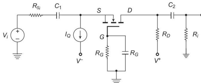
Fig. 3.21 Common gate E-MOSFET amplifier
