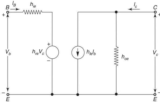
Fig. 3.6  $h$ -parameter model of BJT in CE configuration
