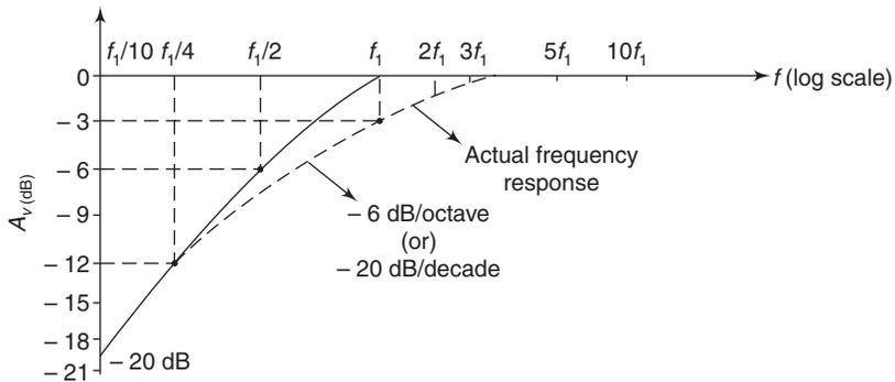
**Fig. 4.12** Bode plot for the low-frequency region
