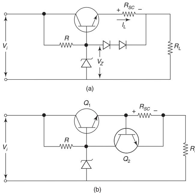
Fig. 5.23 (a) and (b) Overload protection circuit
