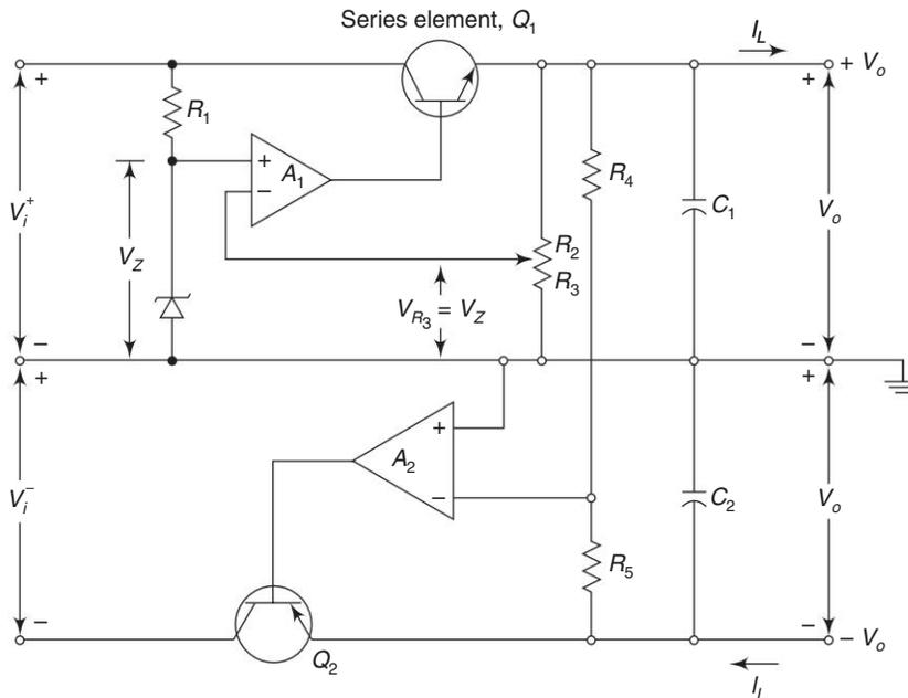
Fig. 5.25 Dual-tracking voltage regulator using op-amps
