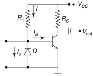
**Fig. 1.25** Diode-bias compensation
