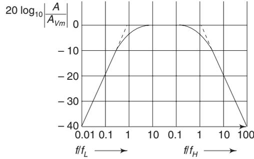
Fig. 2.25 Plot of gain versus frequency for an RC coupled amplifier
