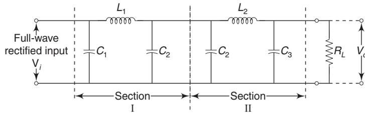
Fig. 5.13 Multiple  $\pi$ -section filter
