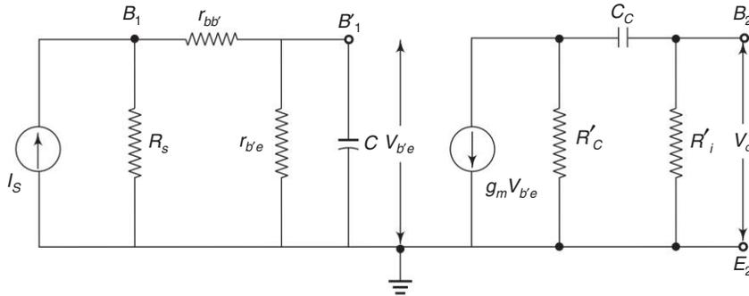
Fig. 2.20 Simplified equivalent circuit of an RC coupled amplifier
