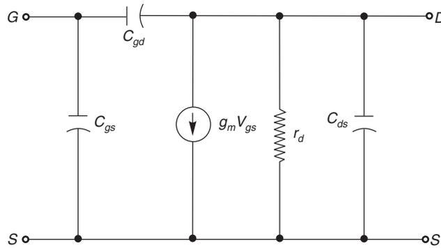
Fig. 3.7 High-frequency model of FET
