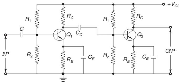
**Fig. 2.16** A two-stage RC coupled amplifier
