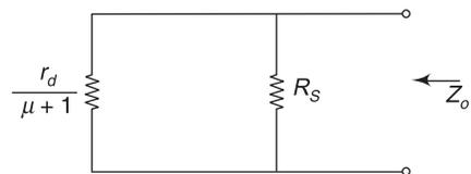
Fig. 3.3 (c) Calculation of output impedance
