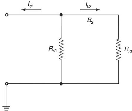
(b) Relating to the calculation of overall current gain
