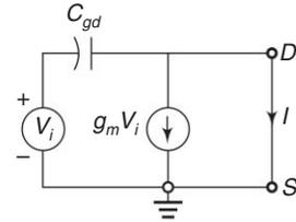
Fig. 4.36 Equivalent circuit to find  $I$
