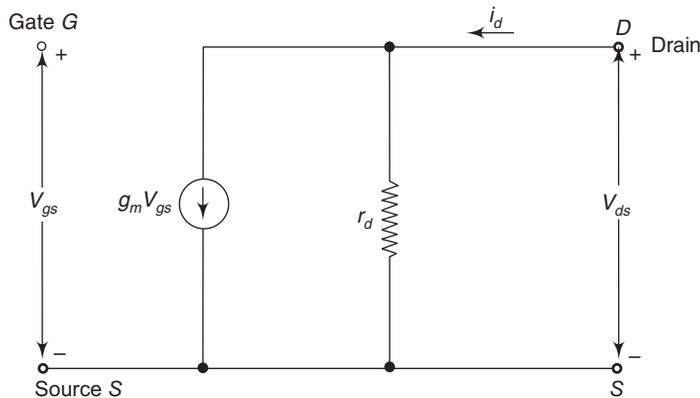
**Fig. 3.5** Small-signal model for FET in CS configuration
