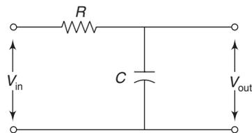
Fig. 4.17 Typical low pass RC network
