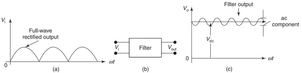
Fig. 5.6 Concept of a filter
