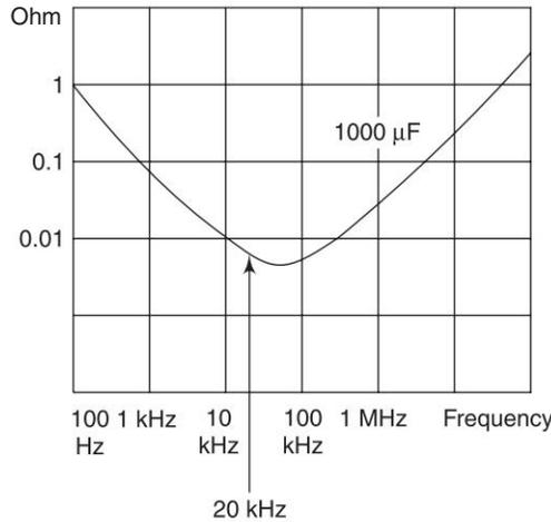
**Fig. 5.44** Variation of impedance of capacitor
