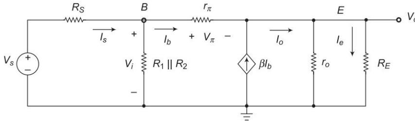
Fig. 2.9 Small signal hybrid- $\pi$  equivalent circuit for CC amplifier
