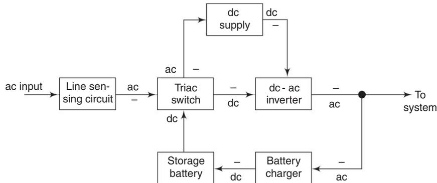
**Fig. 5.42** Block diagram of standby power supply
