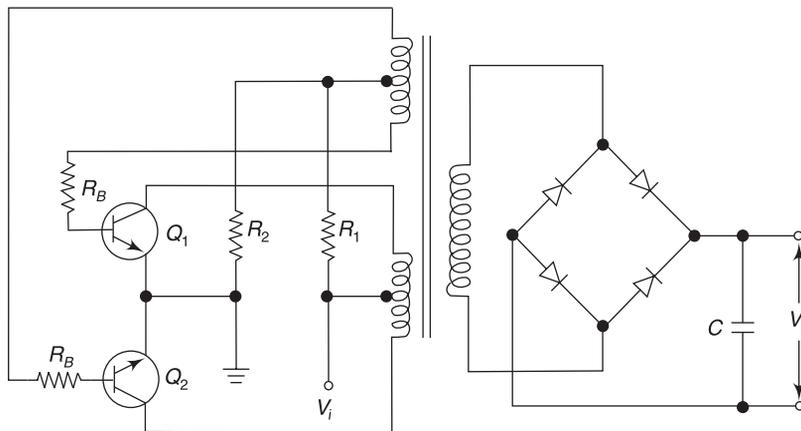
Fig. 5.41 Push-pull converter
