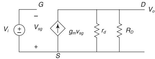
**Fig. 3.13** Small signal equivalent circuit of common source amplifier with PMOS transistor model
