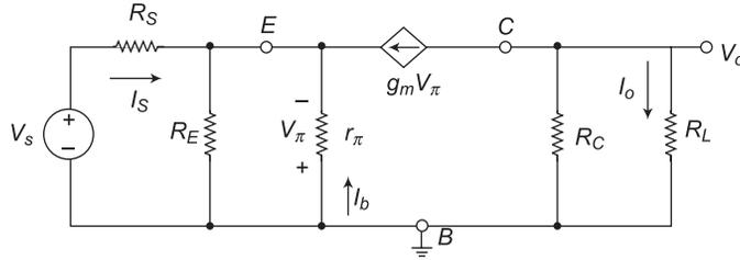
**Fig. 2.6** Small signal hybrid- $\pi$  equivalent circuit for CB amplifier
