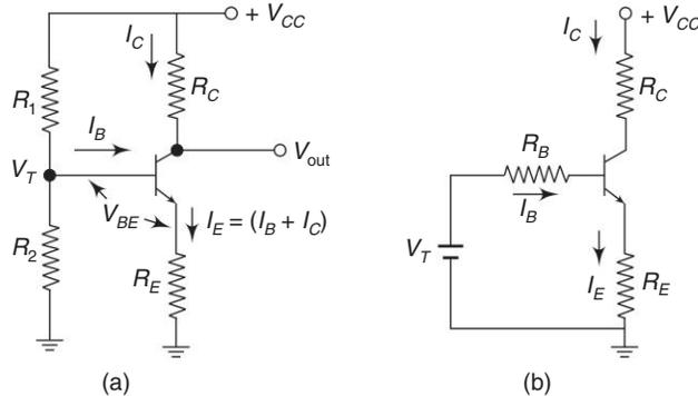
Fig. 1.16 (a) Self-bias circuit (b) Thevenin's equivalent circuit
