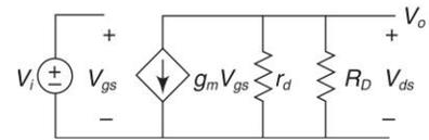
**Fig. 3.10** Small Signal equivalent circuit of common source circuit with NMOS transistor model
