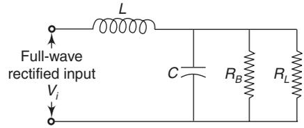
**Fig. 5.10** Bleeder resistor connected at the filter output
