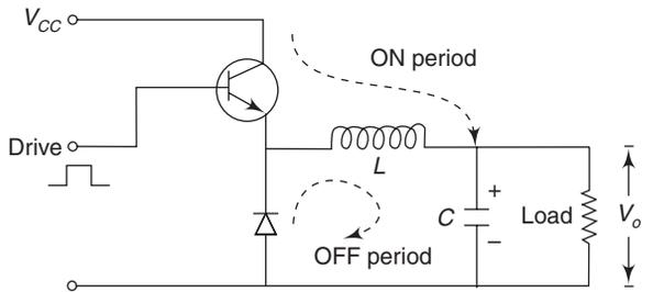
**Fig. 5.37** Circuit diagram of a forward step down converter
