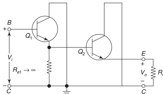
Fig. 2.31 Darlington circuit with two cascaded CC stages
