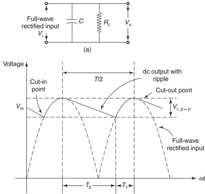
**Fig. 5.8** (a) Capacitor filter (b) Ripple voltage triangular waveform
