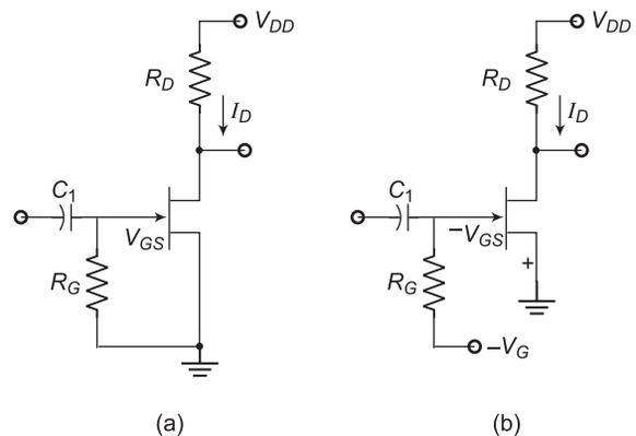
Fig. 1.47 Capacitor-coupled JFET switching circuit in (a) ON state and (b) OFF state
