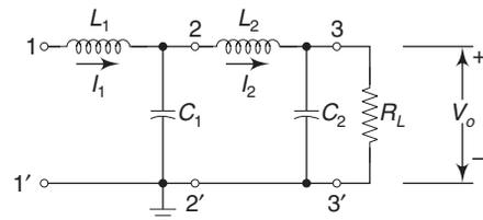
Fig. 5.11 A multiple (two-section) L-section filter
