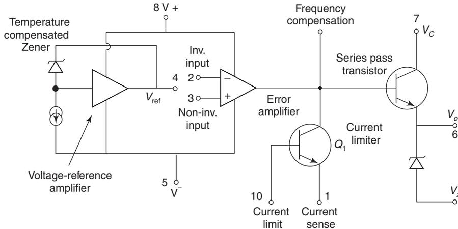
Fig. 5.30 Internal circuit of LM 723C
