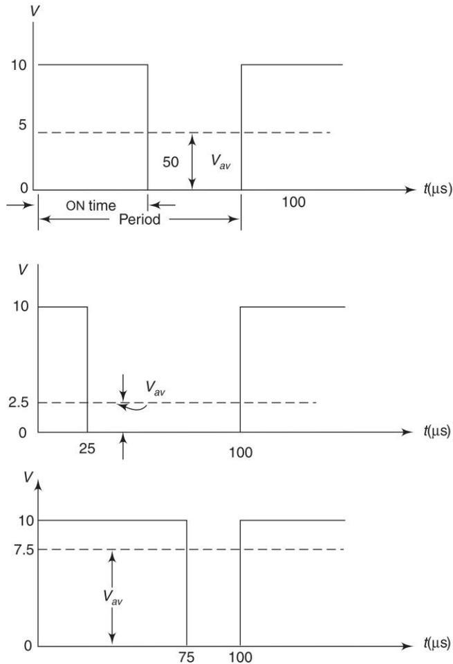
**Fig. 5.35** Pulse width modulation and average value
