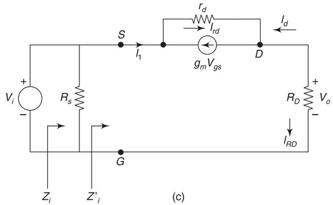
**Fig. 3.4** (c) Modified equivalent circuit
