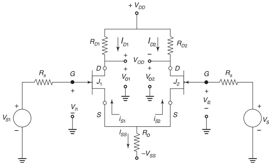
Fig. 3.24 Source coupled differential amplifier
