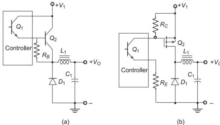
Fig. 5.34 Over-voltage protection circuit of step-down converter using (a) BJT and (b) MOSFET
