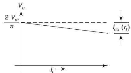
**Fig. 5.15** Load regulation characteristics
