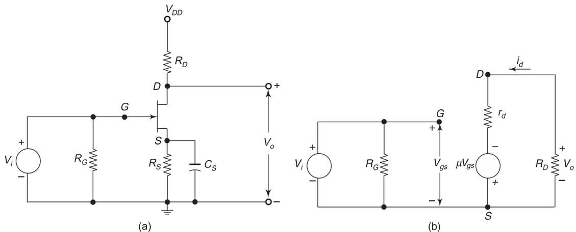
**Fig. 3.2** (a) Common source amplifier (b) Small-signal equivalent circuit of CS amplifier
