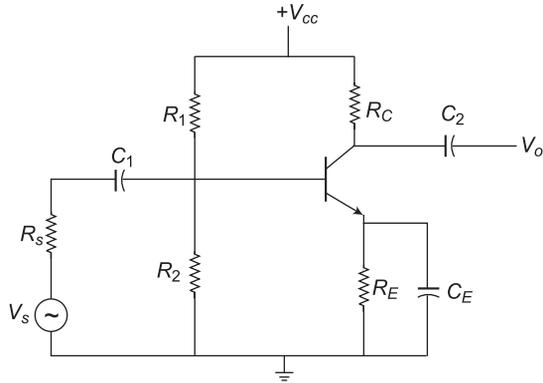
**Fig. 2.1** CE amplifier with bypassed  $R_E$
