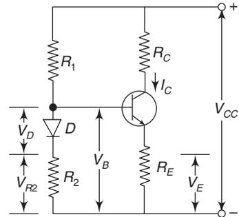
**Fig. 1.24** Diode compensation in voltage-divider bias circuit
