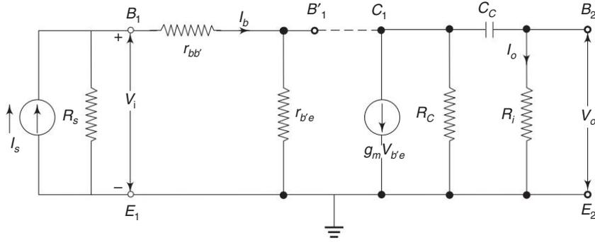
**Fig. 2.23** Simplified equivalent circuit of an RC coupled amplifier in the low-frequency range
