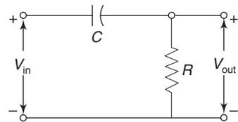
**Fig. 4.8** Equivalent circuit for lower cut-off frequency analysis
