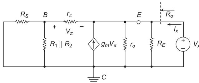
Fig. 2.10 CC equivalent circuit for calculating output resistance
