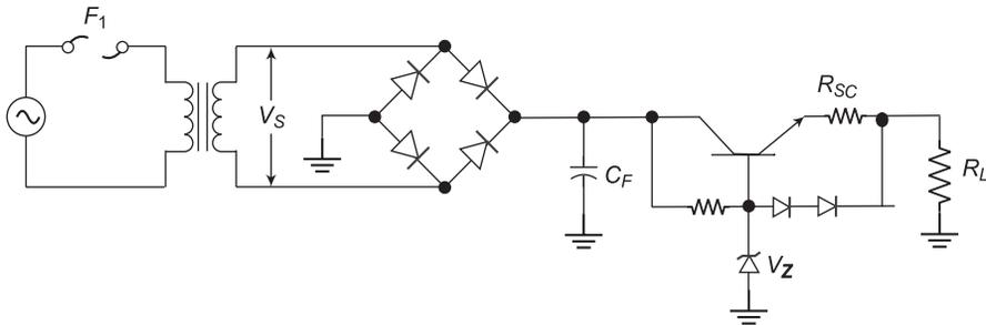
**Fig. 5.45** Basic linear power supply circuit diagram
