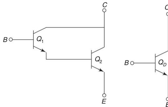
**Fig. 2.29** (a) Darlington transistor connection (b) Single Darlington transistor
