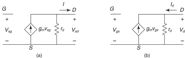
**Fig. 3.14** Small signal equivalent circuit of a P-Channel MOSFET showing (a) the conventional voltage polarities and current directions and (b) the case when the voltage polarities and current directions are reversed.
