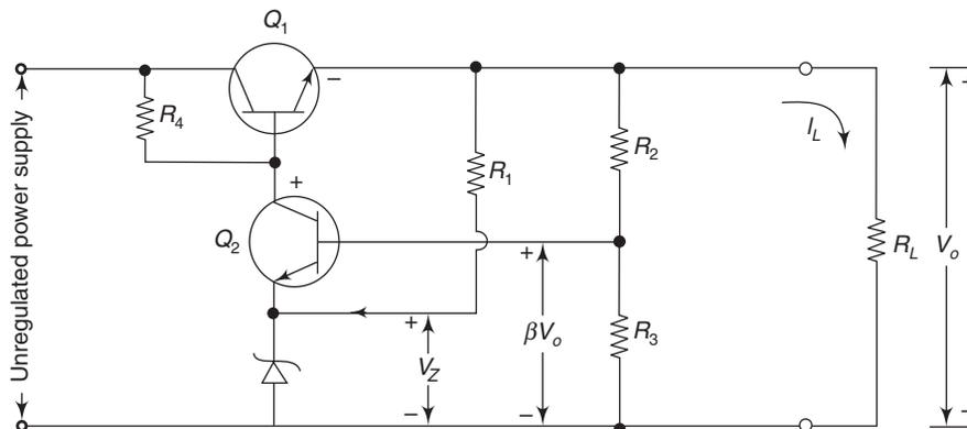
Fig. 5.27 Transistorized series regulator
