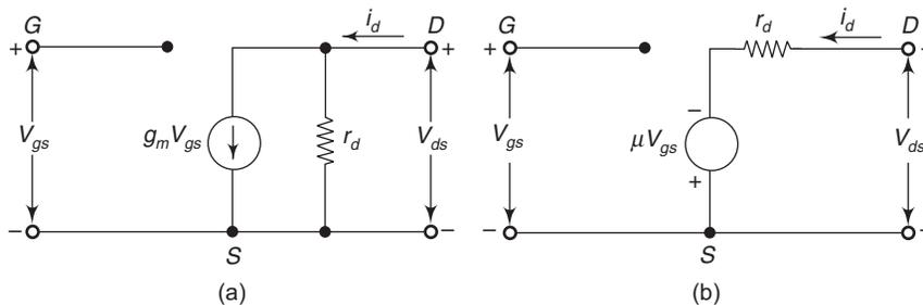
**Fig. 3.1** (a) Small-signal current-source model for FET in CS configuration
