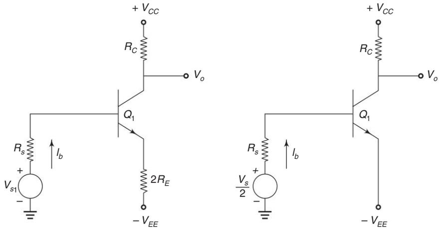
Fig. 2.39 Emitter-coupled pair for (a)  $A_c$  analysis, and (b)  $A_d$  analysis
