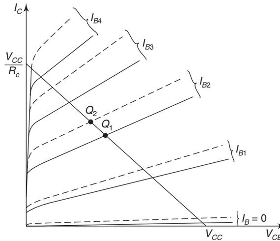
Fig. 1.1 Effect of  $\beta$  on  $Q$ -point
