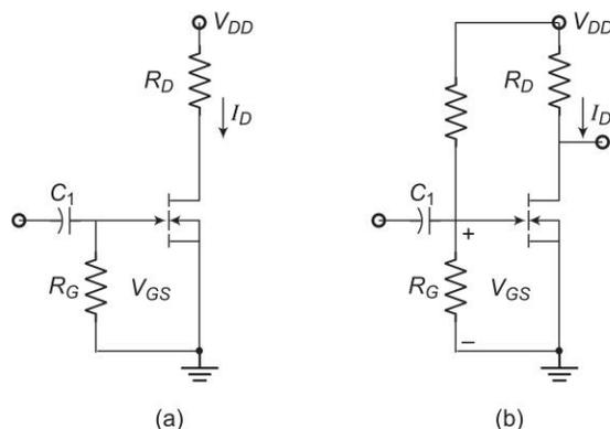
Fig. 1.48 Capacitor-coupled E-MOSFET switching circuit in (a) ON state and (b) OFF state
