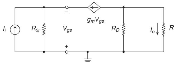
Fig. 3.23 Small signal equivalent circuit of common gate amplifier with Norton current source
