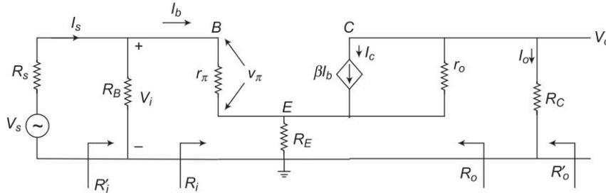
**Fig. 2.4** Small signal hybrid- $\pi$  equivalent circuit for CE amplifier with unbypassed  $R_E$
