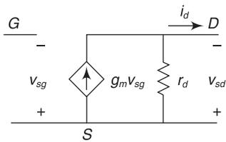
**Fig. 3.12** Small Signal equivalent circuit of PMOS Transistor
