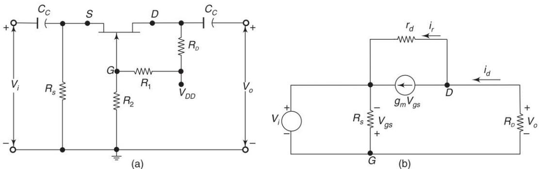
**Fig. 3.4** (a) Common-gate amplifier (b) Small-signal equivalent circuit of a CG amplifier
