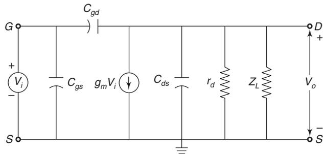
Fig. 4.34 Small-signal equivalent circuit of a CS amplifier at high frequencies
