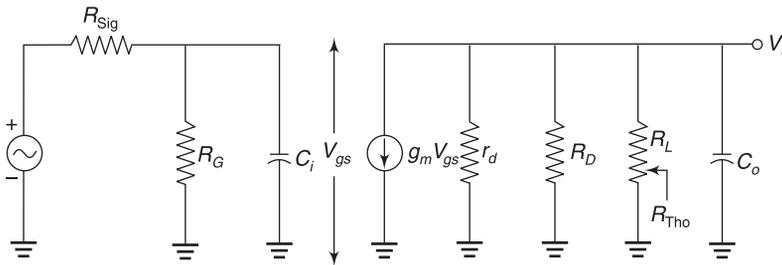
Fig. 4.41(a) Modified high-frequency ac equivalent circuit (CS amplifier)
