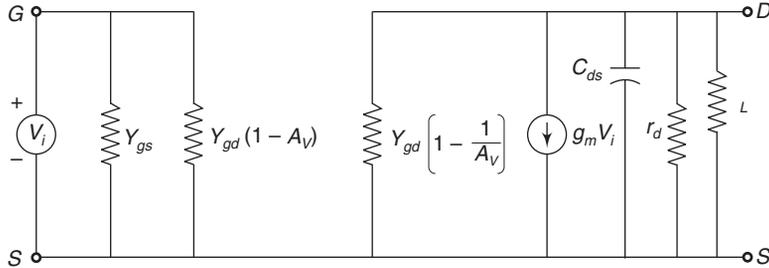
Fig. 4.37 CS amplifier equivalent circuit after applying Miller's theorem
