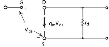
Fig. 3.15 Equivalent circuit model of Enhancement MOSFET
