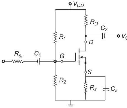
Fig. 3.16 Common source E-MOSFET amplifier
