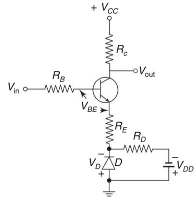
Fig. 1.23 Stabilization by voltage-divider bias compensation
