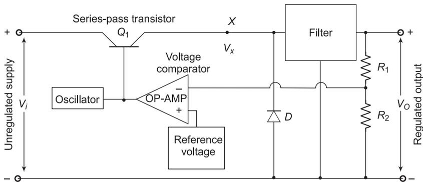
Fig. 5.32 Switching voltage regulator
