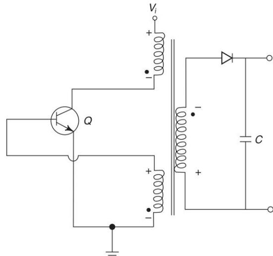
Fig. 5.40 Self-oscillating flyback converter
