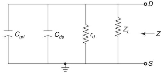
Fig. 4.35 Equivalent circuit to find  $Z$
