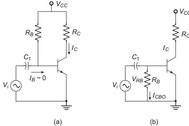
**Fig. 1.27(a)** Capacitor-coupled BJT switching circuit with the transistor biased normally in (a) ON state and (b) OFF state
