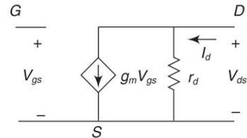
**Fig. 3.9** Expanded small signal Equivalent circuit, including output resistance for NMOS Transistor
