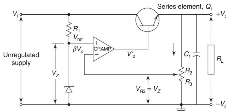
**Fig. 5.24** Basic circuit of a linear voltage regulator
