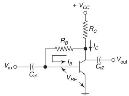
Fig. 1.13 Collector-to-base bias circuit
