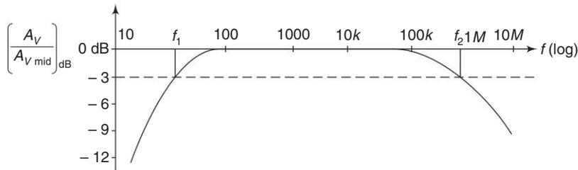
**Fig. 4.7** Decibel plot of the normalized gain versus frequency (logarithmic) of Fig. 4.6
