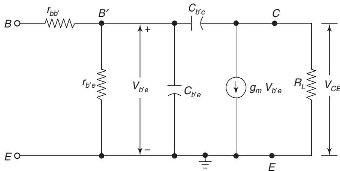
**Fig. 4.25** High-frequency equivalent circuit with resistive load
