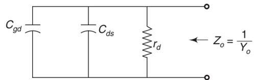
Fig. 4.38 Calculation of output impedance
