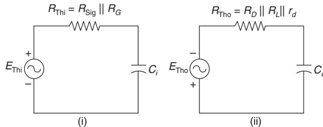
Fig. 4.41(b) Thevenin equivalent circuit for (i) Input circuit, and (ii) Output circuit
