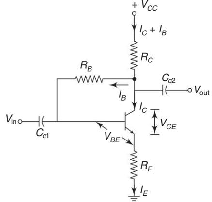
Fig. 1.15 Collector-emitter feedback circuit
