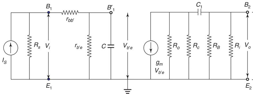
Fig. 2.19 Simplified equivalent circuit of an RC coupled amplifier
