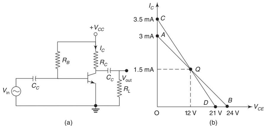
**Fig. 1.2** (a) Biasing circuit (b) CE output characteristics and load line
