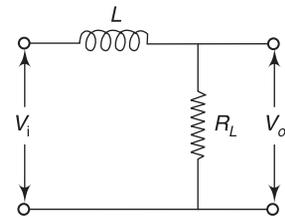
Fig. 5.7 Inductor filter
