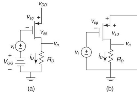
**Fig. 3.11** (a) Common Source circuit with PMOS transistor and (b) corresponding ac equivalent circuit.
