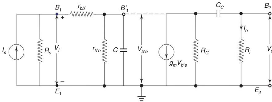
Fig. 2.21 Simplified equivalent circuit of an RC coupled amplifier
