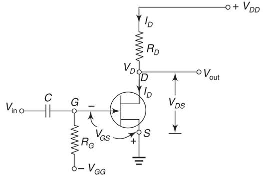
Fig. 1.32 Fixed bias circuit for an *N*-Channel JFET
