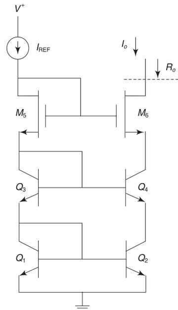
Fig. 3.33 BiCMOS Double cascode constant current source
