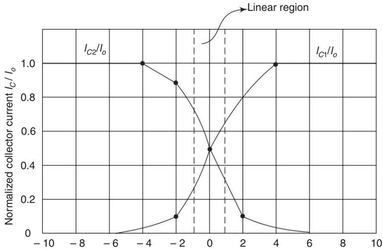
**Fig. 2.44** Transfer characteristics of the basic transistor based differential amplifier circuit (when Q1 is identically equal to Q2)
