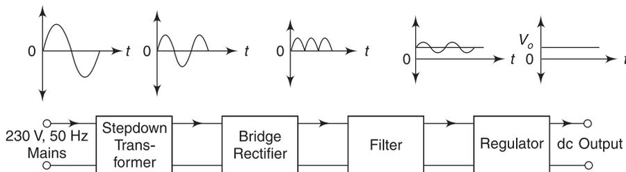
Fig. 5.2 Basic building block of linear-mode power supply
