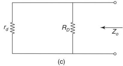
Fig. 3.2 (c) Calculation of output impedance
