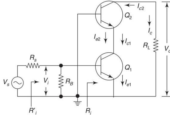
Fig. 2.27 ac equivalent circuit of cascode amplifier
