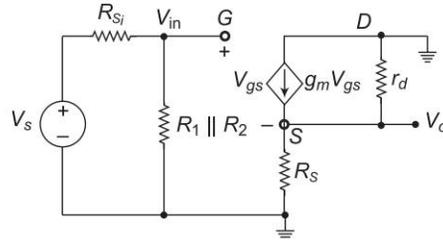
Fig. 3.19 (a) Small signal equivalent circuit of common drain amplifier
