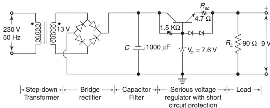
**Fig. 5.46** Designed circuit for 9 V, 100 mA output with short-circuit protection
