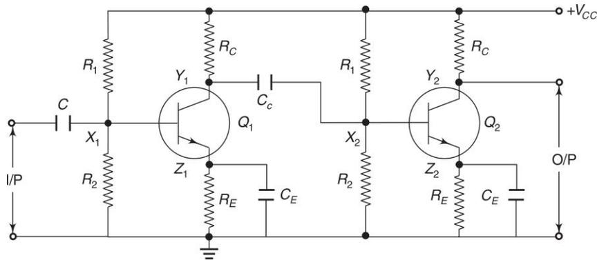
Fig. 2.15 A two-stage RC coupled amplifier
