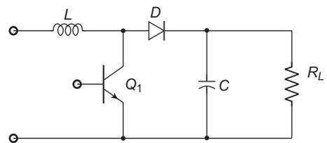
**Fig. 5.38** Circuit of step-up converter
