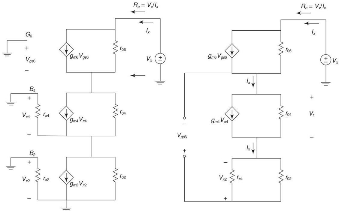
**Fig. 3.34** (a) Equivalent circuit to find output impedance of BiCMOS double cascade source and (b) its equivalent circuit
