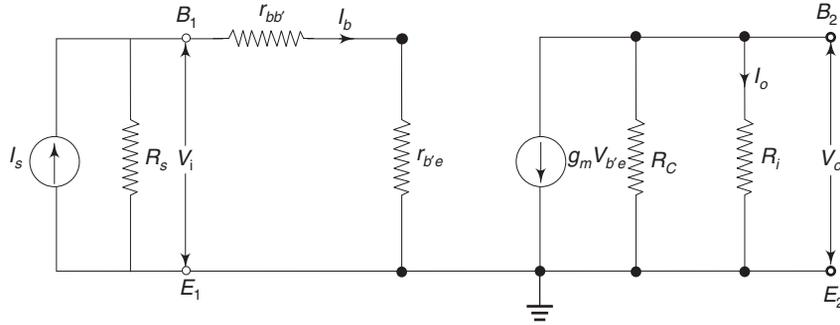
**Fig. 2.22** Simplified equivalent circuit of an RC coupled amplifier for mid-band range
