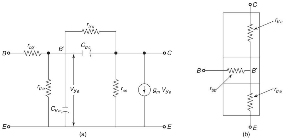
Fig. 4.21 (a) Hybrid- $\pi$  model for a transistor in the CE connection and (b) Virtual base  $B'$  and ohmic base-spreading resistance  $r_{bb'}$
