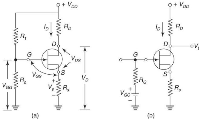
**Fig. 1.31** (a) Voltage-divider bias circuit (b) Thevenin's equivalent circuit
