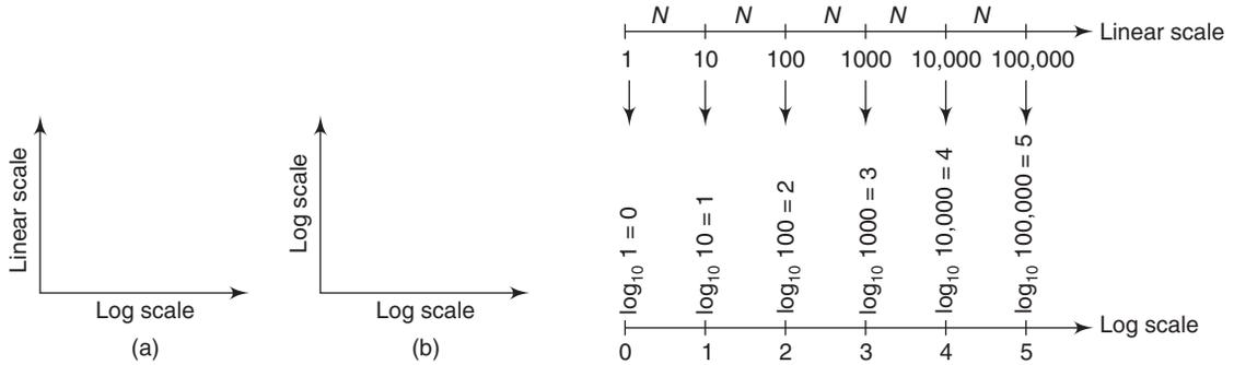
**Fig. 4.1** (a) Semilog graph and (b) Double-log graph
