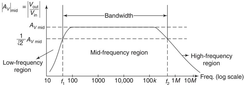
**Fig. 4.5** Gain vs frequency (logarithmic scale) of an RC-coupled amplifier
