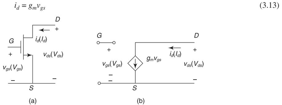
Fig. 3.8 (a) Common source NMOS transistor with small signal parameters (b) Simplified small signal equivalent circuit for NMOS Transistor
