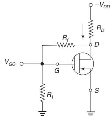
Fig. 1.33 Drain-to-gate bias circuit for enhancement MOSFET
