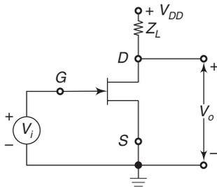
Fig. 4.33 CS amplifier circuit
