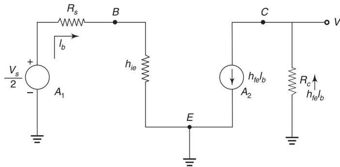
Fig. 2.40 Approximate hybrid model, neglecting  $h_{oe}$
