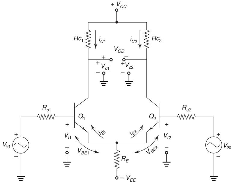
**Fig. 2.37** Circuit diagram of emitter-coupled differential amplifier
