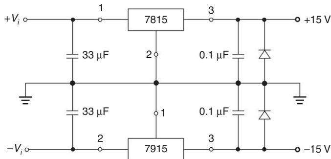
Fig. 5.29 Dual-tracking regulator
