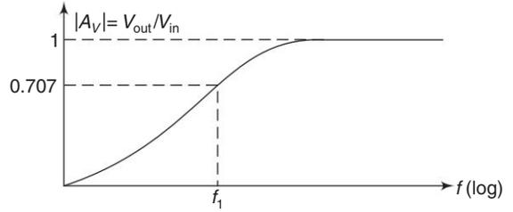
**Fig. 4.11**  $A_v$  vs frequency of a typical RC network
