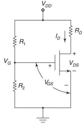
**Fig. 1.34**  $N$ -channel enhancement mode MOSFET common-source circuit with source resistor
