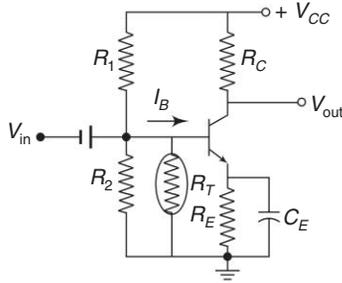
Fig. 1.21 Thermistor-bias compensation
