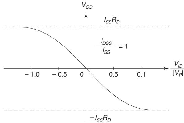
**Fig. 3.26** Differential output voltage of a common-source amplifier as a function of the differential input voltage ( $I_{SS} = I_{DSS}$ )
