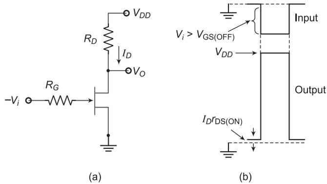
Fig. 1.46 JFET switching circuit (a) Direct-coupled circuit and (b) input/output waveforms
