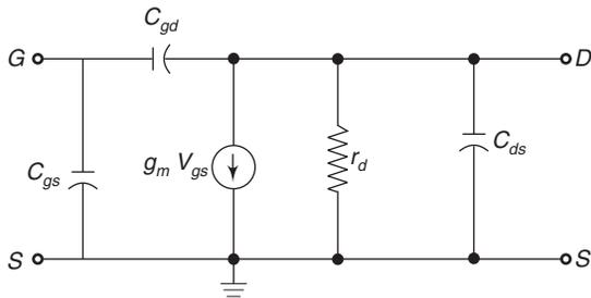
Fig. 4.32 The high-frequency model of FET
