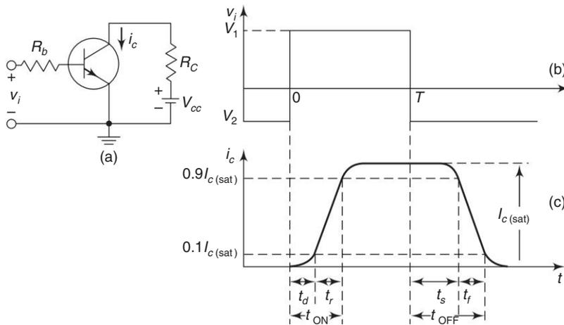
Fig. 4.42 (a) Transistor-switching circuit (b) Input-pulse waveform (c) Collector-current response
