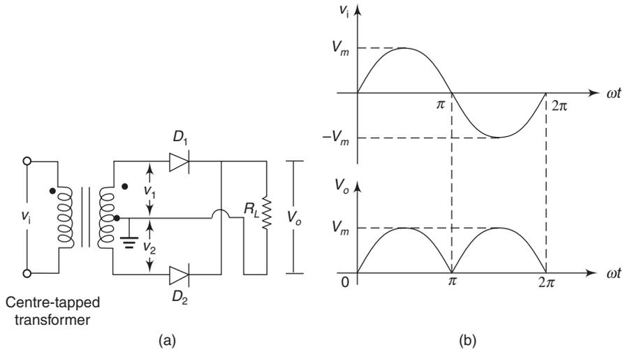
**Fig. 5.4** Full-wave rectifier
