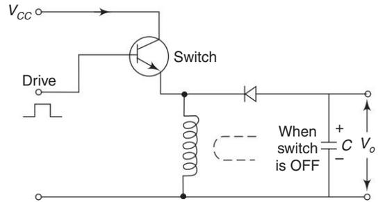
Fig. 5.39 Circuit diagram of a flyback converter
