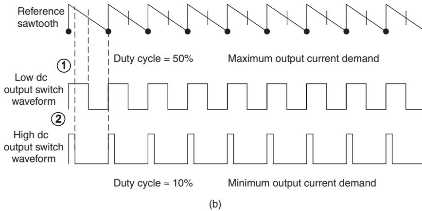
**Fig. 5.36** (a) Block diagram of switching power supply (b) Switching power supply waveforms
