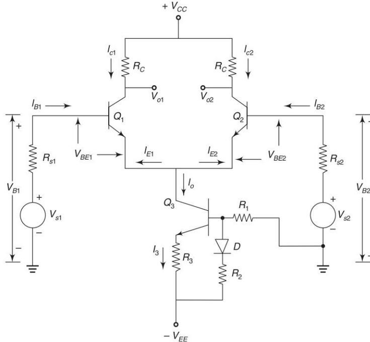
**Fig. 2.42** Differential BJT amplifier with active loading
