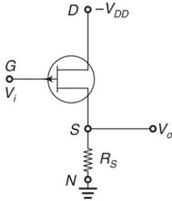
Fig. 4.39 Common-drain amplifier
