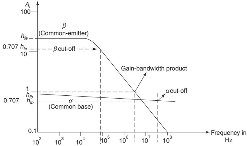
Fig. 4.24 Variation of  $A_i$  with frequency for CE and CB amplifiers
