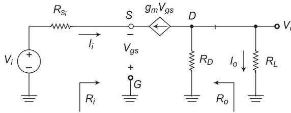
Fig. 3.22 Small signal equivalent circuit of common gate amplifier
