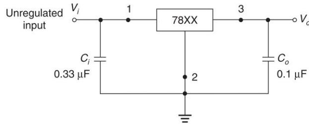
Fig. 5.28 Monolithic voltage regulator
