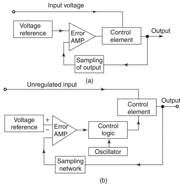
Fig. 5.1 (a) Principle of a normal linear mode power supply, (b) Block diagram of a switched mode power supply
