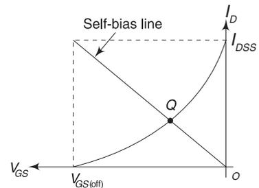
**Fig. 1.29** Self-bias line through  $I_{DSS}$  and  $V_{GS(off)}$
