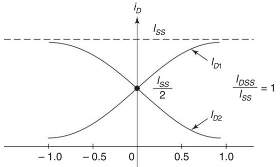
**Fig. 3.25** Drain current of a source-coupled pair as a function of the differential input voltage  $I_{SS} = I_{DSS}$
