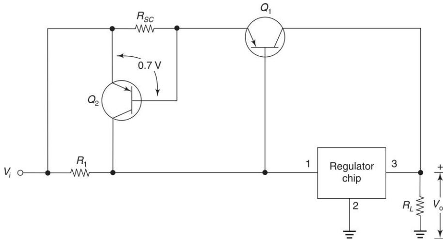
Fig. 5.31 Regulator with current limiting
