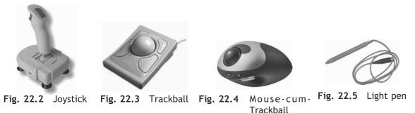
**Light pen** A light pen, Fig. 22.5, is a light-sensitive input device used directly on the computer's CRT monitor. The pen, when placed against the screen, detects light from the screen enabling the computer to identify the location of the pen on the screen. Thus, it can be used to select the menus or draw directly on the screen. A light pen can work with any CRT-based monitor, but not with LCD screens, projectors or other display devices.
