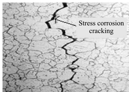
FIGURE 4.13 Stress corrosion cracking
