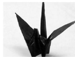
FIGURE 19.19 A macroscopic aggregate of carbon nanotubes is called 'buckypaper'.
