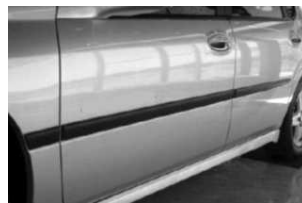
FIGURE 19.49 Car side mouldings with nanoclay
