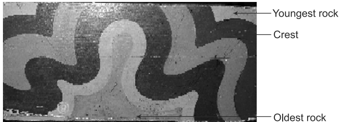
Geological Model 6: Fan fold
