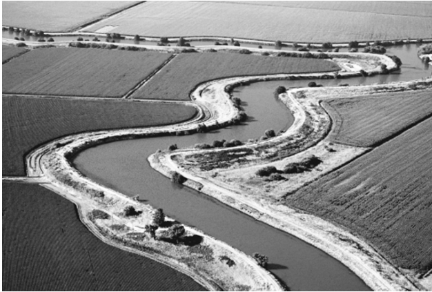
Fig. 10.10 Natural levees produced by a river
