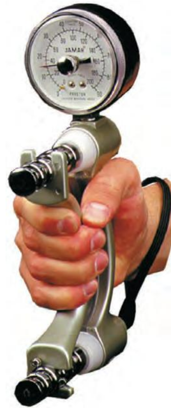
Figure 20.12 Use of the typical hand-grip dynamometer. Photo courtesy of Lafayette Instrument Company.
