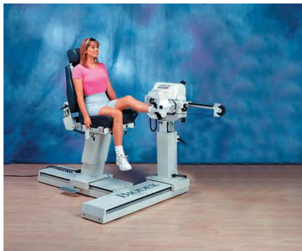
Figure 20.11 Use of a commercially available tensiometer to measure static force during a knee extension. Photo courtesy of Biodex Medical Systems, Inc.
