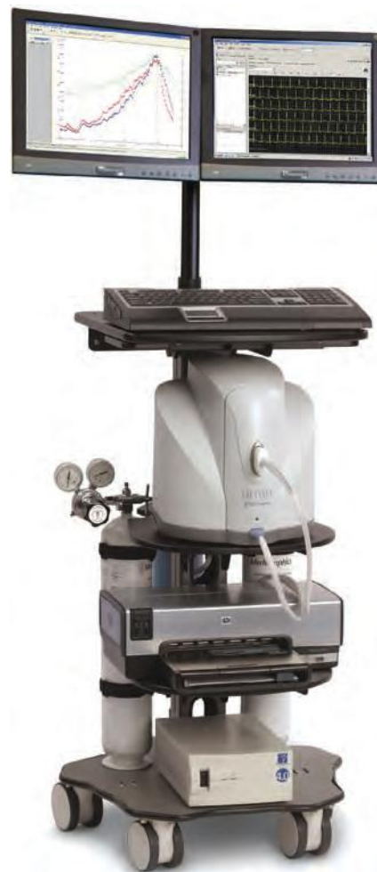
Figure 6.4 Modern systems for the measurement of pulmonary gas exchange utilize electronic flow sensors, gas analyzers, and computer technology. These devices are used to measure oxygen uptake and carbon dioxide production at rest and during exercise. Source: Medical Graphics Corporation
