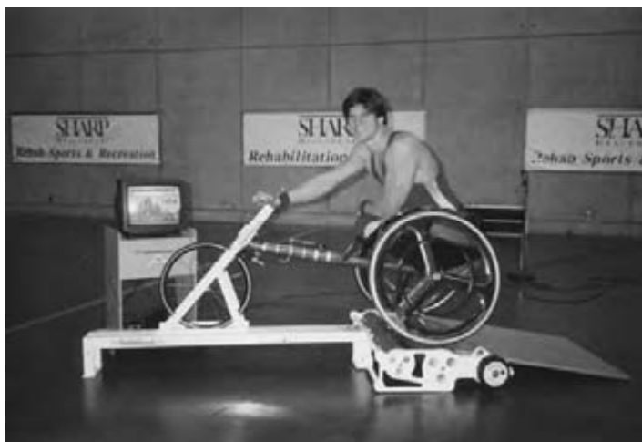
Specialized fitness equipment has been developed to meet the needs of athletes in wheelchairs. This resistance trainer, created by D & J Development, has an interactive computer that simulates road racing conditions.
