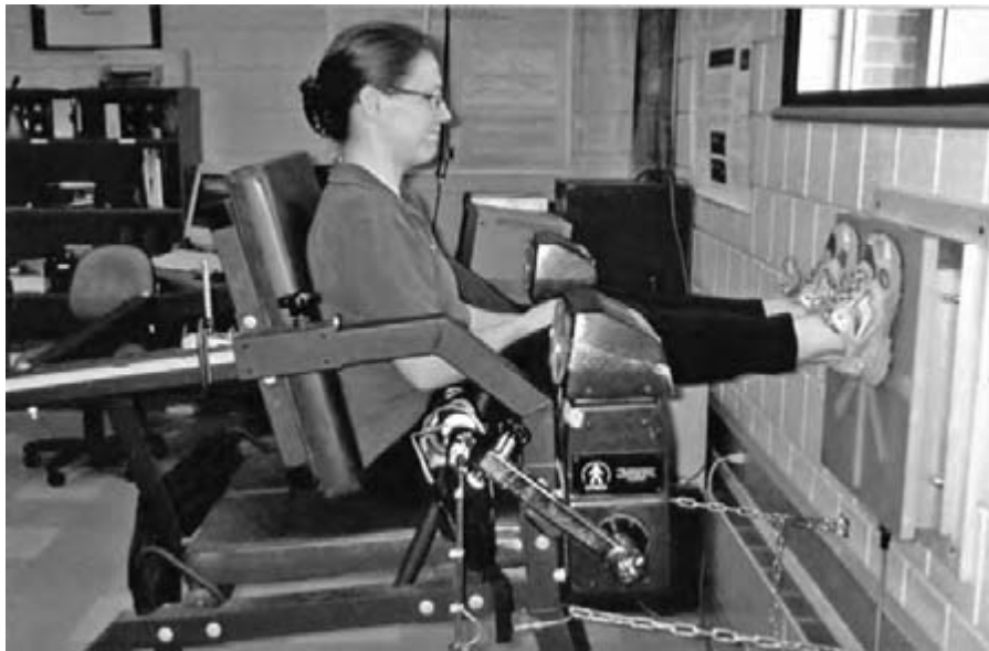
Leg press strength is being measured with a force plate attached to a wall. The force plate is connected to a computer where peak force and rate of force developed are displayed.
