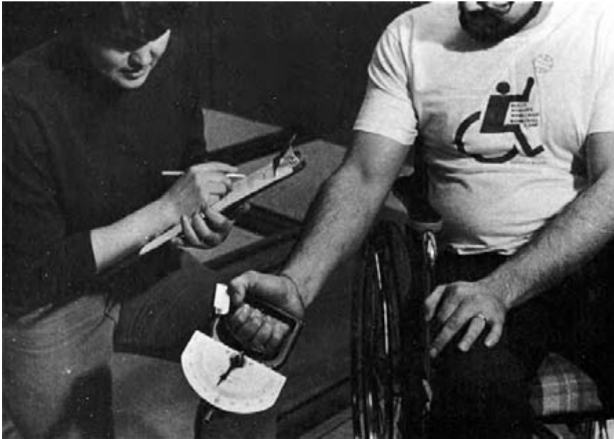
Some devices are specially designed to assess grip strength, such as this hand dynamometer.
