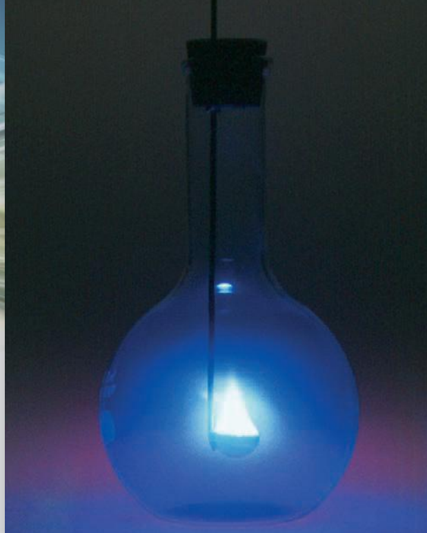
Sulfur burning in oxygen to form sulfur dioxide. About 50 million tons of \text{SO}_2 are released to the atmosphere every year.
