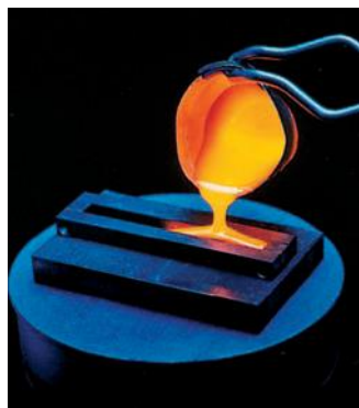
Molten glass is poured over nuclear waste before burial.
