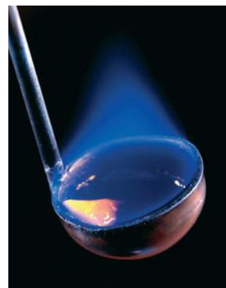
Sulfur burning in air to form \text{SO}_2 .
