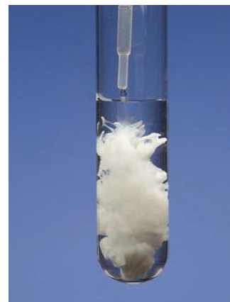
Figure 4.5 Formation of \text{BaSO}_4 precipitate.
