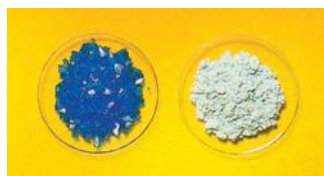
\text{CuSO}_4 \cdot 5\text{H}_2\text{O} (left) is blue; \text{CuSO}_4 (right) is white.
