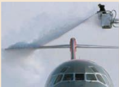
Airplane wings are de-iced with a solution that contains ethylene glycol, which lowers the freezing point, so the ice melts.
