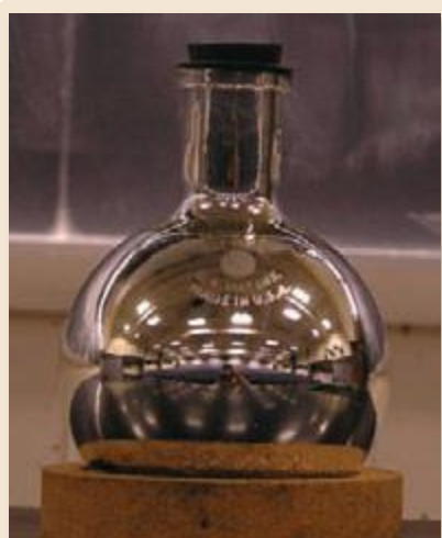
Aldehydes are said to give a positive Tollens test; that is, they react with \text{Ag}^+ to form \text{RCOOH} and \text{Ag} . When the reaction is carried out in a glass flask, a silver mirror is formed on its walls. Other functional groups give a negative Tollens test; that is, no silver mirror forms.
