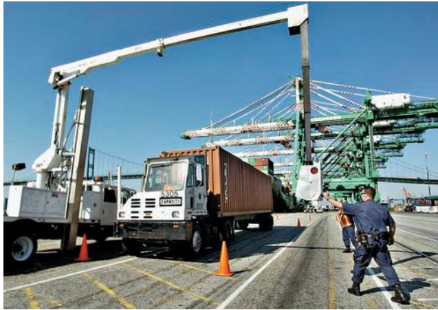
A U.S. Customs officer helps direct the use of a mobile gamma ray scanner to reveal the contents of a steel-shipping container, one of the 20 million closed containers that carry cargo into the United States each year. The device, used to help reveal nuclear, biological, or chemical threats inside, is one of more than 100 gamma and x-ray inspection devices deployed at major ports and border crossings into the United States. (AP/Wide World Photos)
