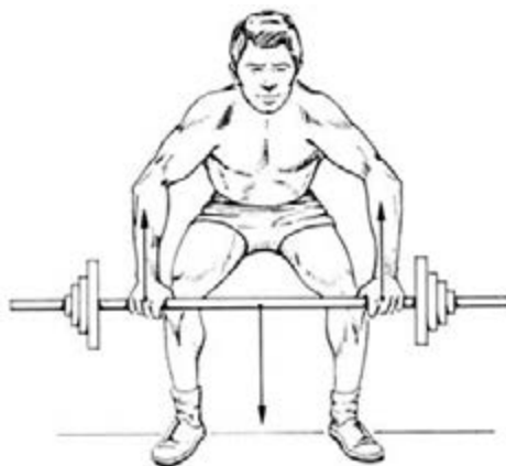
Figure 12.10 Example of parallel forces producing linear motion.
