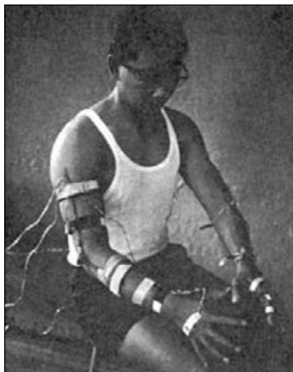
Figure 22.7 Elbow and wrist elgons on right arm; index finger and forearm elgons on left arm. Source: From "An Introduction to Electrogoniometry," Kinesiology Review 1968, by M. J. Adrian. Copyright © 1968, American Association for Health, Physical Education and Recreation, Washington, DC.
