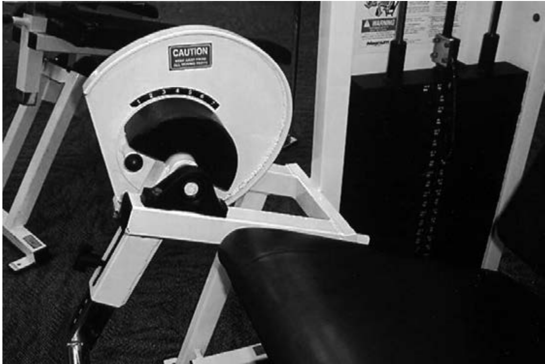
Figure 15.3 A resistance machine with an isotonic cam. The length of the resistance arm changes to vary the resistance as the muscle angle of pull changes.
