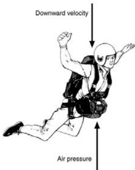
Figure 20.9 The spread-eagle position used to increase air pressure in skydiving.
