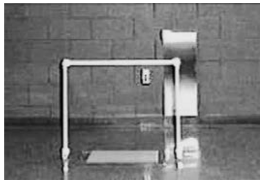
Figure 22.5 A reference frame consists of known distances in the x (horizontal) and y (vertical) directions.
