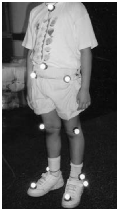
Figure 22.6 Reflective markers are used with a number of optoelectronic data collection systems.
