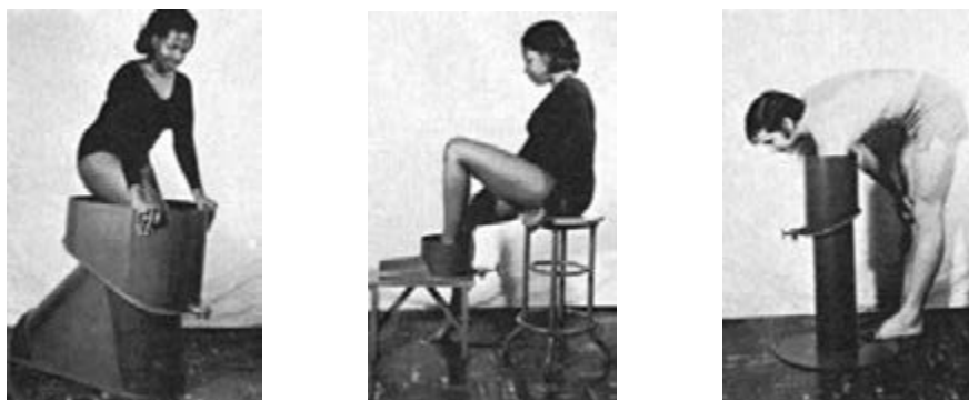
Figure 14.19 Immersion tanks for determination of segmental weights. Using segment landmarks as defined by Dempster, the segment is immersed in water. The displaced water is weighed and multiplied by the specific gravity of the segment to obtain the segmental weight. Source: From Scientific Bases of Human Movement (3rd ed.), by B. Gowitzke & M. Milner. Copyright © 1988, Williams & Wilkins, Baltimore, MD.
