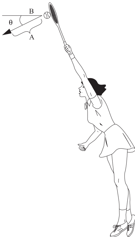
Figure 12.2 Graphic representation of a force vector. The magnitude of the force is the vector line, A; the point of application is the beginning of the vector, B; and the direction of the vector is represented by the arrowhead and the angle \theta .
