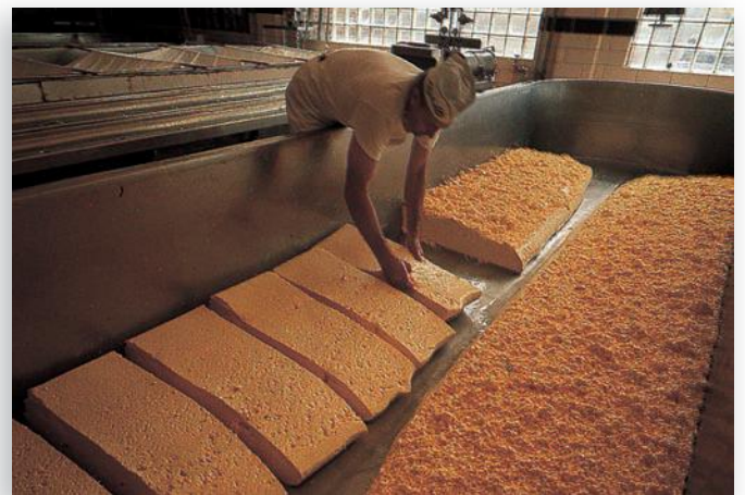
Figure 25.10 Cheese making. The curd-cutting stage in the making of cheddar cheese.
