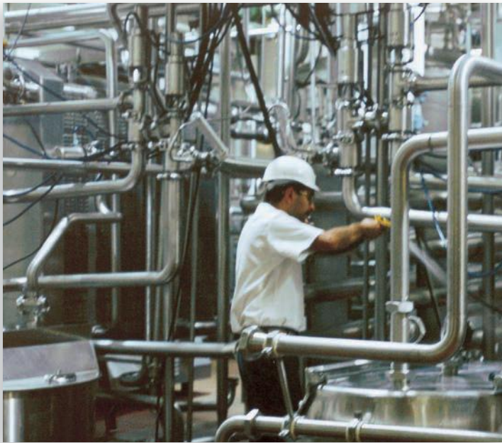
Figure 25.13 A modern flash pasteurizer, a system used in dairies for high-temperature short-time (HTST) pasteurization.
