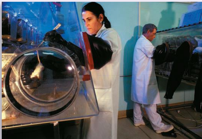
Sterile enclosure for rearing and handling germ-free laboratory animals.
