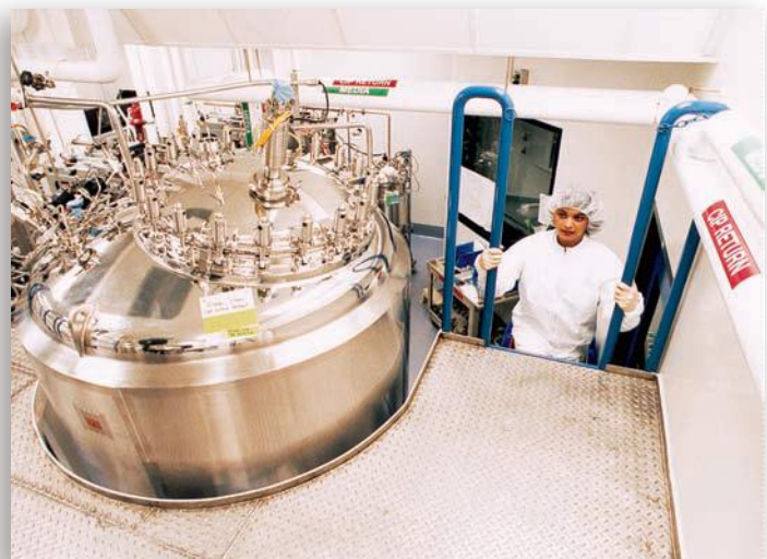
Figure 25.17 A cell culture vessel used to mass-produce pharmaceuticals. Such elaborate systems require the highest levels of sterility and clean techniques.
