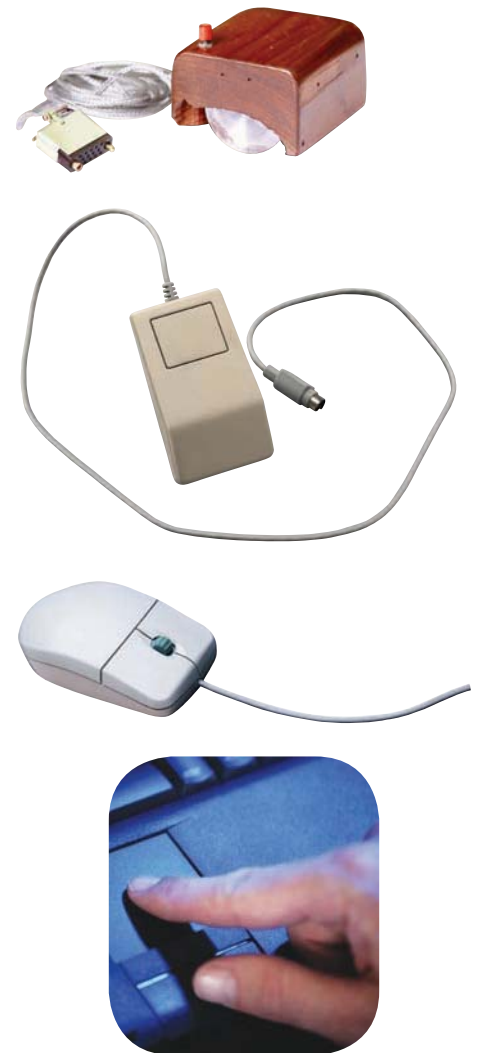
FIGURE 55.1 Building a Better Mouse The figure shows the evolution of the computer mouse from its wooden-box beginnings ( top ) to its later, sleeker forms ( middle photos ). The evolution has continued with the development of the touchpad or trackpad ( bottom )—a built-in mouse substitute in laptop computers. The mouse and the touchpad are tools that many of us take for granted, but they are the product of design decisions that have improved their utility and efficiency.
