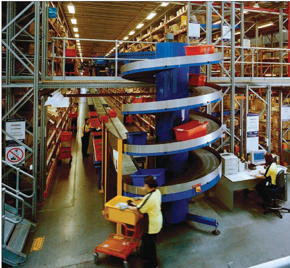
POST LOGISTICS IN AUSTRALIA DISTRIBUTES THE SPEEDO SWIMWEAR BRAND. THREE LEVELS OF STORAGE ARE CONNECTED BY A SPIRAL CONVEYOR LINKED TO A "SMART" HORIZONTAL CONVEYOR SYSTEM THAT INTERCONNECTS PICKING ZONES ON EACH OF THE THREE LEVELS AND CARRIES THROUGH TO A SIX-LANE PACKING AND DISTRIBUTION AREA.
