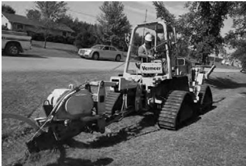
Fig. 2.47 A cable plowing machine that is used in a nonurban environment. (Photo courtesy of © VERMEER CORPORATION. All Rights Reserved; www.vermeer.com .)
