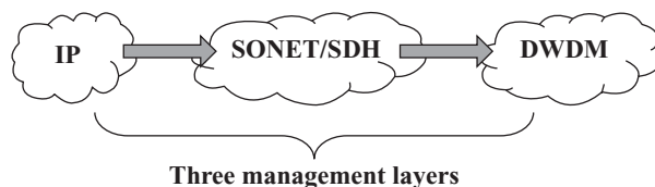
Fig. 13.49 Concept of an IP-over-SONET-over-DWDM architecture
