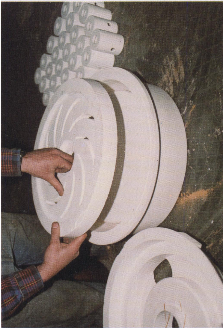
Fig. 3.47 Complete ceramic shell mold for producing stainless steel pump impellers, volutes, and diffusers for the chemical, food, petroleum, and other associated industries. Photo shows core being inserted into drag half prior to closure. Cast accuracy and surface finish matches investment casting at a fraction of the cost. Smooth cast surface vastly improves a pump operating efficiency over castings produced in sand molds
