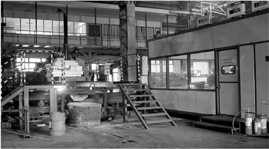
Fig. 9.4 Automatic Pouring System installed by M/S Inductotherm at the Automotive Castings Foundry of M/S Mahindra Hinoday Industries, Pune. (By courtesy of M/S Inductotherm (india) Pvt. Ltd., Ahmedabad)
