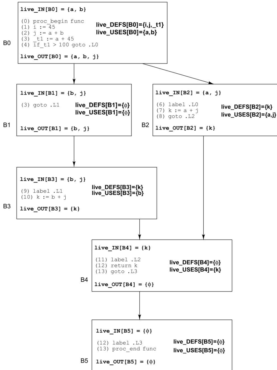
Fig. 7.45 Flow graph annotated with live variable analysis information
