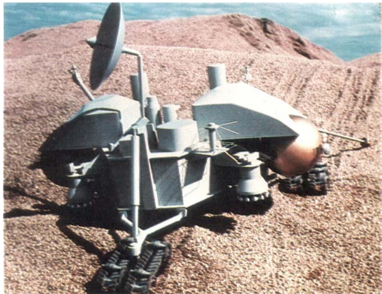
Two prototypes of future Mars rovers: a smart obstacle-avoiding machine, constructed at the Rensselaer Polytechnic Institute, and a Viking Lander mounted on tractor treads. The actual Mars rovers of the future are likely to include elements of both designs.
