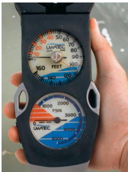
A scuba diver's pressure gauge shows the amount of air (usually measured in psi) in his tank before and during a dive.
