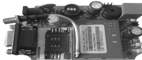
Fig9:SIM300 with Antenna Connector used:
