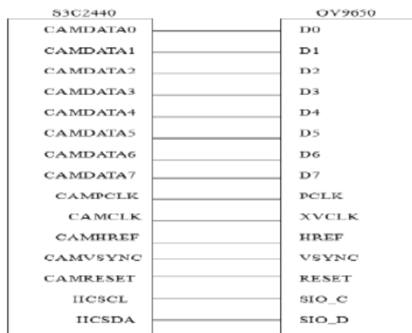
Fig5: The interconnection of S3C2440 and OV9650
