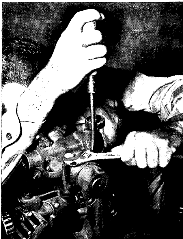
Figure 61. Loosening worm clamping bolt of elbow telescope.
