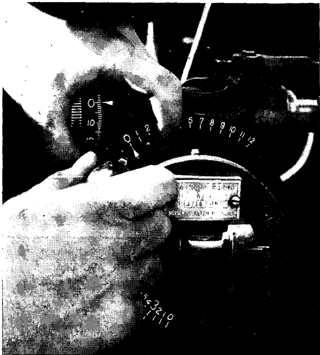
Figure 58. Shifting elevation scale index to zero.
