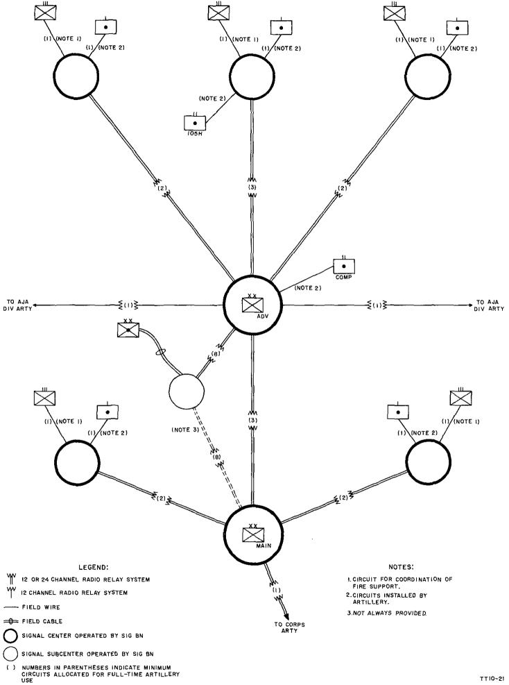
Figure 4. Type artillery sole-user circuits provided by division area communication system.
