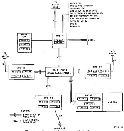
Figure 21. Forward signal center, block diagram.
