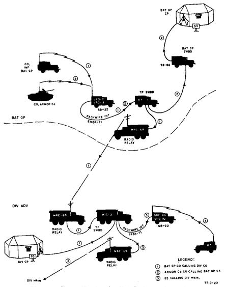
Figure 10. Type utilization of radio/wire integration system.
