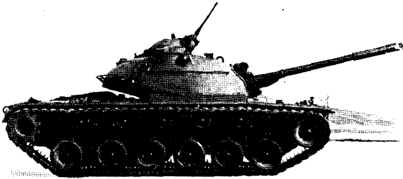
Figure 5. The M48, a medium-gun tank. Main armament is a 90-mm gun. A caliber .30 machinegun is coaxially mounted with the main gun, and a caliber .50 machinegun is mounted in the cupola.
