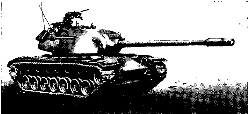
Figure 6. The M103, a heavy-gun tank. Main armament is a 120-mm gun. A caliber .30 machinegun is coaxially mounted with the main gun, and a caliber .50 machinegun is mounted on the turret.
