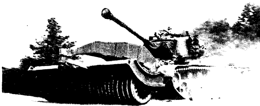
Figure 18. High Herman. A tank-mounted mine clearance device. Weighs 36 tons and detonates mines by pressure. (A development item.)
