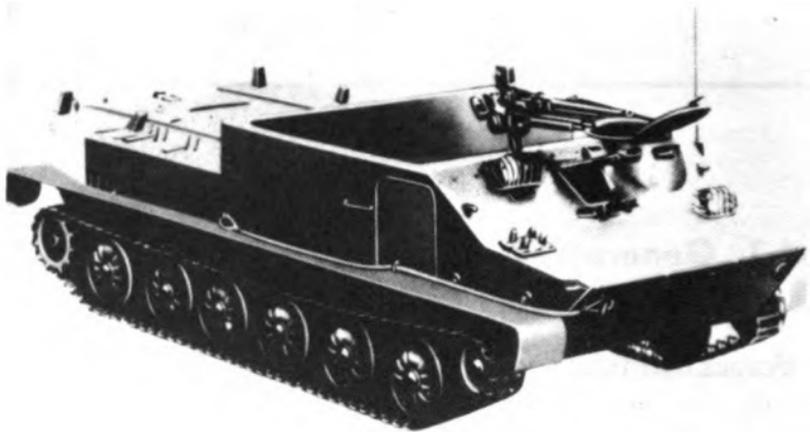
*Figure 6-1. BTR-50P series tracked APCs. The original BTR-50P (above) has an open top. The newer BTR-50PK (below), with overhead armor covering, is in more general use. Most tank divisions use tracked APCs, either the newer BMP or BTR-50P types.*
