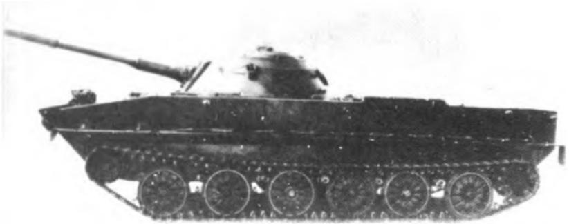
*Figure 6-18. PT-76 light amphibious tank.* With its light armor and 76-mm gun, the PT-76 is better equipped for reconnaissance missions than for armored battles. Note the rectangular shaped chassis with sloping bow, the low-profile turret, and the fold-up bow flap for amphibious swimming.
