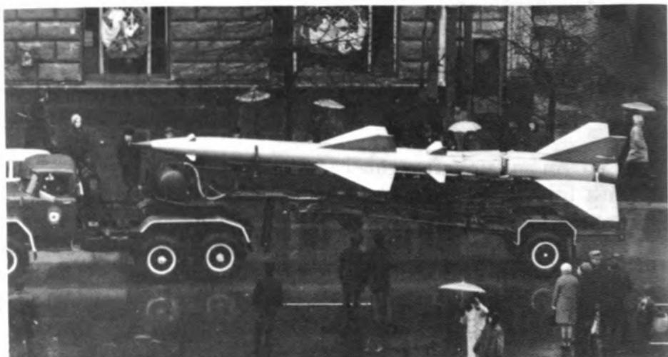
**Figure 6-40. SA-2 GUIDELINE.** A medium-range surface-to-air missile transported on a truck-towed trailer/launcher. The main SAM system in the Soviet Air Defense Forces (PVO Strany), GUIDELINE is also deployed with Soviet Ground Forces in Europe and has been exported to satellite nations.
