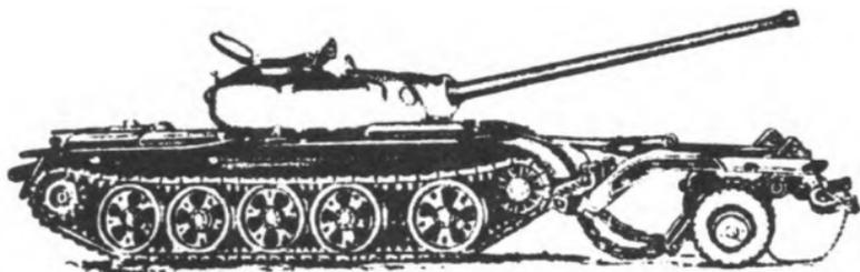
*Figure 6-53. Mine clearing equipment.* Mine clearing devices can be fitted to tanks or wheeled vehicles. Mine rollers (above) or plows (below) are used to clear pathways through minefields.
