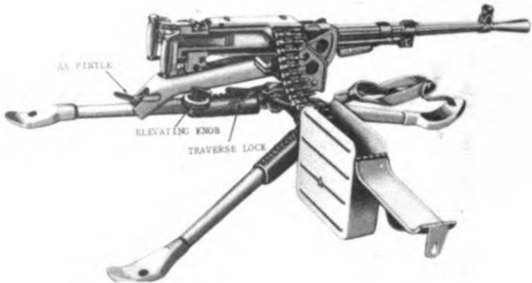
*Figure 6-8. 7.62-mm heavy machinegun SGM.* Mounted on many APCs, this weapon is belt-fed and has an effective range of about 1,000 m.
