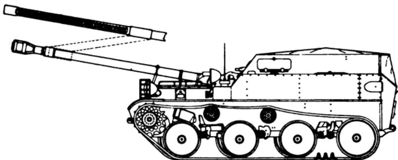
*Figure 6-19. Self-propelled assault guns. Two types of light SP assault guns are employed by Soviet airborne troops. The ASU-57 (above), with a 57-mm anti-tank gun, has only light armored protection and an uncovered crew's compartment. Note the four large roadwheels. The newer 85-mm ASU-85 (below) is fully armored.*
