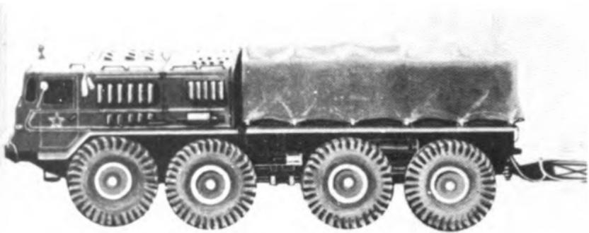
**Figure 6-73. Heavy trucks. The 7.5-ton KrAZ-255B (above) is often used to carry bridge spans for the PMP folding bridge. The MAZ-535 (below) tows a launcher/trailer for surface-to-air missiles.**
