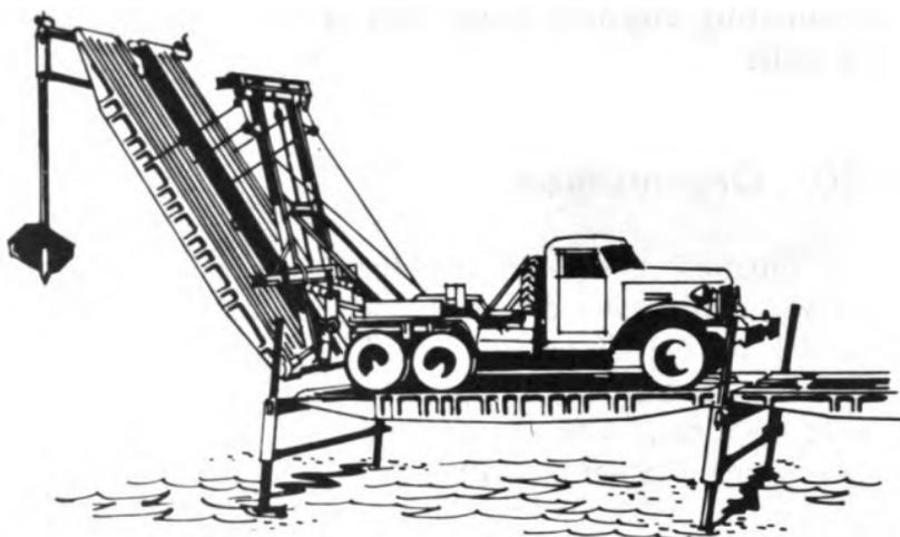
**Figure 6-48. Truck-launched bridges.** Soviet truck-launched bridges are noted for their multi-span capacity. The KMM (above) and TMM scissors-type (below) bridges are launched from the rear of trucks, each truck backing out over the already laid spans.
