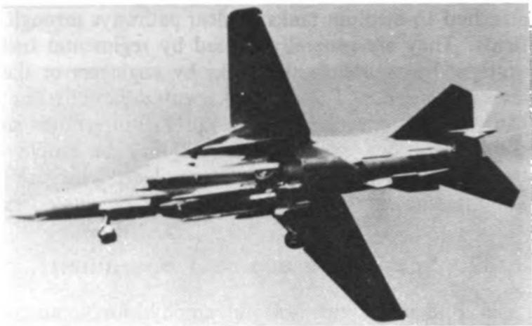
*Figure 6-55. Tactical air support.* The MiG-23 FLOGGER (above), a variable geometry wing fighter-bomber, is an effective short take-off and landing (STOL) aircraft. The Mig-25 FOXBAT (below) is an all-weather, high-altitude interceptor, easily recognized by its rectangular air intakes on either side of the fuselage.
