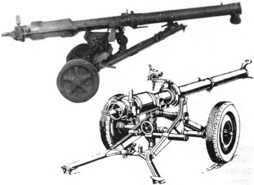
*Figure 6-35. Recoilless anti-tank guns. Older weapons, such as the 82-mm B-10 (above, left) and the 107-mm B-11 (above, right), are now being replaced by the new 73-mm SPG-9 (below), which fires a rocket assisted projectile at ranges of about 1,000 meters.*
