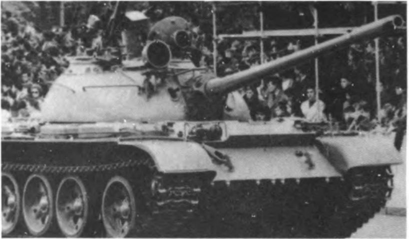
**Figure 6-16. T-54/55 medium tanks. T-54 and T-55 tanks exist in numerous variations, all of which mount a 100-mm main gun and can be easily recognized by the large gap between the first and second roadwheels. The T-54A (above) mounts an AA machinegun in addition to coaxial and bow machineguns. The T-55 (below) lacks the AA machinegun.**
