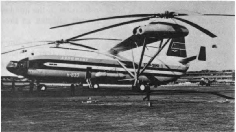
*Figure 6-56. Mi-12 HOMER.* HOMER is the largest helicopter in the world. It is easily recognized by the two large wing-tip rotors, and is shown here in use by AEROFLOT, the Soviet civilian airline.
