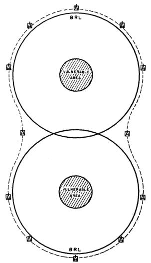
Figure 16. Modified oval, optimum gun ring.
