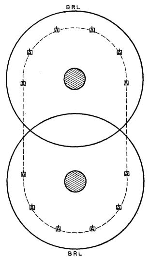
Figure 15. Multiple vulnerable areas—oval (race track), optimum gun ring.
