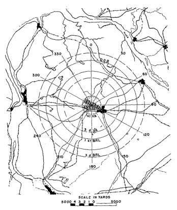
Figure 23. Third vulnerable area and bomb release line.
