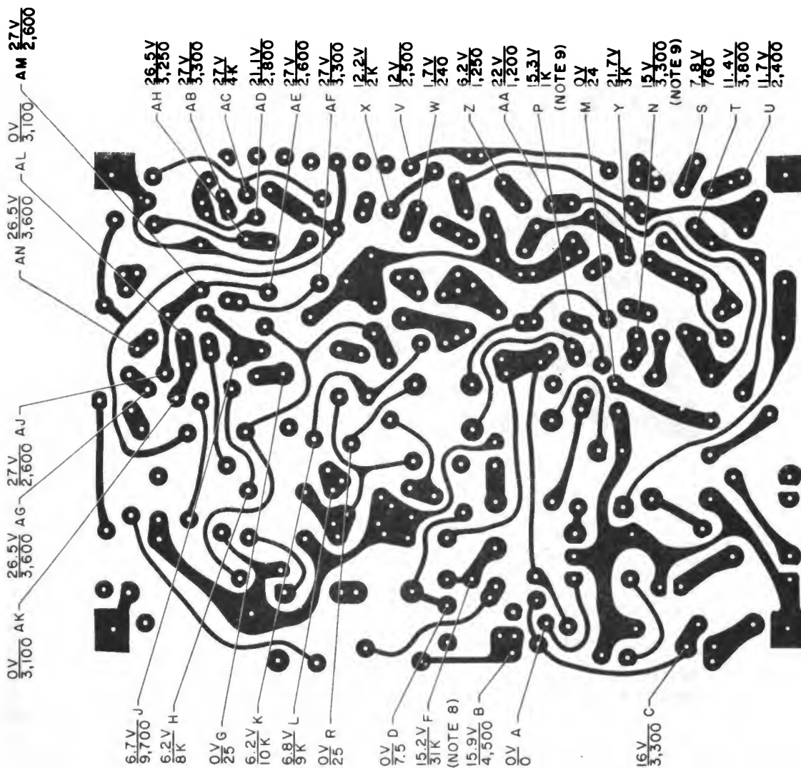
Figure 9. Voltage and resistance measurements and test point location diagram, R-1041A/ARN.
