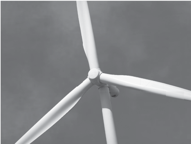
(a) Wind Turbine: An Open, Unshrouded, Incompressible, Axial Turbomachine
