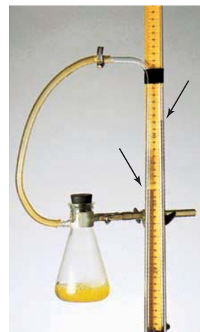
Figure 14.7 The rate of hydrogen peroxide decomposition can be measured with a manometer, which shows the increase in the oxygen gas pressure with time. The arrows show the mercury levels in the U tube.
