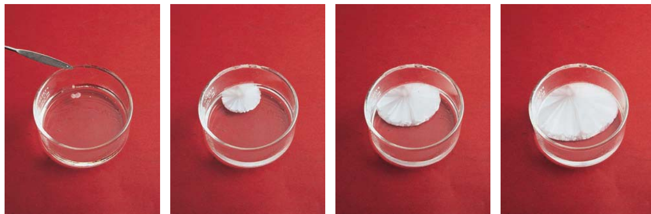
Figure 9.4 Sodium acetate crystals rapidly form in a supersaturated solution when a small seed crystal is added (left).
