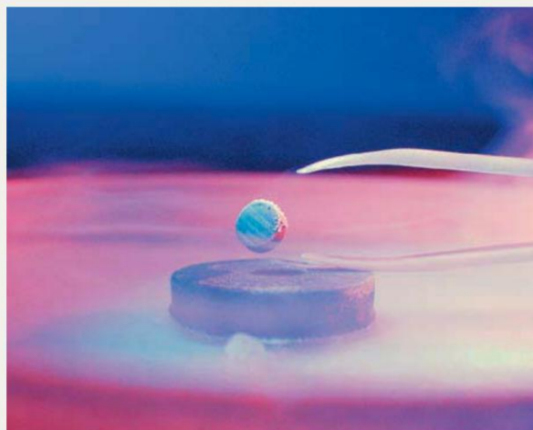
The levitation of a magnet above high-temperature superconductor immersed in liquid nitrogen
