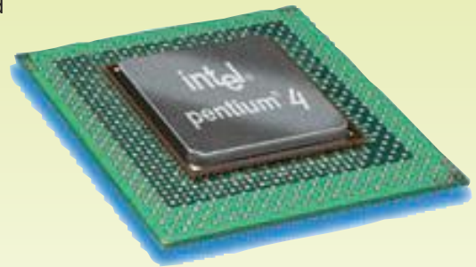
(above) Pentium 4 microprocessor chip mounted in protective frame with pins that can be connected to an electronic device such as a microcomputer.
