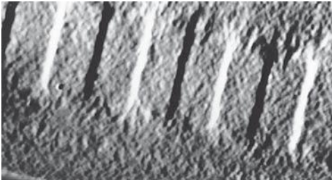
Bits on disk. Magnetic bits on a disk surface, caught by a magnetic force microscope. The dark stripes are 0 bits; the bright stripes are 1 bits.
