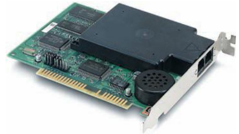
Fax modem circuit board, which plugs into an expansion slot inside the computer
