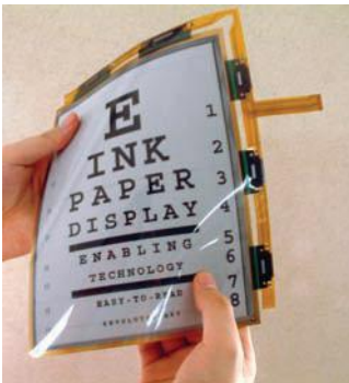
E Ink’s flexible screen on 0.3-millimeter thick electronic “paper” with millions of tiny capsules with black and white pigment chips and transmitting electrodes.
