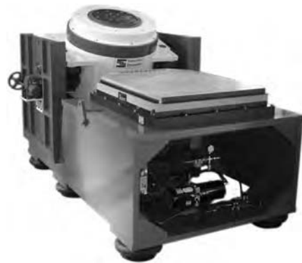
FIGURE 4.3 Photograph of slip table (Courtesy of Saraswati Dynamics Private Ltd., India)
