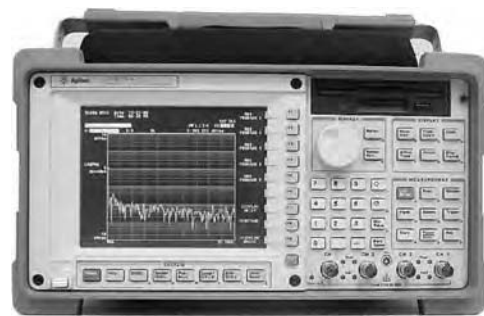
FIGURE 8.11 FFT analyser (Courtesy of http://www.home.agilent.com )
