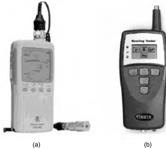
FIGURE 8.5 Instruments for measuring vibration: (a) portable vibration meter (Courtesy of http://www.rion.co.jp ), (b) shock pulse meter (Courtesy of http://www.bdi-usa.com )
