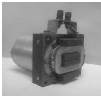
FIGURE 4.13 Electromagnetic exciter: (a) schematic, (b) photograph (Courtesy of IIT Madras)
