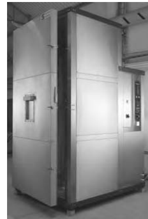
FIGURE 4.4 Climatic chamber (Courtesy of Saraswati Dynamics Private Ltd., India)
