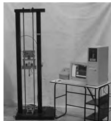
FIGURE 4.20 Drop shock machine (Courtesy of http://www.mpmtechnologies.com )
