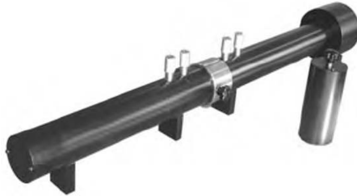
FIGURE 13.16 Photograph of impedance tube (Courtesy of http://www.bswa-tech.com )
