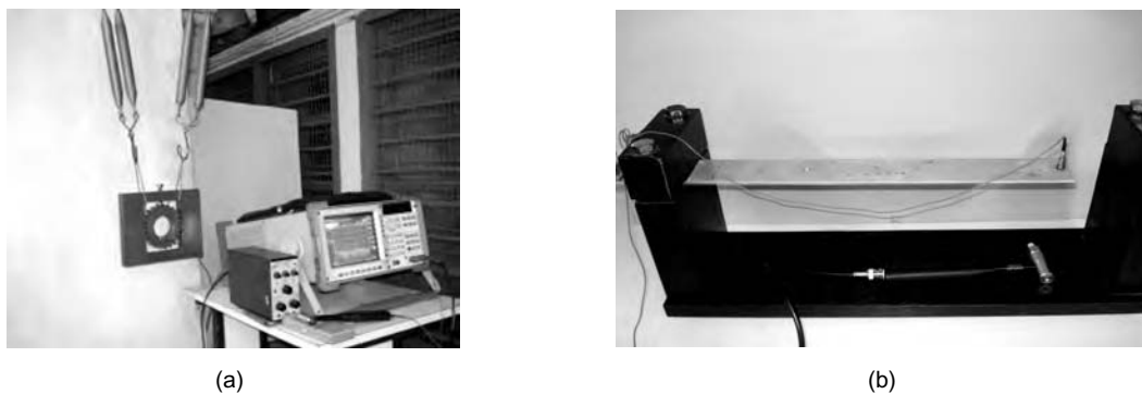
FIGURE 10.1 Boundary conditions in modal testing: (a) free, (b) fixed
