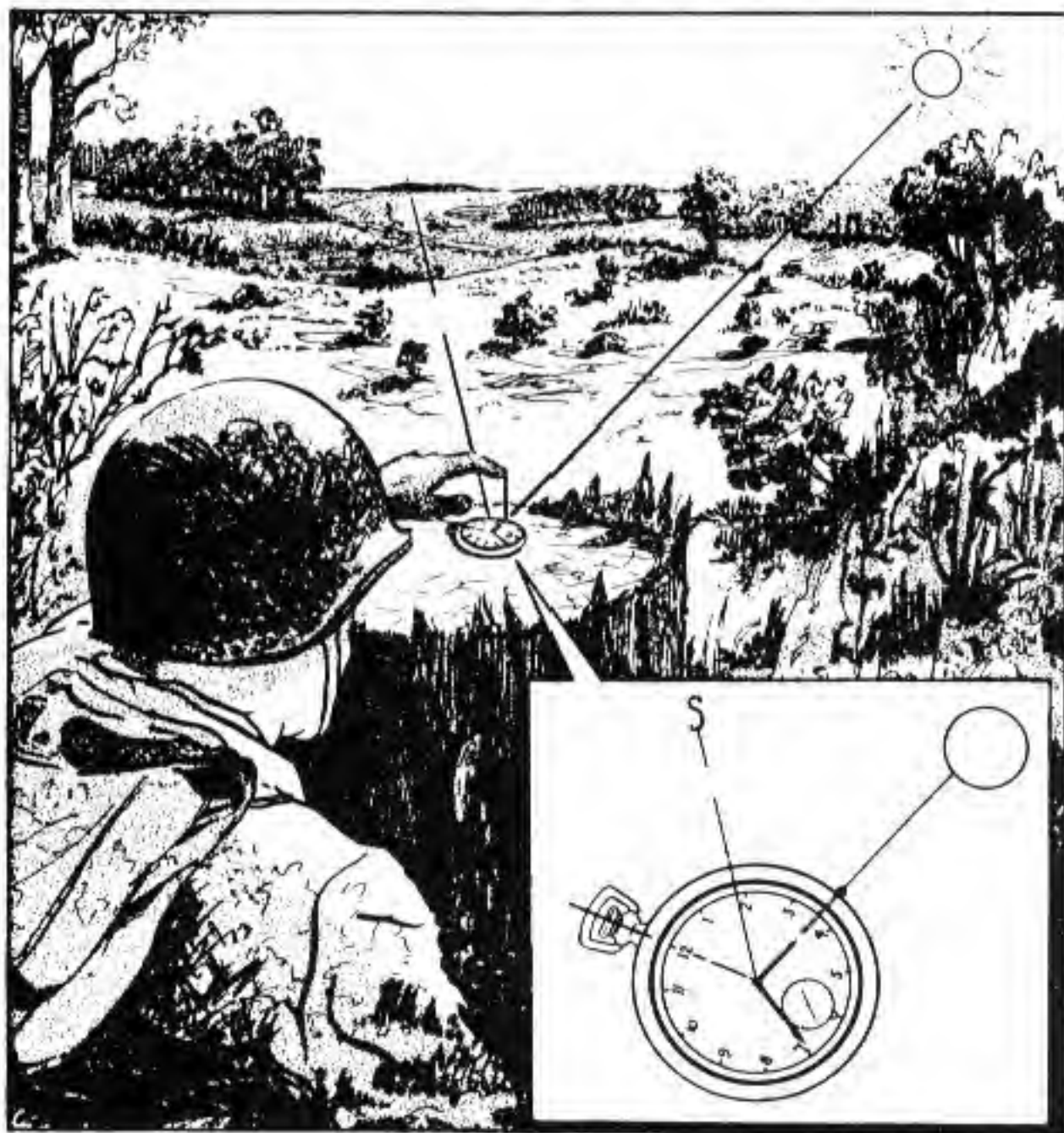
Figure 9. Sun and watch method of determining direction.
