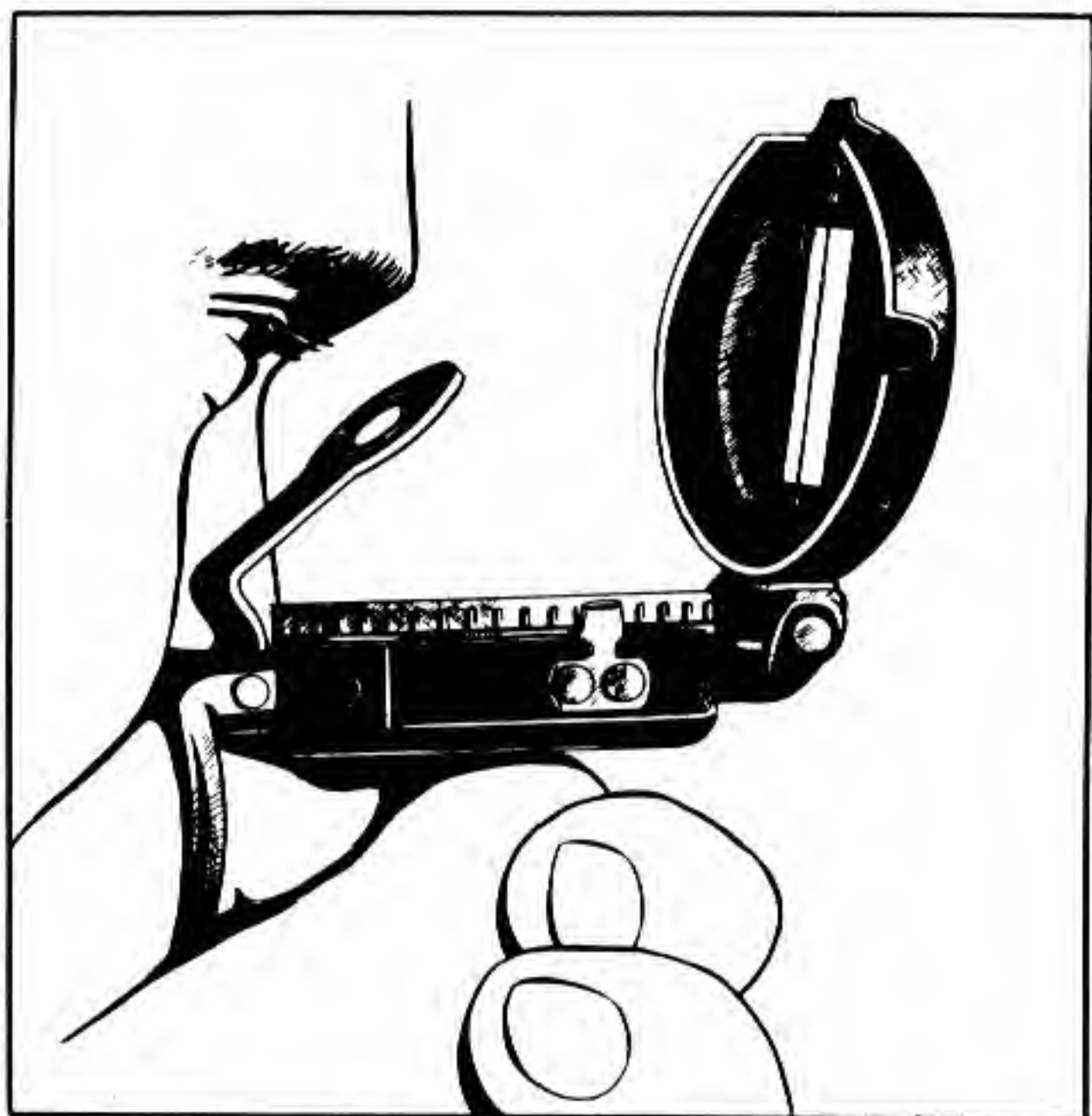
Figure 35. A method of holding the compass.
