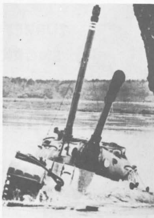
NOTE: Periscope on top of snorkel.
