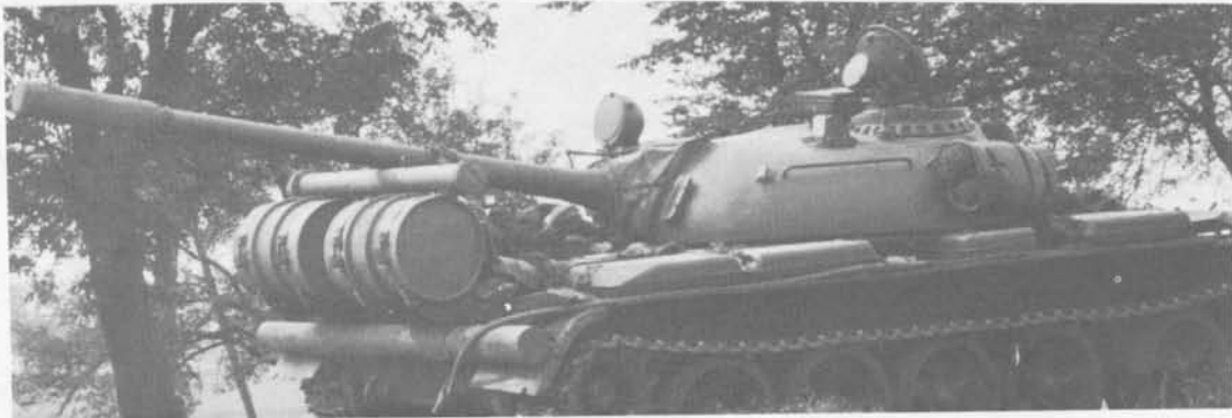
T-55 NOTE STOWAGE OF COMBAT SNORKEL AND DEDITCHING LOG
