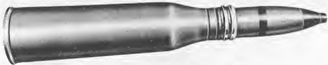
SOVIET 57-mm MODEL UOR-281 FRAG-T CARTRIDGE
