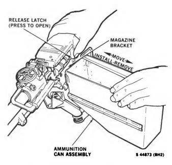
Figure 4-10. Installation and Removal of Ammunition Can on Machinegun M60D
