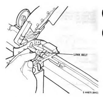
Figure 4-11. Positioning Cartridge Link Belt on Machinegun M60D
