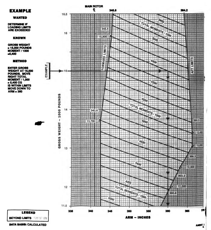
Figure 6-2. Center of Gravity Limits Chart (Sheet 1 of 2)
