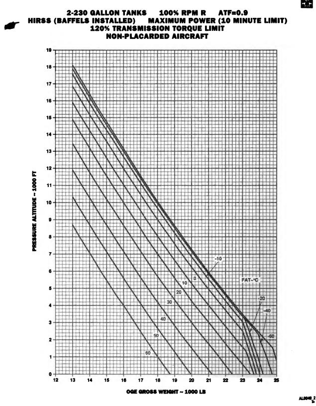
Figure 7.1-6.1.2. Maximum Gross Weight to Hover OGE - High Drag (Sheet 2 of 2)
