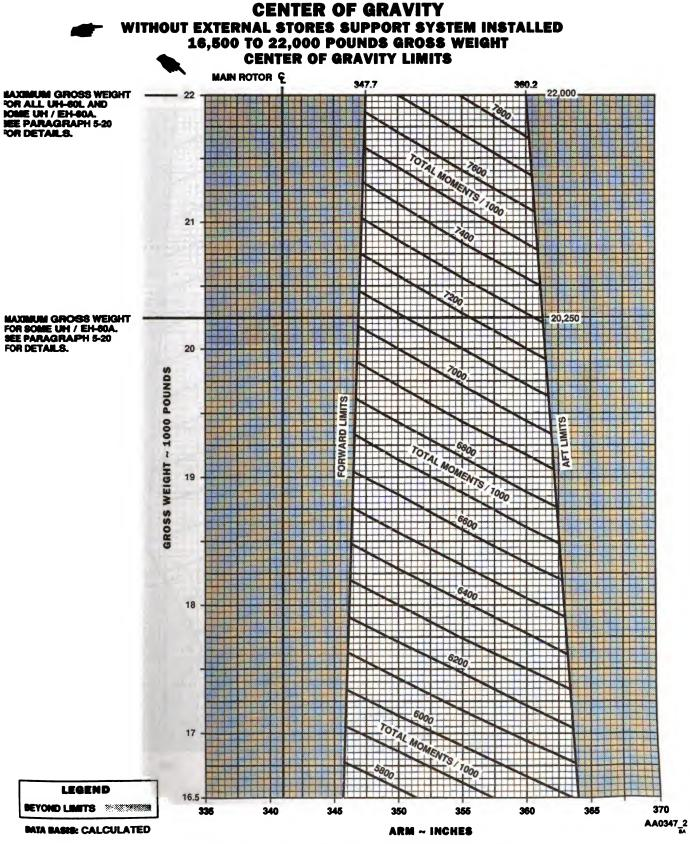
Figure 6-2. Center of Gravity Limits Chart (Sheet 2 of 2)
