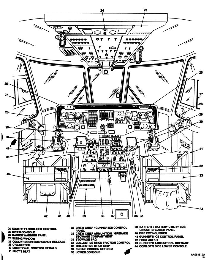
Figure 2-4. Cockpit Diagram (Sheet 2 of 2)
