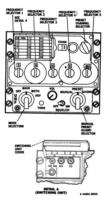
Figure 3-6. UHF Control, AN/ARC-164(V)
