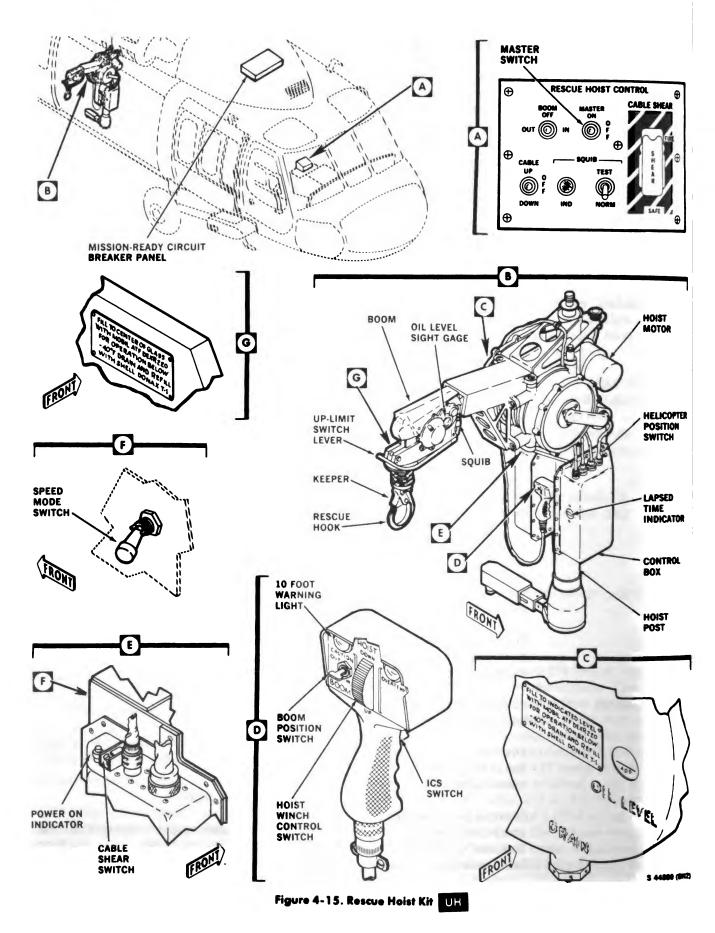
head is allowed to swivel 65° above the boom cable and 30° from side-to-side and guide the cable to wrap or unwrap from a 30° cone angle. The upper limits of cable control includes an automatic means for decelerating the cable to 67 feet-per-minute cable speed. At 8 to 10 feet below the boom head, a caution light on the crewman's control pendant marked CAUTION will go on. The cable will again decrease speed to 12 feet-perminute at 12 to 18 inches below the boom head.
