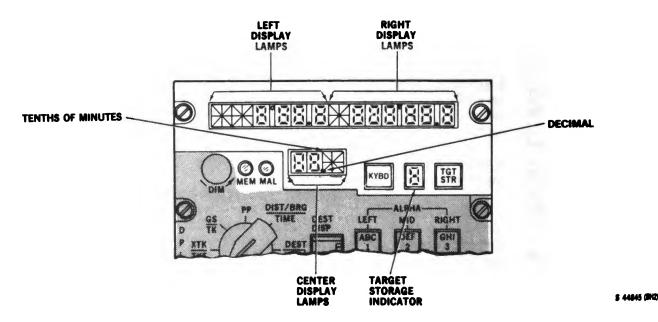
Figure 3-12. Doppler Lamp Test Mode Display
