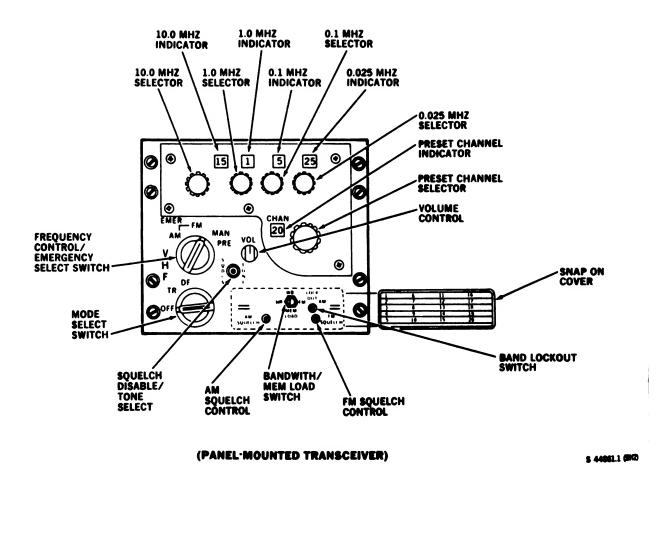
Figure 3-5. VHF Control AN/ARC-186(V) (Sheet 1 of 2)
