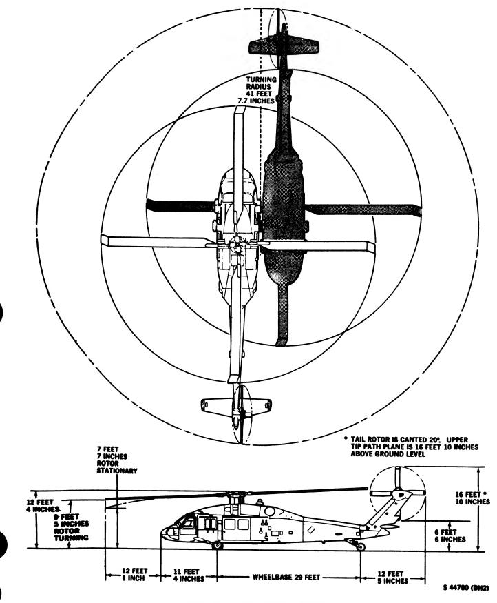
Figure 2-3. Turning Radius and Clearance
