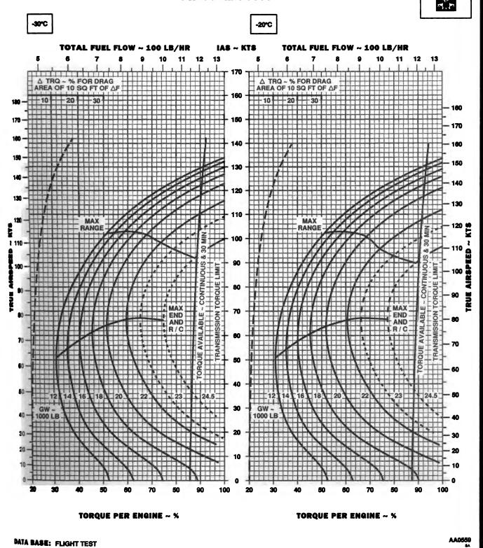
Figure 7-21. Cruise High Drag - Pressure Altitude 8,000 Feet (Sheet 2 of 6)
