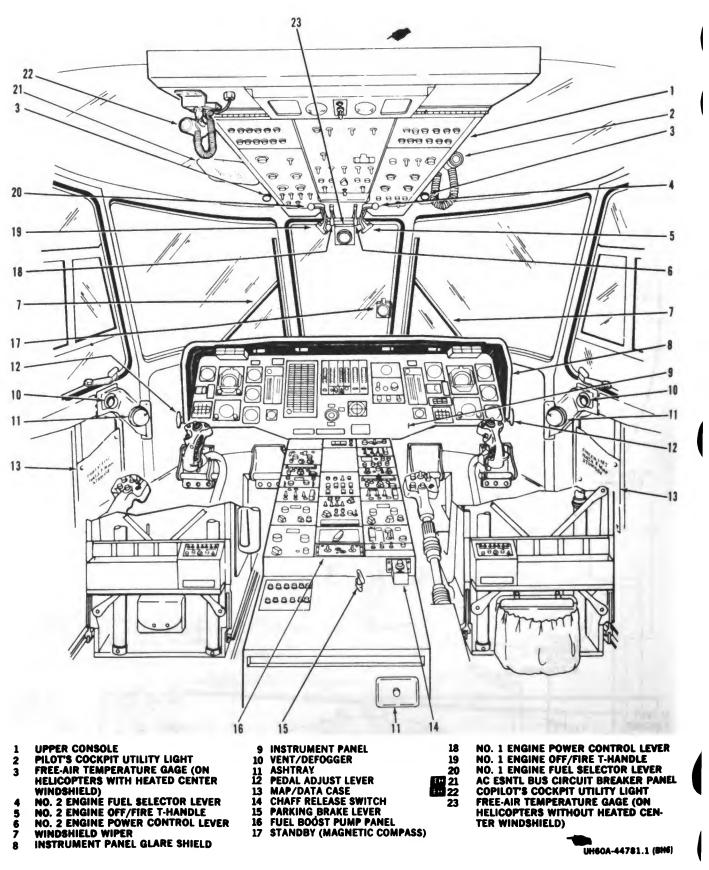
Figure 2-4. Cockpit Diagram (Sheet 1 of 2)
