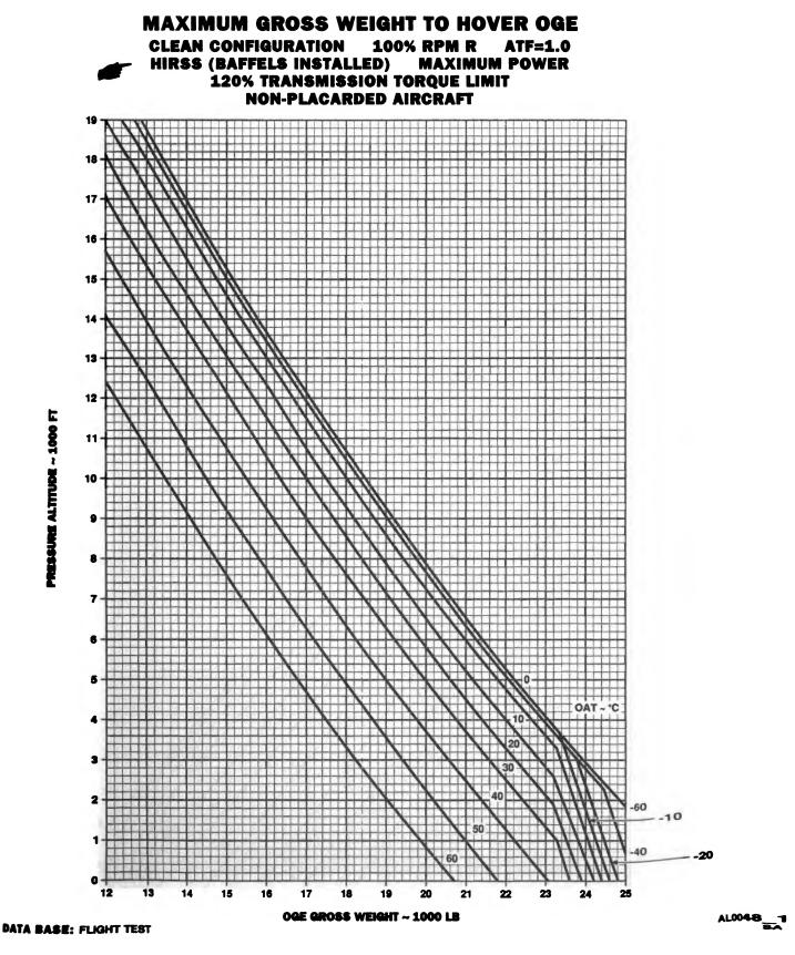
Figure 7.1-6.1.1. Maximum Gross Weight to Hover OGE (Sheet 1 of 2)
