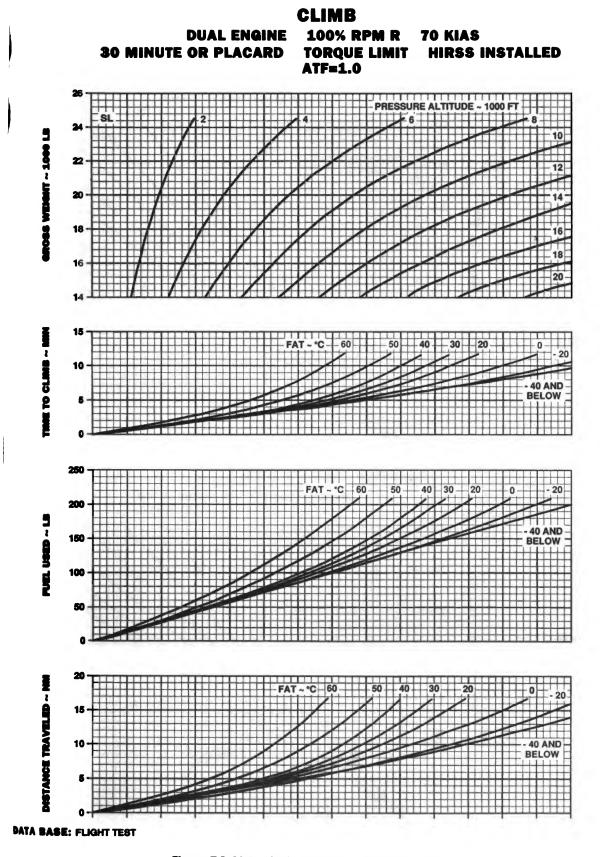
Figure 7.1-22.1. Climb - 2 Engine, ATF=1.0 - High Drag
