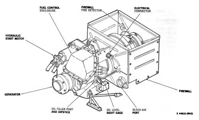
Figure 2-21. Auxiliary Power Unit (APU) (Typical)
