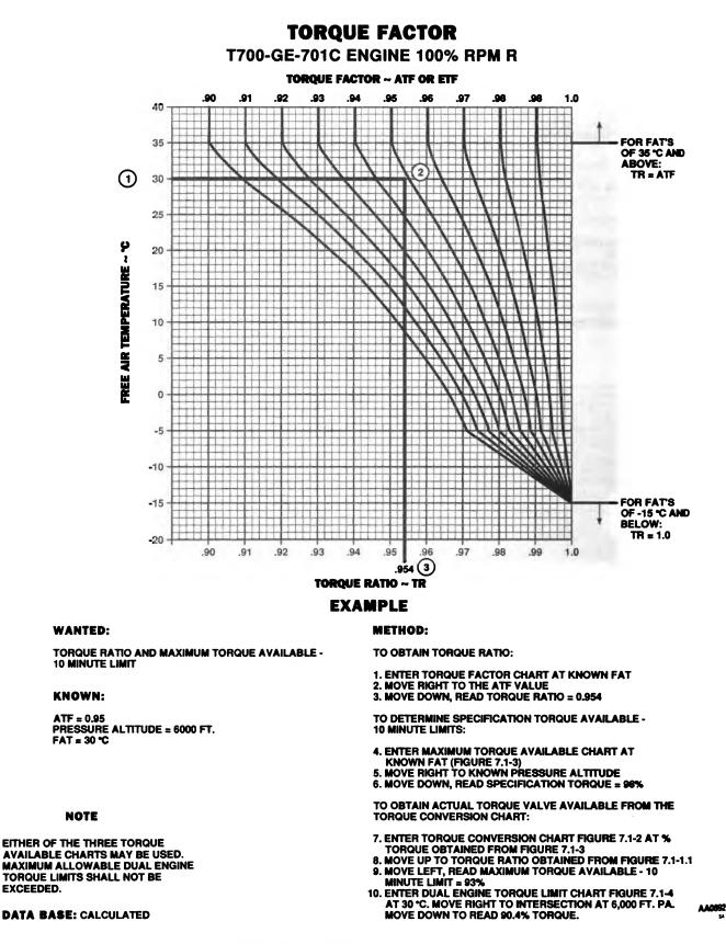
Figure 7.1-1.1. Aircraft Torque Factor (ATF)
