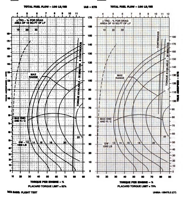
Figure 7.1-16. Cruise - Pressure Altitude 14,000 Feet (Sheet 2 of 5)
