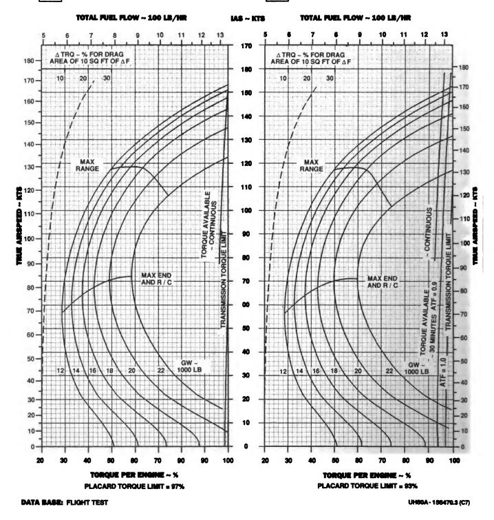
Figure 7.1-13. Cruise - Pressure Altitude 8,000 Feet (Sheet 3 of 6)
