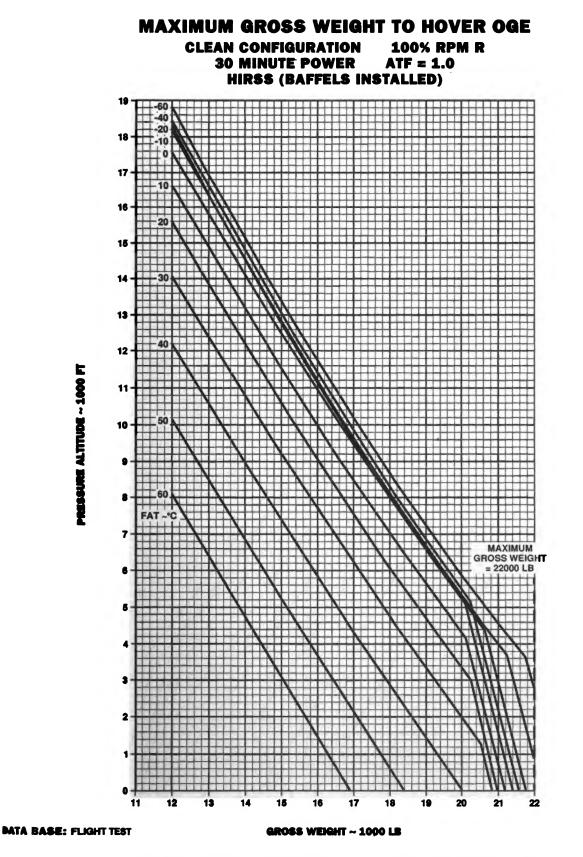
Figure 7-6. Maximum Gross Weight to Hover OGE - Clean (Sheet 1 of 2)
