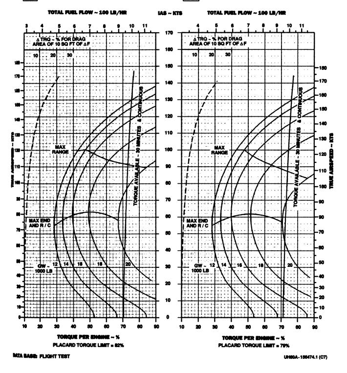
Figure 7.1-17. Cruise - Pressure Altitude 16,000 Feet (Sheet 1 of 4)
