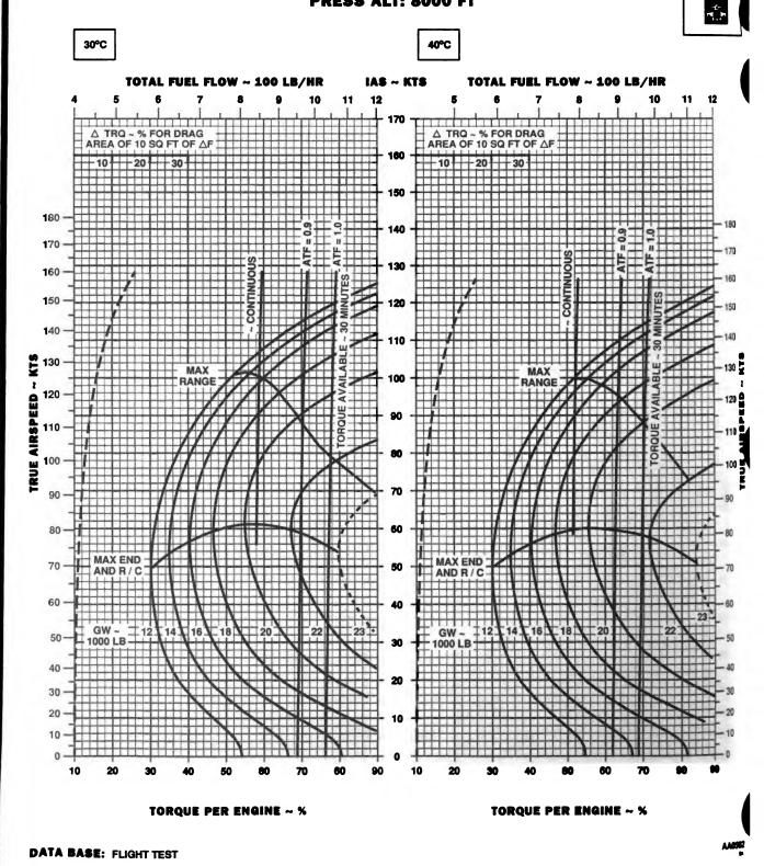
Figure 7-21. Cruise High Drag - Pressure Altitude 8,000 Feet (Sheet 5 of 6)
