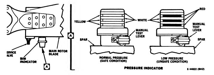
Figure 2-14. Main Rotor Blade and BIM System
