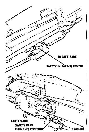
Figure 4-7. Location and Identification of Safety on Machinegun M60D
