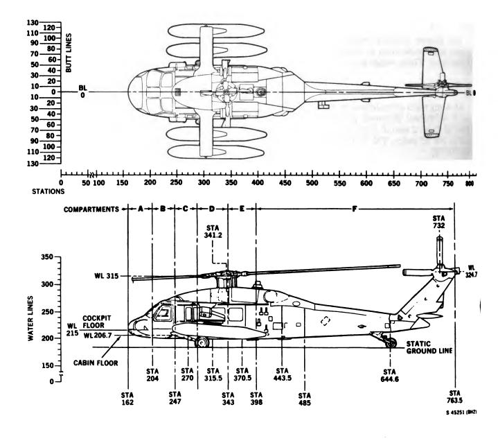
Figure 6-1. Helicopter Compartment and Station Diagram
