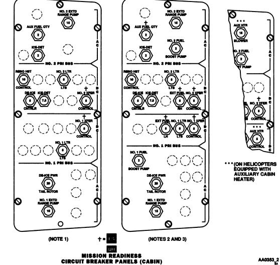
Figure 2-19. DC and AC Circuit Breaker Panels (Typical) (Sheet 2 of 4)
