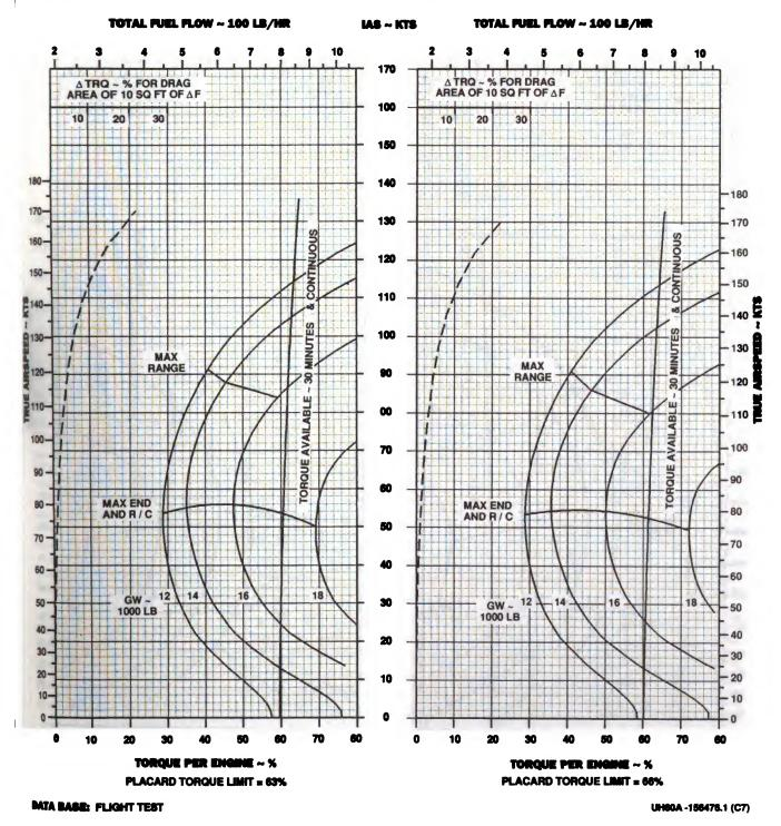
Figure 7.1-19. Cruise - Pressure Altitude 20,000 Feet (Sheet 1 of 4)
