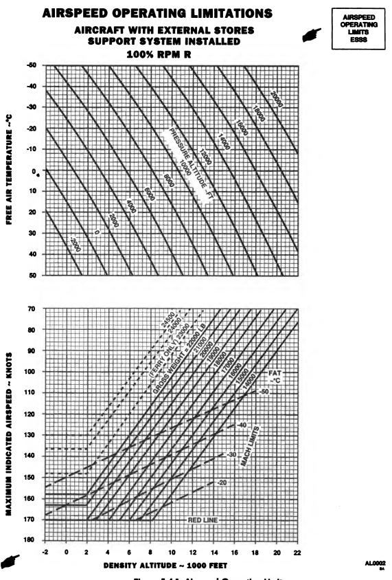
Figure 5-4.1. Airspeed Operating Limits
