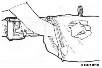
Figure 4-12. Charging (Cocking) Machinegun M60D
