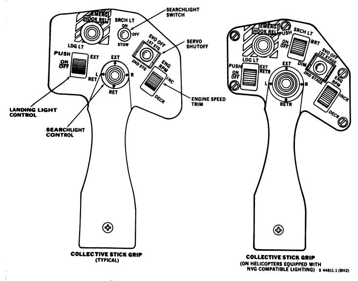
Figure 2-11. Collective and Cyclic Grips (Sheet 1 of 2)
