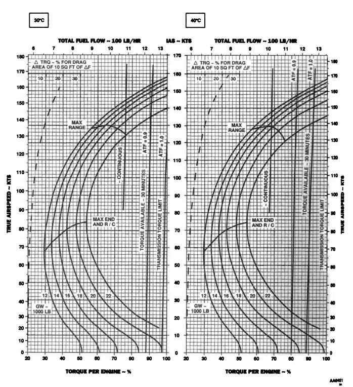
Figure 7-14. Cruise - Pressure Altitude 2,000 Feet (Sheet 5 of 6)
