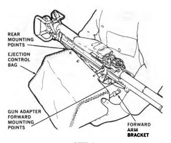
STEP 1 POSITION EJECTION CONTROL BAG ON MOUNTING POINTS
