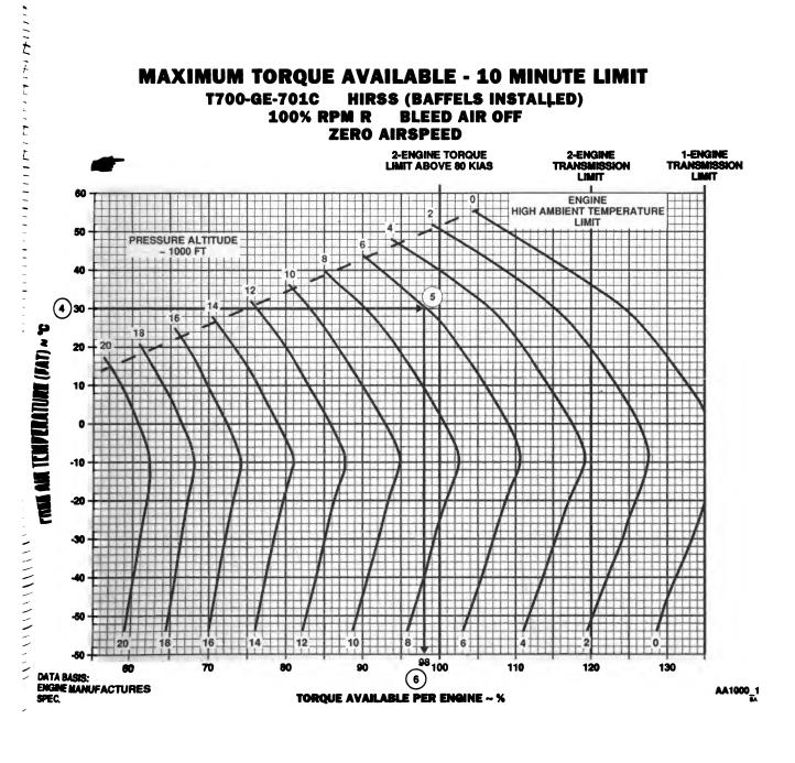
Figure 7.1-3. Maximum Torque Available (Sheet 1 of 3)
