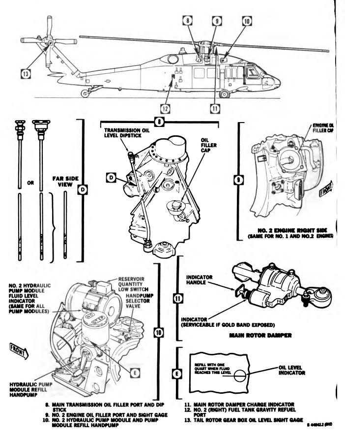
Figure 2-26. Servicing Diagram (Sheet 2 of 3)
