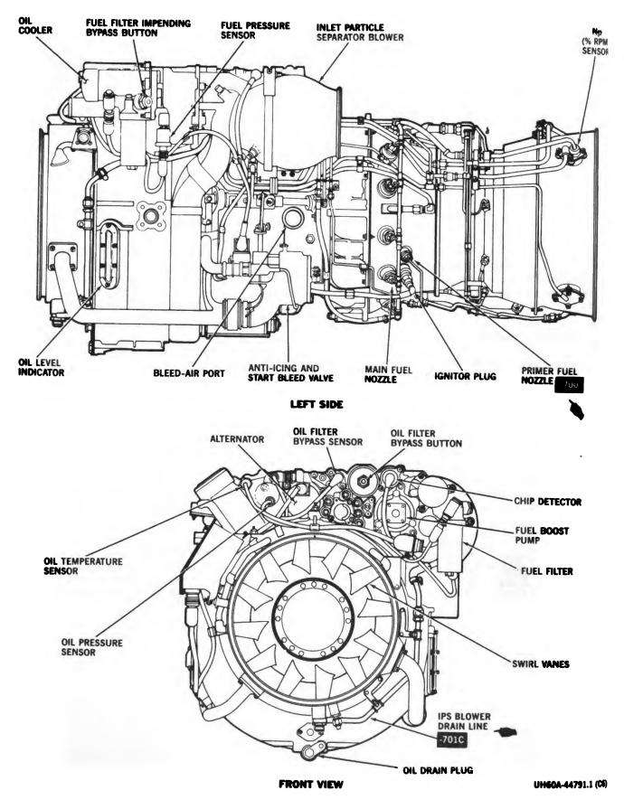
Figure 2-9. Engine T700 (Sheet 1 of 2)
