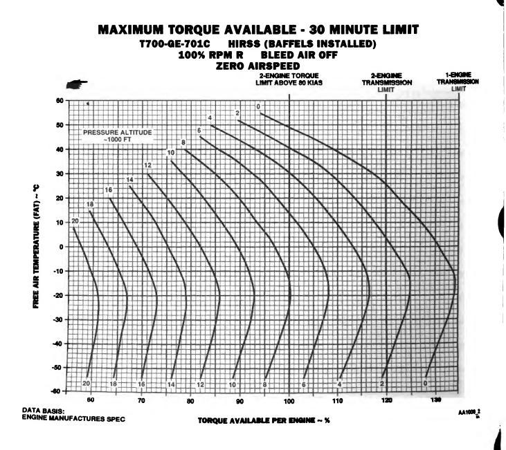
Figure 7.1-3. Maximum Torque Available (Sheet 2 of 3)
