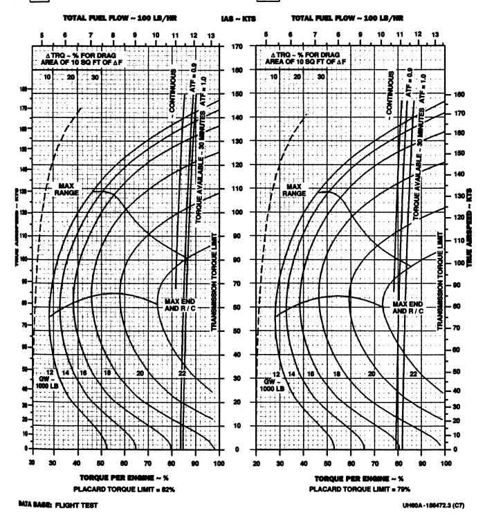
Figure 7.1-15. Cruise - Pressure Altitude 12,000 Feet (Sheet 3 of 5)
