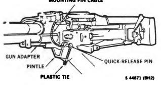
Figure 4-8. Installation of Machinegun M60D on Pintle
