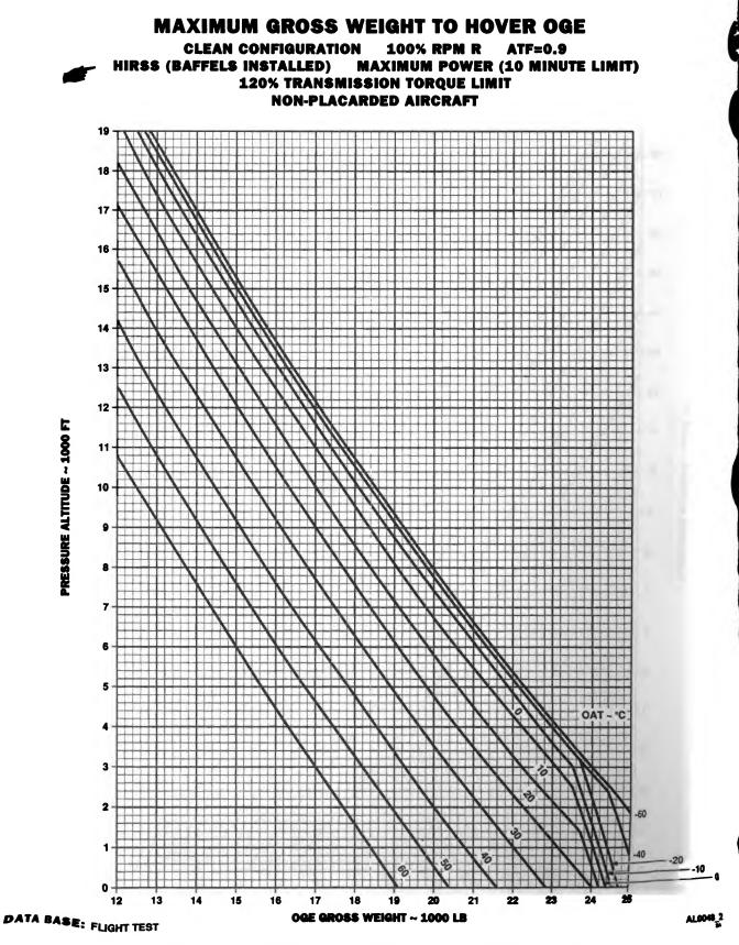
Figure 7.1-6.1.1. Maximum Gross Weight to Hover OGE (Sheet 2 of 2)
