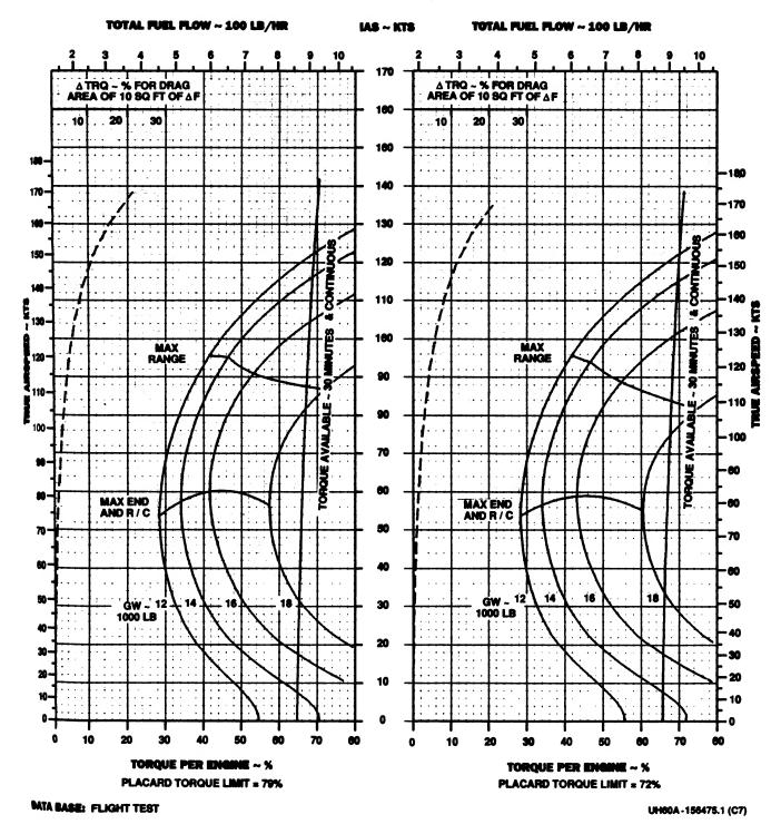
Figure 7.1-18. Cruise - Pressure Altitude 18,000 Feet (Sheet 1 of 4)
