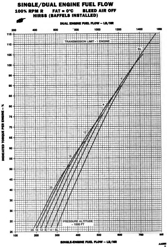
Figure 7-42. Single/Dual-Engine Fuel Flow
