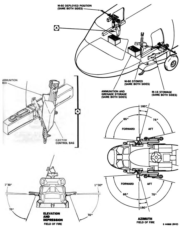
Figure 4-5. Machinegun M60D Installation
