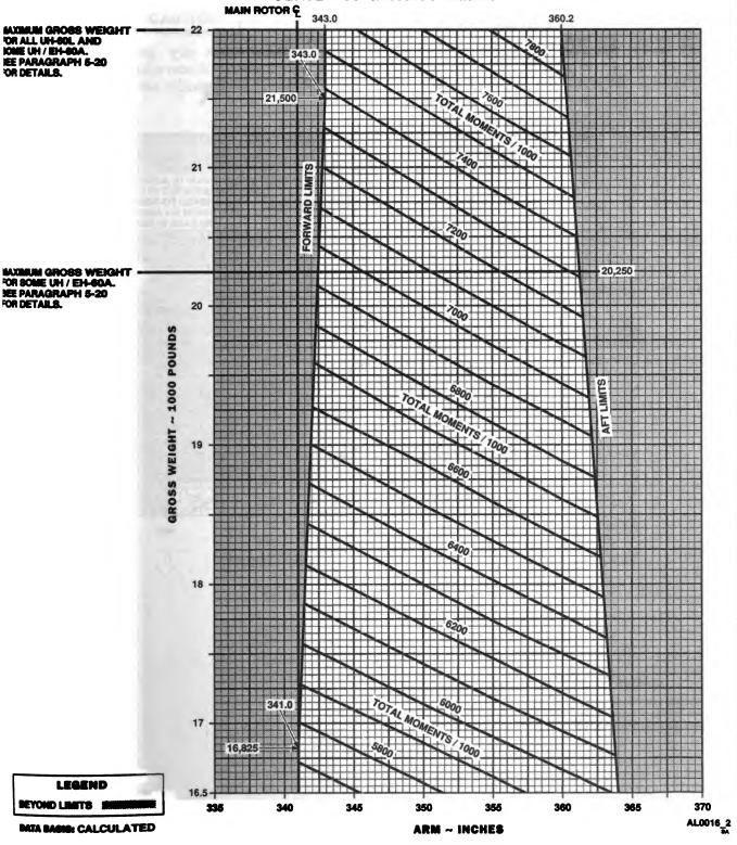
Figure 6-2.1. Center of Gravity Limits Chart (Sheet 2 of 3)
