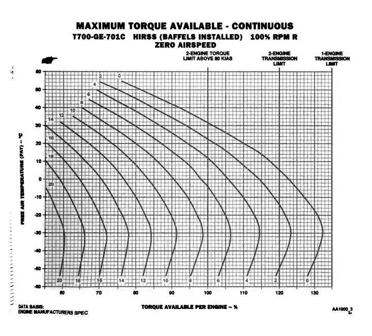
Figure 7.1-3. Maximum Torque Available (Sheet 3 of 3)
