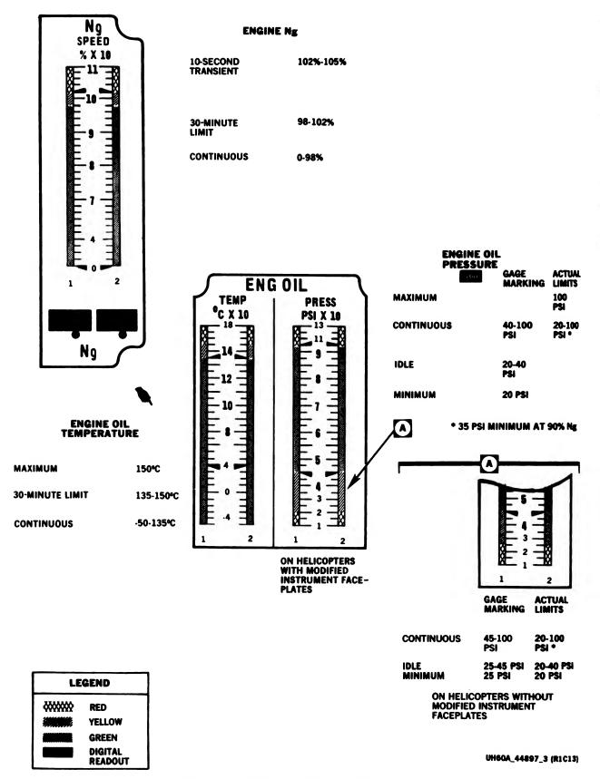
Figure 5-1. Instrument Markings (Sheet 3 of 4)
