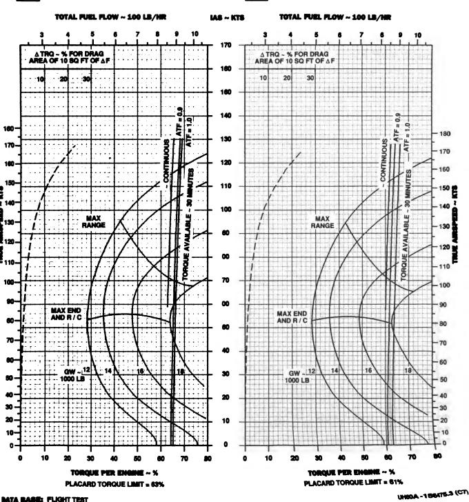
Figure 7.1-18. Cruise - Pressure Altitude 18,000 Feet (Sheet 3 of 4)
