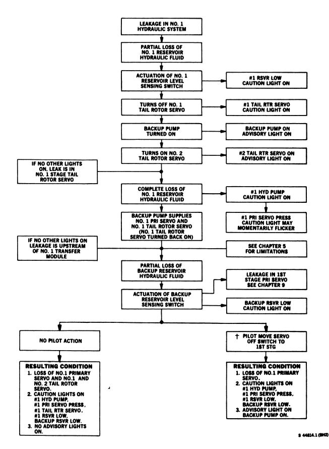
Figure 2-13. Hydraulic Logic Module Operation Principle (Sheet 1 of 2)
