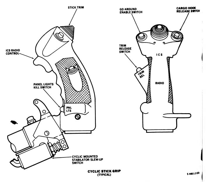
Figure 2-11. Collective and Cyclic Grips (Sheet 2 of 2)
