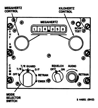
Figure 3-4. VHF Control AN/ARC-115A
