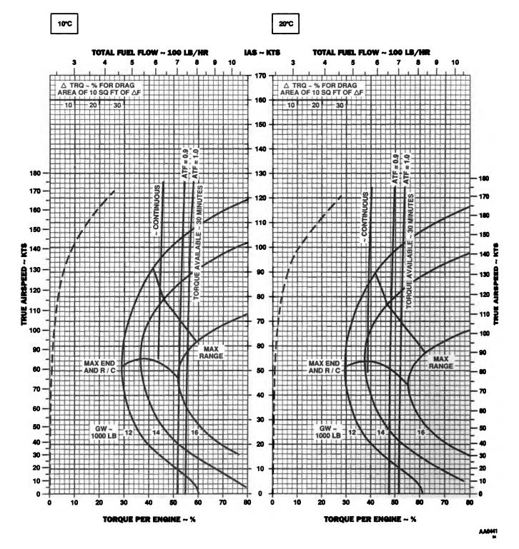
Figure 7-30. Cruise - Pressure Altitude 18,000 Feet (Sheet 4 of 5)
