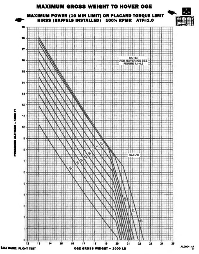
Figure 7.1-6.1. Maximum Gross Weight to Hover OGE - High Drag (Sheet 1 of 2)
