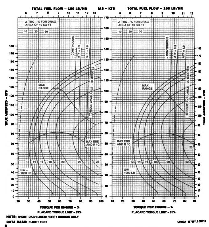
Figure 7.1-13.1. Cruise High Drag - Pressure Altitude 8,000 Feet (Sheet 5 of 6)
