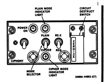
Figure 3-7. Voice Security System Control C-8157/ARC
