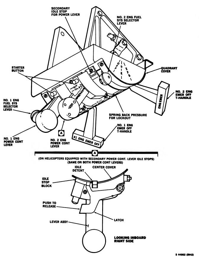
Figure 2-10. Engine Control Quadrant
