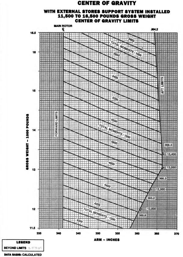
Figure 6-2.1. Center of Gravity Limits Chart (Sheet 1 of 3)
