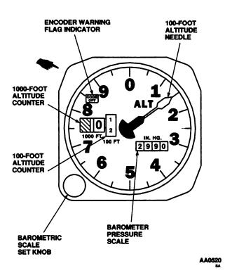
Figure 2-23. Altimeter Encoder AAU-32A
