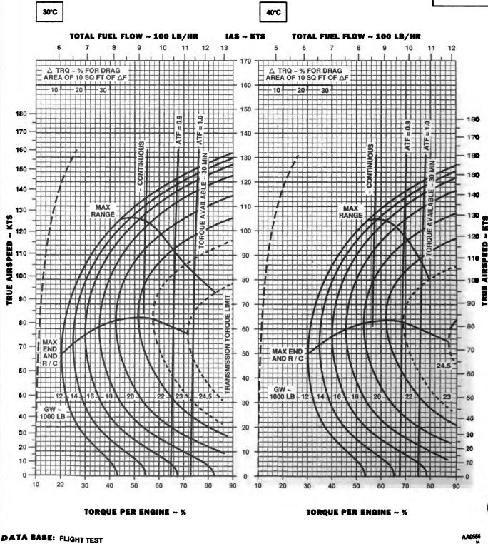
Figure 7-19. Cruise High Drag - Pressure Altitude 6,000 Feet (Sheet 5 of 6)
