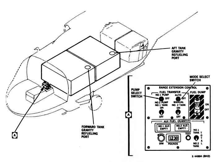
Figure 4-20. Range Extension Control Panel
