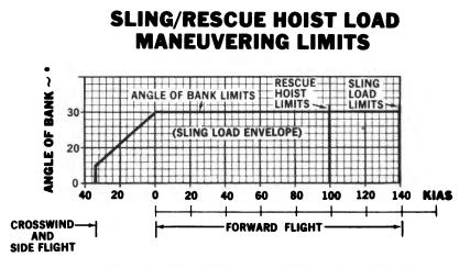
Figure 5-6. Sling/Hoist Load Maneuvering Limitations
