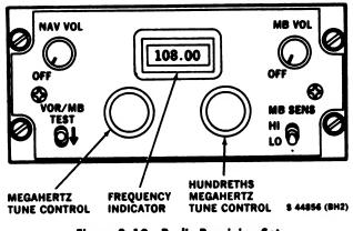
Figure 3-10. Radio Receiving Set AN/ARN-123(V)
