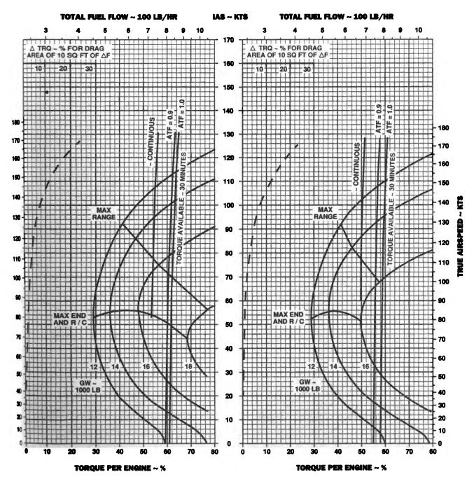
Figure 7-30. Cruise - Pressure Altitude 18,000 Feet (Sheet 3 of 5)
