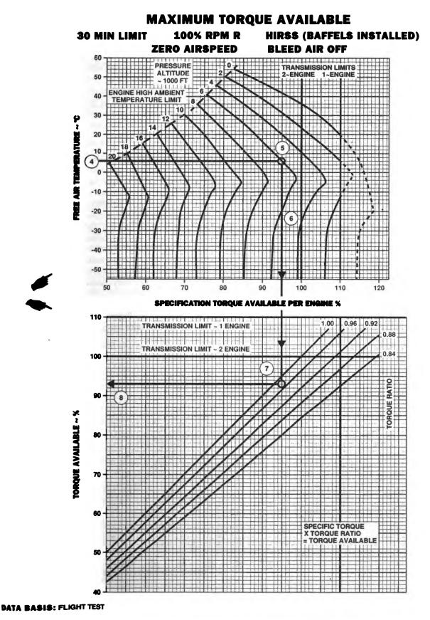
Figure 7-3. Maximum Torque Available - 30-Minute Limit
