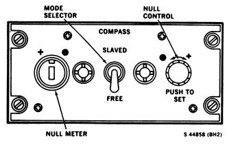
Figure 3-22. Compass Control Panel C-8021/ASN-75
