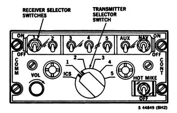
Figure 3-2. Intercommunication Control Panel C-6533/ARC
