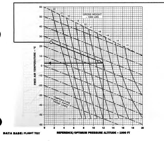
Figure 7-34. Optimum Altitude For Maximum Range (Sheet 1 of 2)
