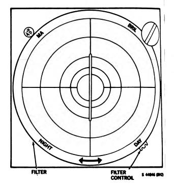
Figure 4-4. Typical Self-Test Mode Display
