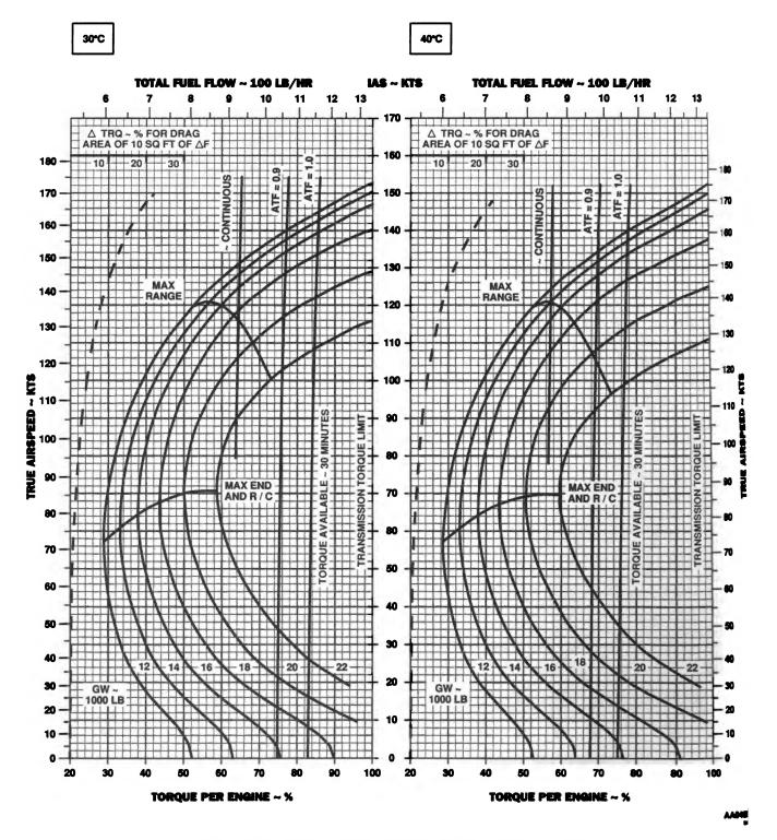
Figure 7-18. Cruise - Pressure Altitude 6,000 Feet (Sheet 5 of 6)
