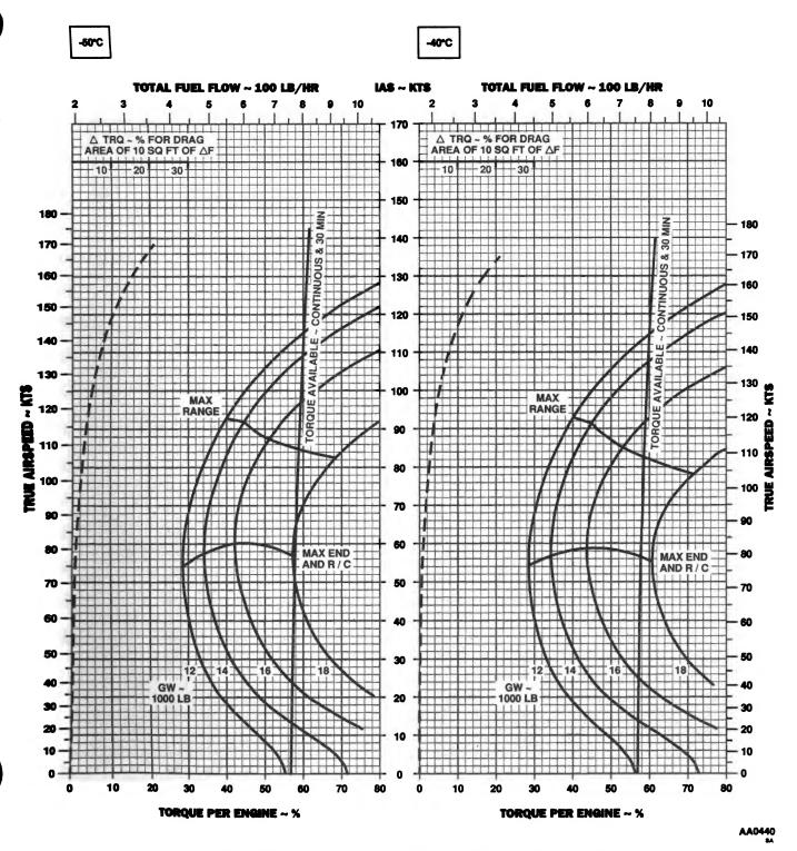
Figure 7-30. Cruise - Pressure Altitude 18,000 Feet (Sheet 1 of 5)
