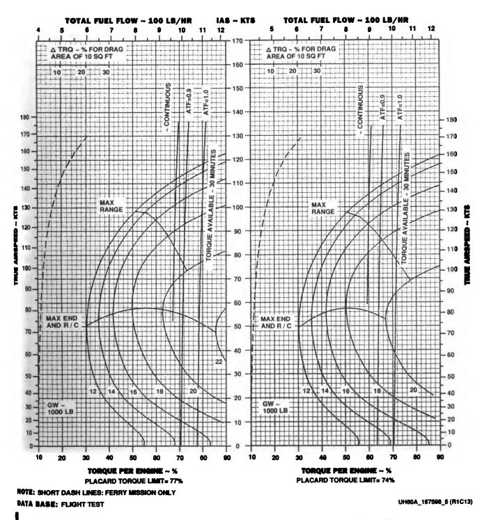
Figure 7.1-14.1. Cruise High Drag - Pressure Altitude 10,000 Feet (Sheet 5 of 5)
