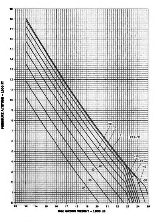
Figure 7.1-6.1.2. Maximum Gross Weight to Hover OGE - High Drag (Sheet 1 of 2)
