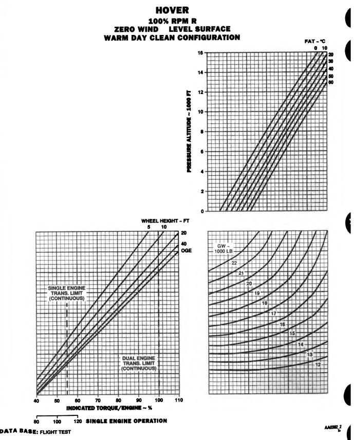
Figure 7-4. Hover - Clean Configuration (Sheet 2 of 2)
