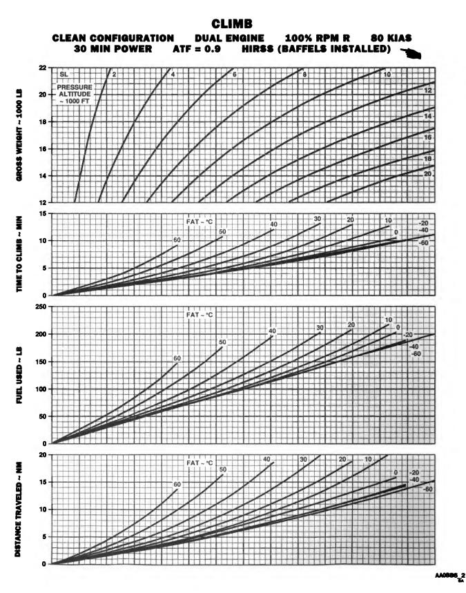
Figure 7-38. Climb - 2 Engine (Sheet 2 of 3)
