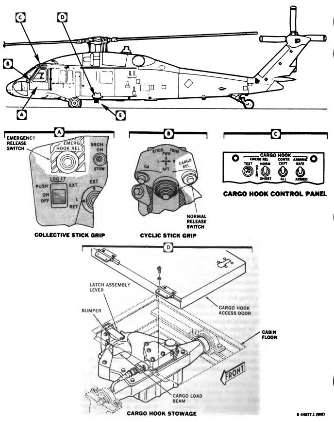
Figure 4-13. Cargo Hook System (Sheet 1 of 2)
