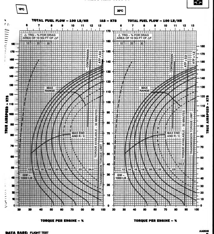
Figure 7-17. Cruise High Drag - Pressure Altitude 4,000 Feet (Sheet 4 of 6)
