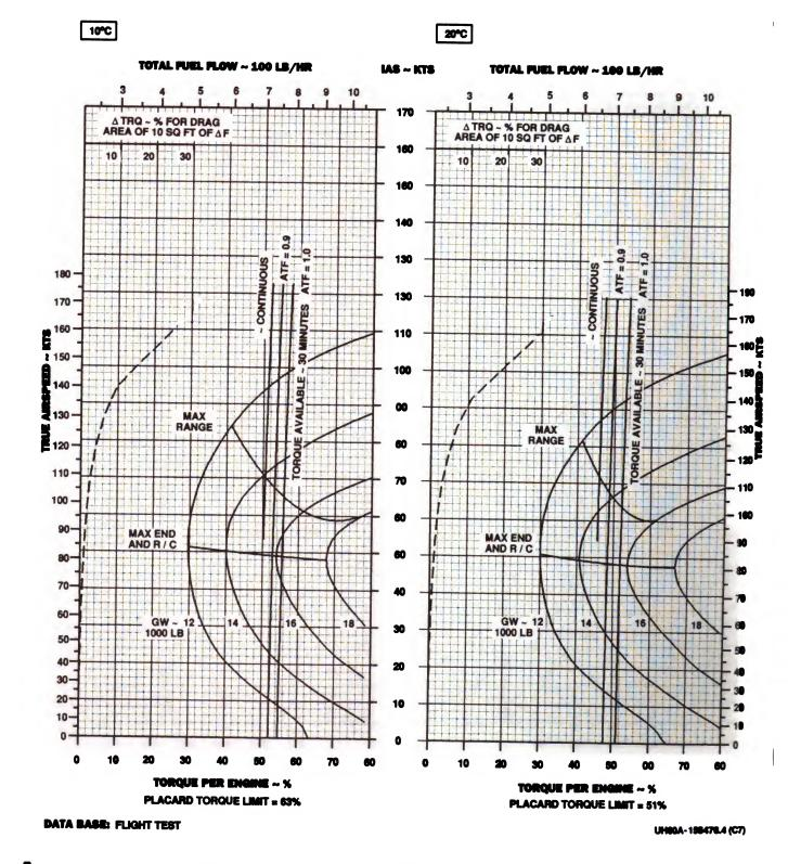
Figure 7.1-19. Cruise - Pressure Altitude 20,000 Feet (Sheet 4 of 4)
