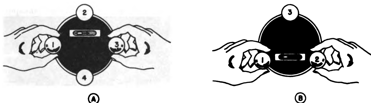
Figure 2-5. Manipulating the leveling screws.
