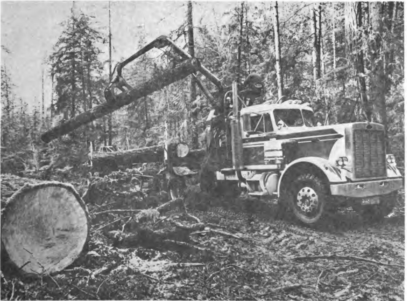
*Figure 7-29. Truck-mounted grapple.*
