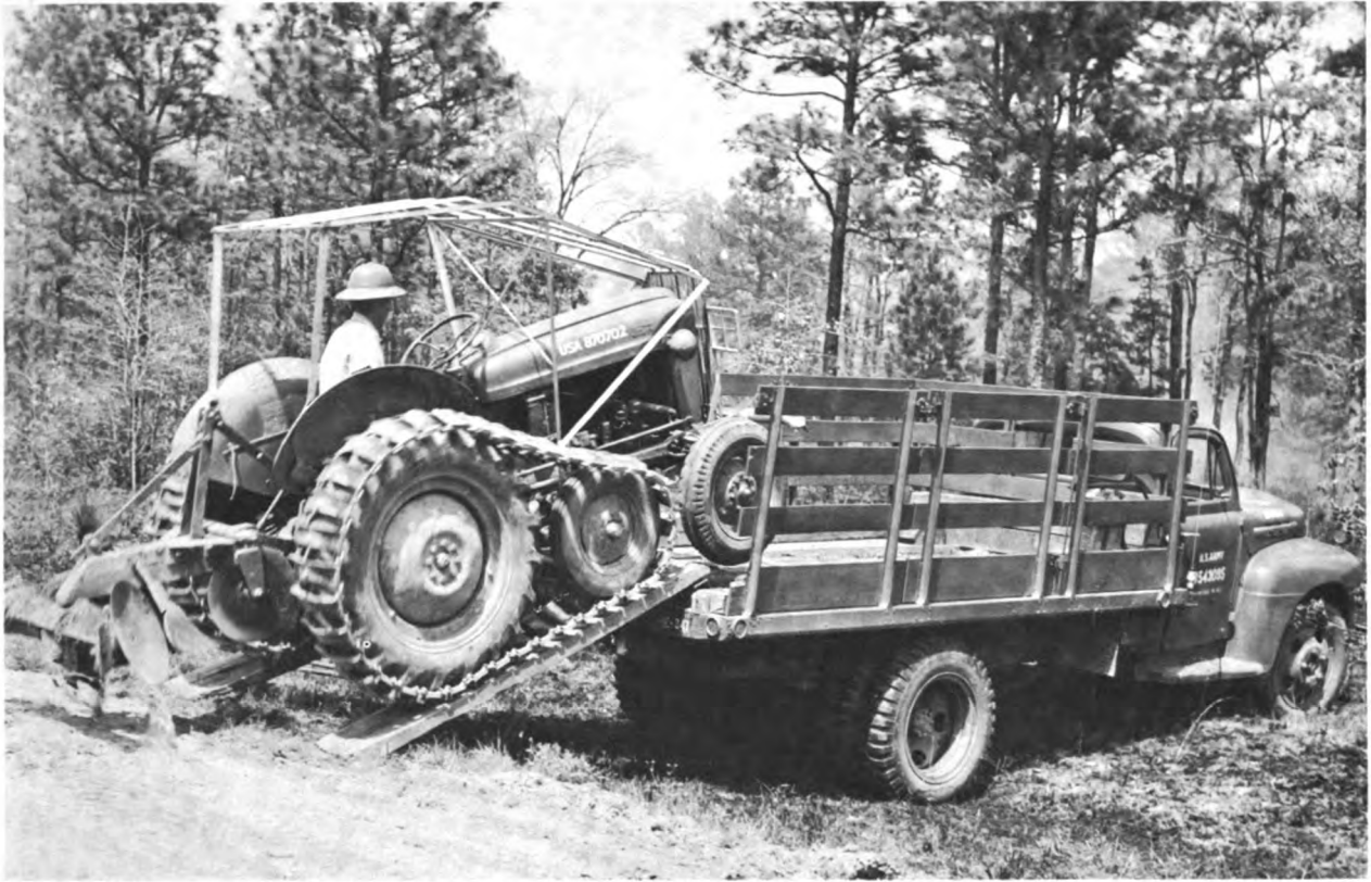
Figure 24. Loading light tractor with fire plow attached. (Note supplemental track.)
