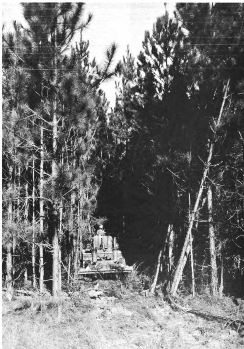
Figure 23. V-bar tree pusher at work. (This tractor is also pulling a fire plow. A brush guard for the driver is lacking.)
