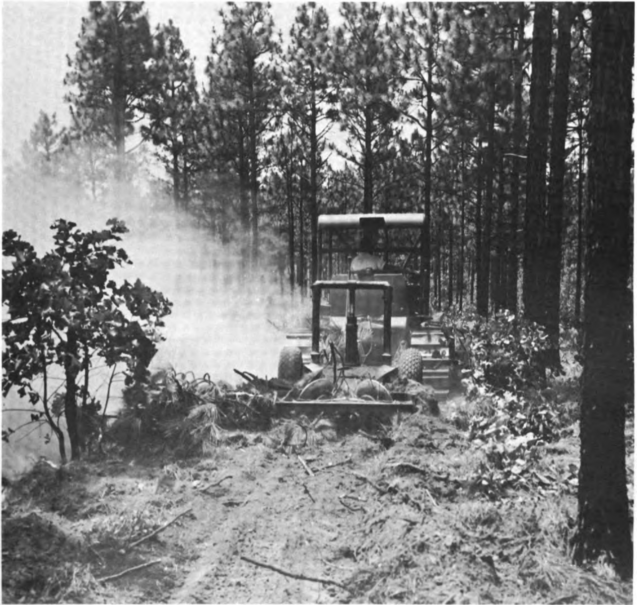
Figure 20. Fire-line construction using heavy fire-line plow.
