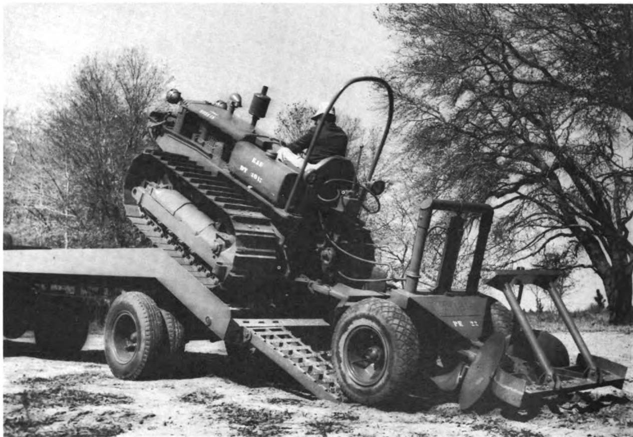
Figure 25. Loading a D-4 unit with two-disk plow attached. (Note 20-inch shoes on tractor.)
