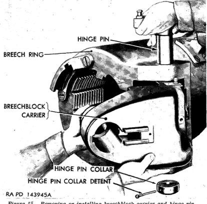
Figure 55. Removing or installing breechblock carrier and hinge pin.
