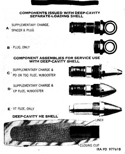
Figure 135. Components used with deep-cavity HE shell.
