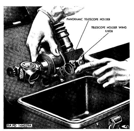
Figure 88. Removing or installing panoramic telescope M12A6 or M12A7G in telescope case.
