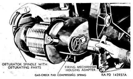
Figure 47. Removing or installing firing mechanism housing adapter, gas-check pad compressing spring, and obturating parts.
