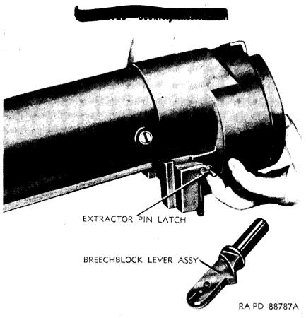
Figure 115. Depressing extractor pin latch.
