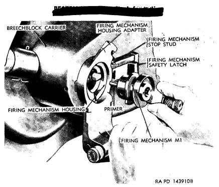
Figure 21. Inserting firing mechanism M1 in firing mechanism housing.
