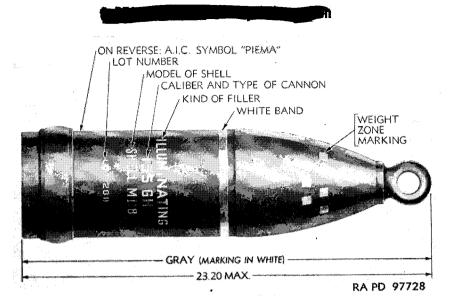
Figure 132. Illuminating shell, M118.
