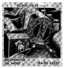
Figure 68. Rear ends of recuperator and counterrecoil cylinders.
