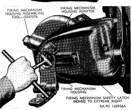
Figure 46. Removing or installing firing mechanism housing.
