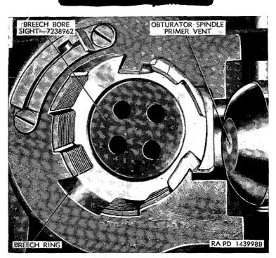
Figure 93. Breech bore sight installed in howitzer breech.
