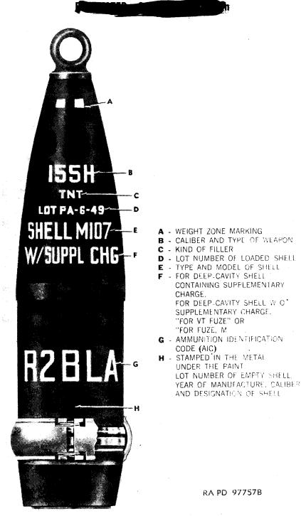
Figure 129. Marking of deep-cavity HE shell.
