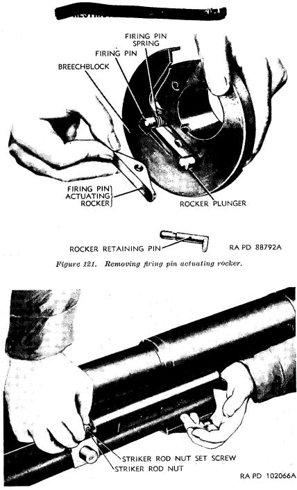
Figure 122. Removing striker rod nut setscrew and nut.
