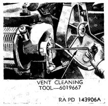
Figure 17. Cleaning primer vent in obturator spindle.
