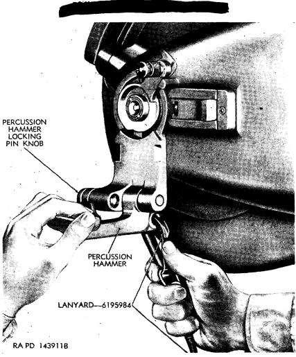
Figure 22. Attaching lanyard to percussion hammer.
