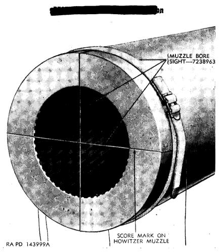
Figure 94. Muzzle bore sight in place on howitzer muzzle.
