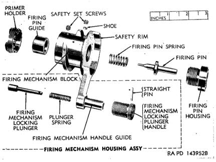
Figure 61. Firing mechanism M1-exploded view.
