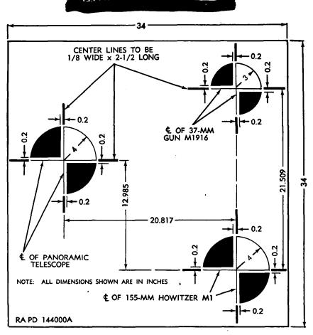
Figure 95. Testing target for boresighting 155-mm howitzer M1 and howitzer mount M14 mounted on motor carriage M41.
