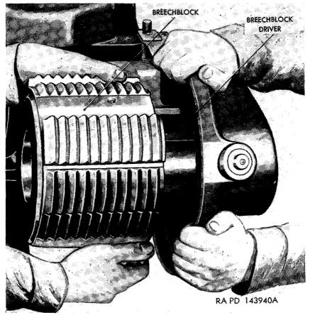
Figure 50. Removing or installing breechblock.
