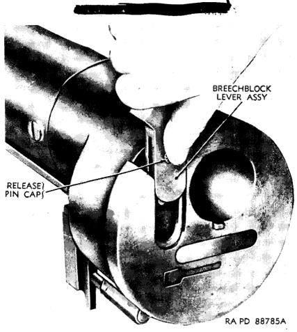
Figure 114. Removal of breechblock lever assembly.
