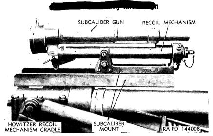
Figure 101. 37-mm subcaliber equipment mounted on howitzer.
