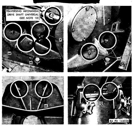
Figure 33. Localized lubrication points-155-mm howitzer mount M14.
