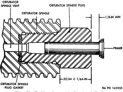
Figure 58. Checking primer seat in obturator spindle plug.
