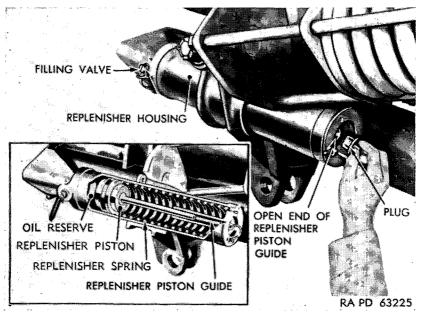
Figure 66. Replenisher-assembled and sectional views.
