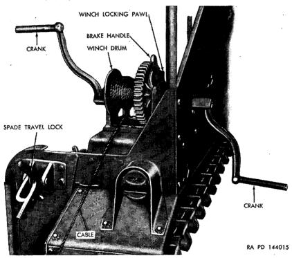
Figure 6. Spade winch and controls.
