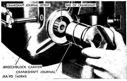
Figure 53. Removing or installing crankshaft journal.
