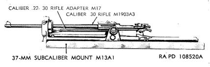
Figure 109. Caliber .30 subcaliber equipment.
