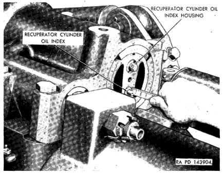
Figure 15. Checking recuperator cylinder oil reserve.
