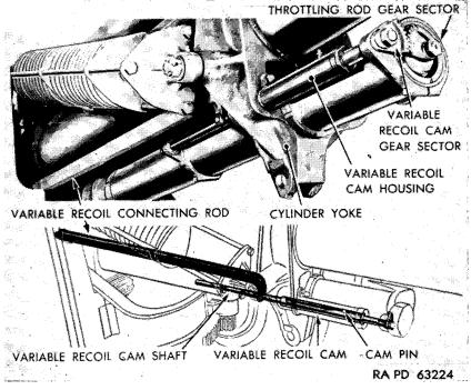
Figure 65. Variable recoil cam-assembled and phantom views.
