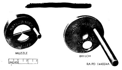
Figure 99. Boresights for 37-mm subcaliber gun M1916.
