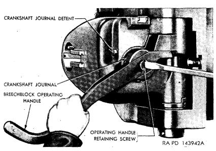
Figure 52. Removing or installing operating handle retaining screw.
