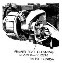
Figure 16. Reaming primer seat in obturator spindle plug.
