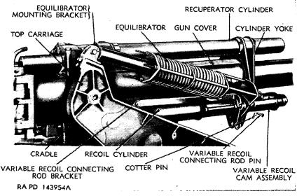
Figure 63. Recoil mechanism in place of mount-right side view.
