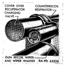
Figure 67. Front ends of recuperator and counterrecoil cylinders.
