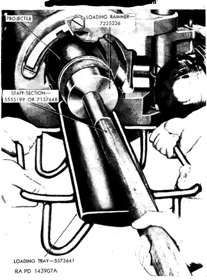
Figure 18. Pushing projectile into breech recess.
