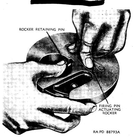
Figure 124. Installing rocker retaining pin.
