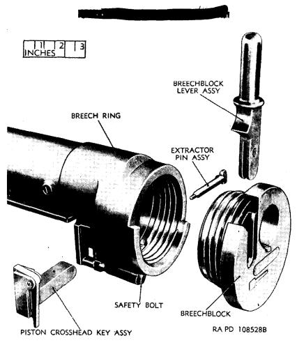
Figure 118. Breechblock-exploded view.
