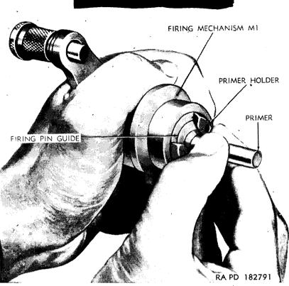
Figure 20. Inserting primer in firing mechanism M1.
