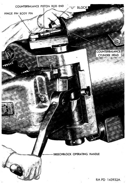
Figure 43. Installing or removing "U" block on counterbalance piston rod.
