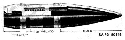
Figure 133. Dummy projectile, M7.
