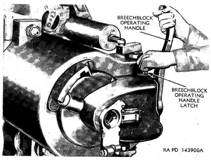
Figure 11. Releasing breechblock operating handle.
