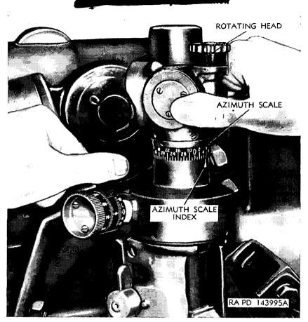
Figure 81. Rapid slewing of rotating head by use of azimuth worm throwout lever.
