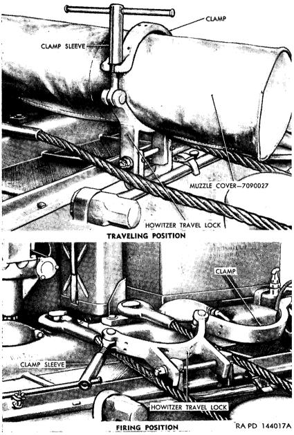
Figure 8. Howitzer travel lock on motor carriage M41.
