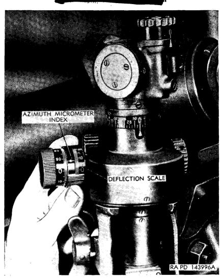
Figure 82. Turning movable azimuth micrometer index to set in constant azimuth deflection.
