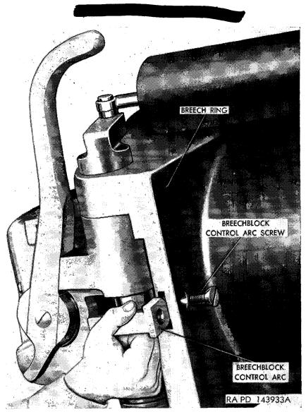
Figure 42. Removing or installing breechblock control arc.
