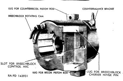
Figure 41. Breech ring-right rear view.
