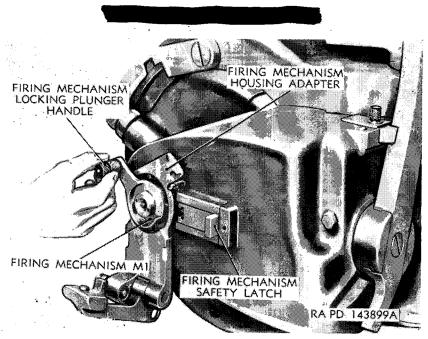
Figure 10. Removing firing mechanism M1 from firing mechanism housing adapter.
