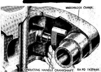
Figure 54. Removing or installing operating handle crankshaft.
