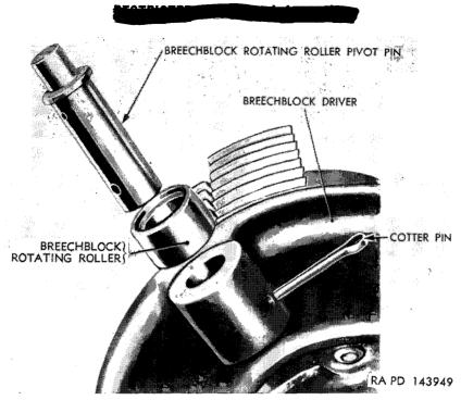
Figure 57. Breechblock rotating roller and pivot pin.
