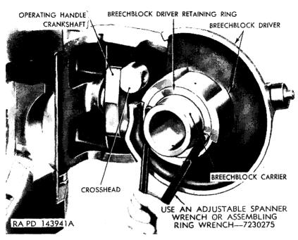
Figure 51. Removing or installing breechblock driver retaining ring.
