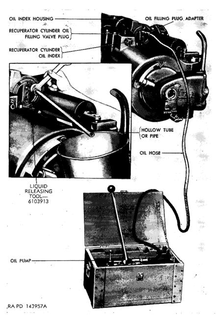
Figure 72. Draining and filling recuperator cylinder.
