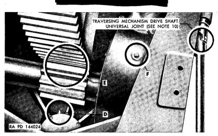
Figure 31. Localized lubrication points—155-mm howitzer mount M14—top carriage well.
