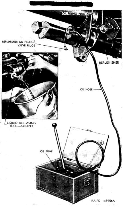
Figure 71. Draining and filling replenisher.
