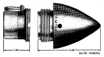
Figure 137. Fuze, CP, M78A1, and Booster, M25.
