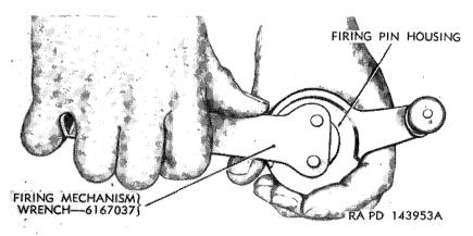
Figure 62. Disassembling or assembling firing mechanism M1
