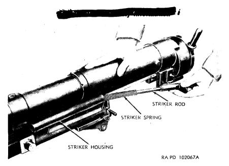
Figure 123. Removing striker rod and spring.
