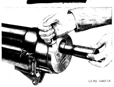
Figure 110. Loading the 37-mm gun.
