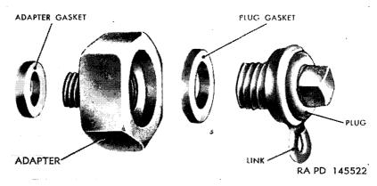
Figure 126. Adapter and components-exploded view.
