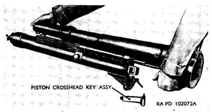
Figure 113. Removing subcaliber gun from recoil mechanism.
