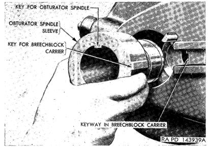
Figure 49. Removing or installing obturator spindle sleeve.
