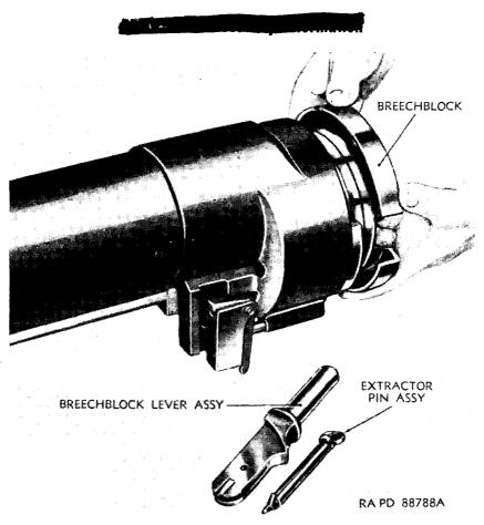
Figure 116. Removal of breechblock.
