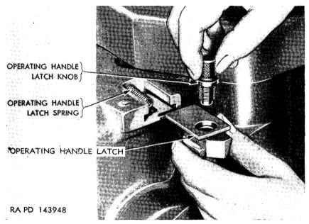
Figure 56. Removing or installing operating handle latch.
