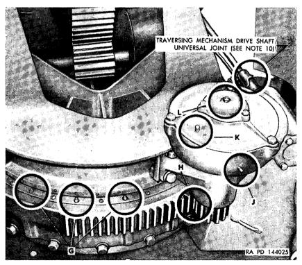
Figure 32. Localized lubrication points-155-mm howitzer mount M14.
