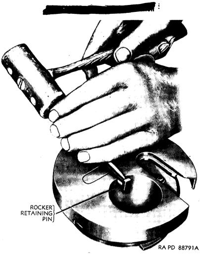
Figure 120. Removing rocker retaining pin.
