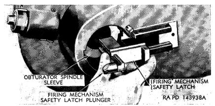
Figure 48. Removing or installing firing mechanism safety latch and plunger.
