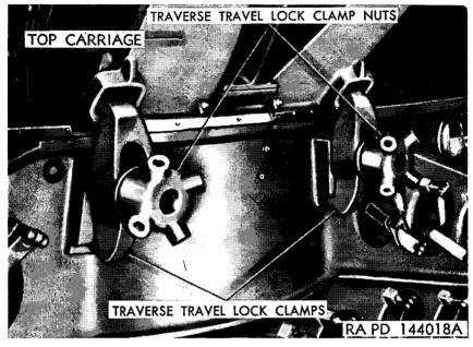
Figure 9. Howitzer mount traverse travel locks on motor carriage M41 traveling position.
