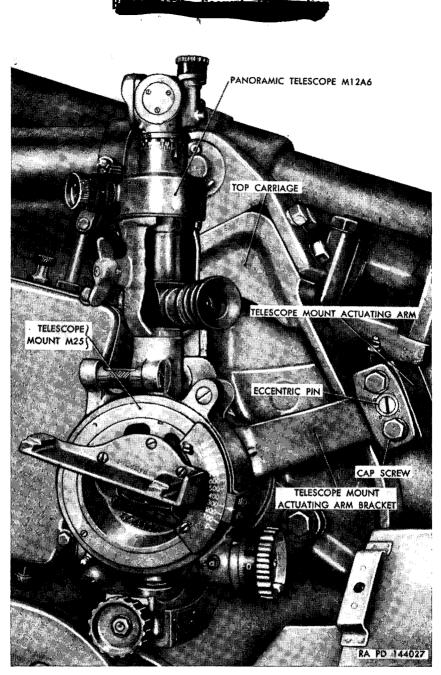
Figure 75. Telescope mount M25 with panoramic telescope M12A6 in place on Mount M14.
