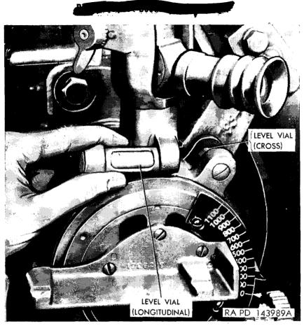
Figure 90. Uncovering longitudinal level vial.
