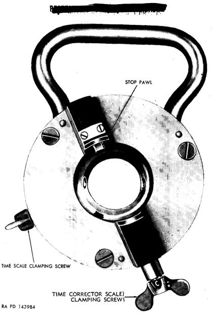
Figure 85. Fuze setter M22 or M23-bottom view.
