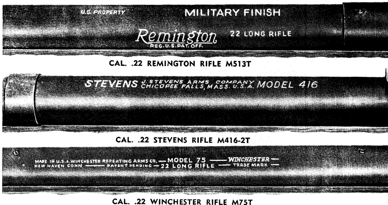
Figure 19. Barrel and receiver identification markings.
