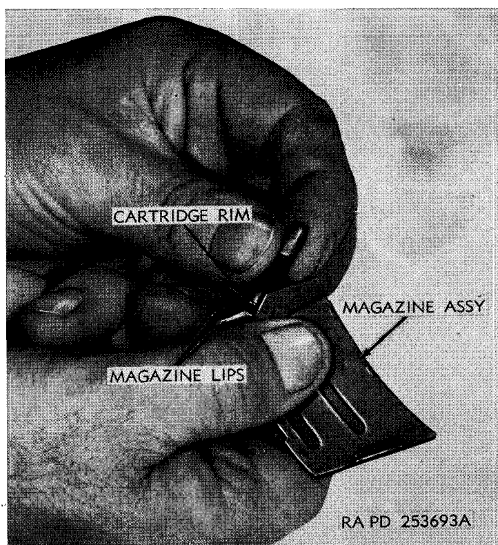
Figure 21. Loading cartridge into magazine assembly (Remington rifle M513T).
