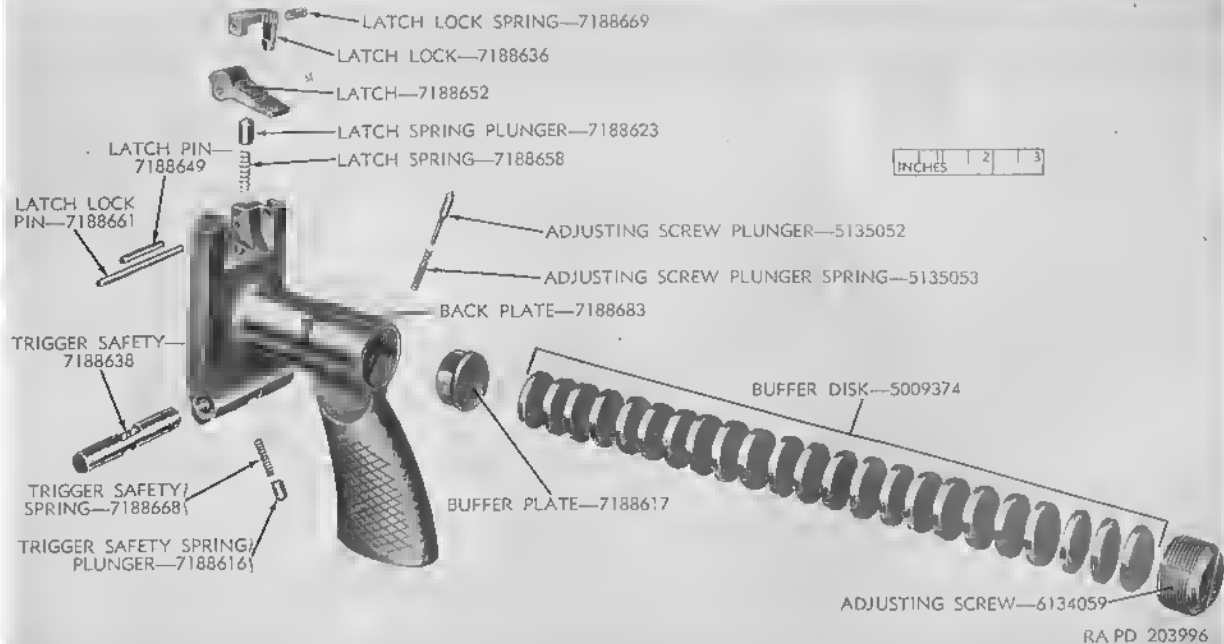
Figure 14. Back plate assembly—exploded view.
