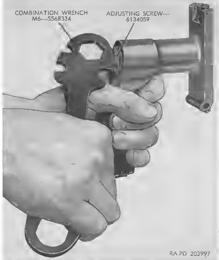
Figure 13. Removing adjusting screw, using combination wrench M6 5568334.
