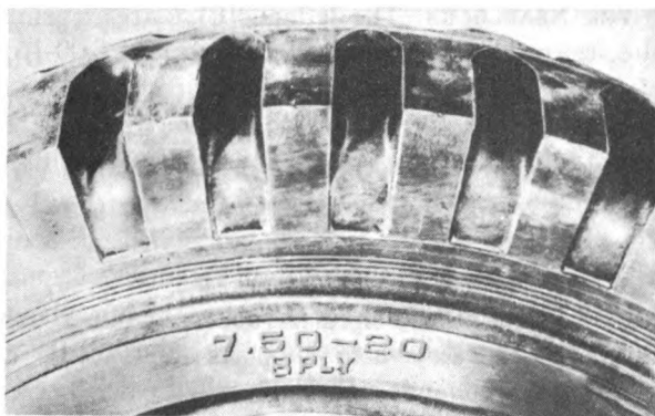
Figure 258. Size and Ply Markings on Tire.
