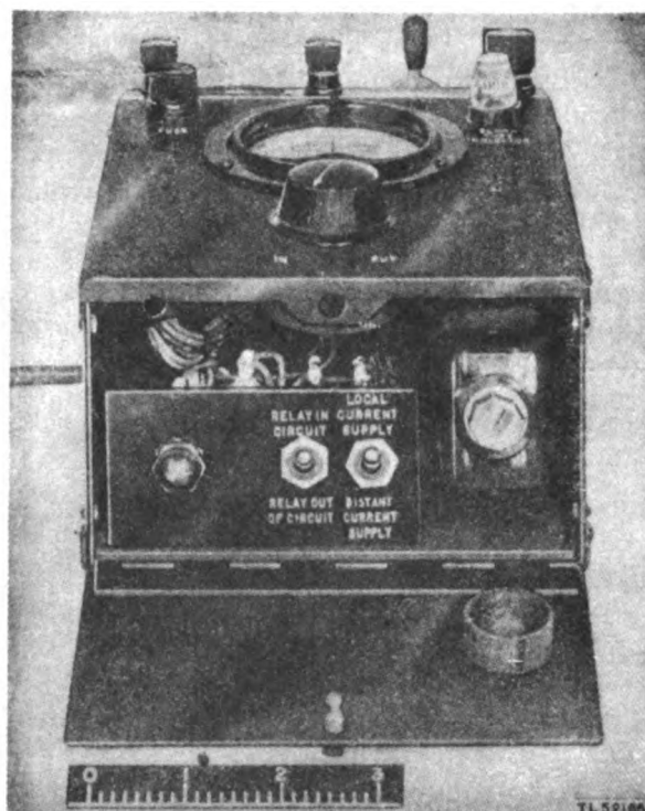
Figure 76. Line Unit BE-77-A, door open.
