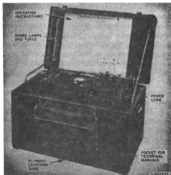
Figure 155. Repeater TG-30 (Terminal, Telegraph) ready for operation.
