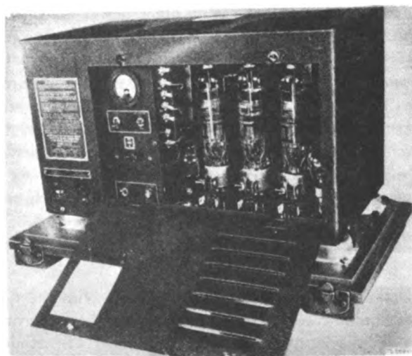
Figure 118. Rectifier RA-43-B, front view.
