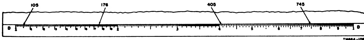
Figure 96. Locating numbers on the D scale.
