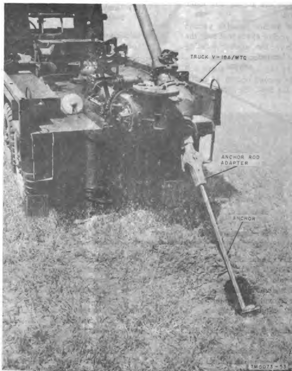
Figure 12. Truck V-18A/MTQ, using boring machine to set anchor.
