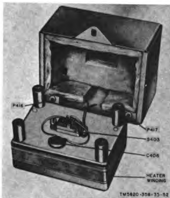
Figure 48. Crystal-oscillator subchassis, internal view of crystal oven.
