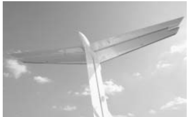
108. ELEVATOR, ELEVATOR TAB, STATIC WICKS (3 EACH SIDE)—CHECKED
