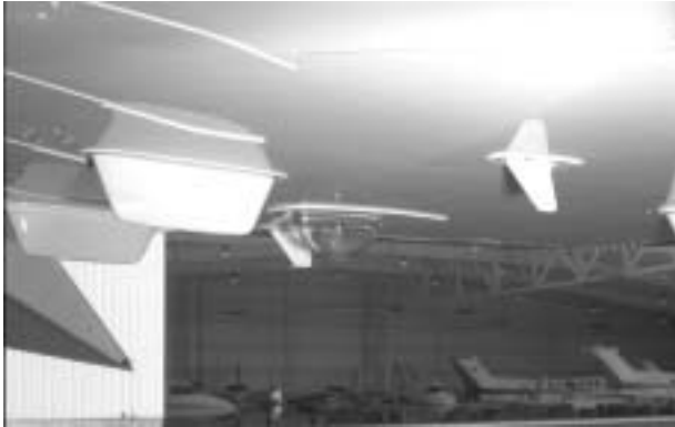
42. LOWER ANTENNAS AND BEACON—CHECKED
