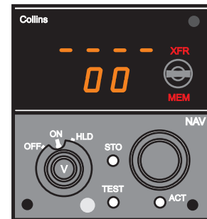
TEST DISPLAY NO FAULT PRESENT
