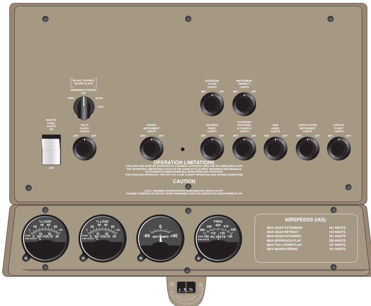
Figure 1-4. Overhead Light Control Panel (BB-1632 and After)
