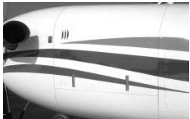
26. ENGINE COMPARTMENT DOOR (OUTBOARD)— SECURE, BLEED VALVE EXHAUST CLEAR
