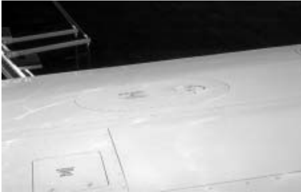
36. AUXILIARY FUEL TANK CAP—SECURE
