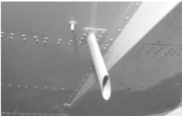
114. AFT COMPARTMENT DRAIN TUBE—CLEAR 115. OXYGEN OVERPRESSURE DRAIN TUBE—CLEAR
