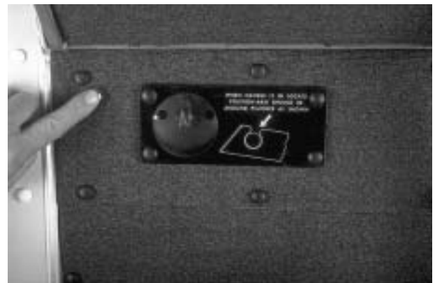
Figure 1-29. Placard and Inspection Port
