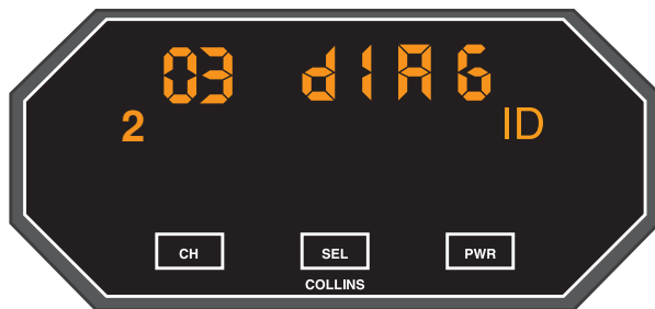
IND-42C SELF-TEST DISPLAY 03 (TRANSMITTER) FAULT FOUND
