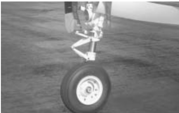
46. NOSE GEAR, DOORS, STRUT, TIRE—CHECKED
