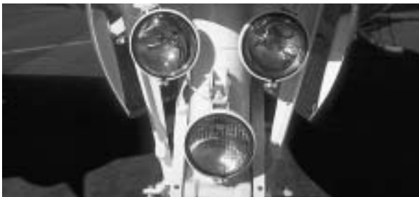
Figure 3-14. Landing and Taxi Lights
