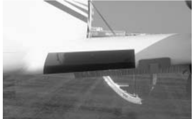
39. INBOARD DEICE BOOTS—CHECKED
