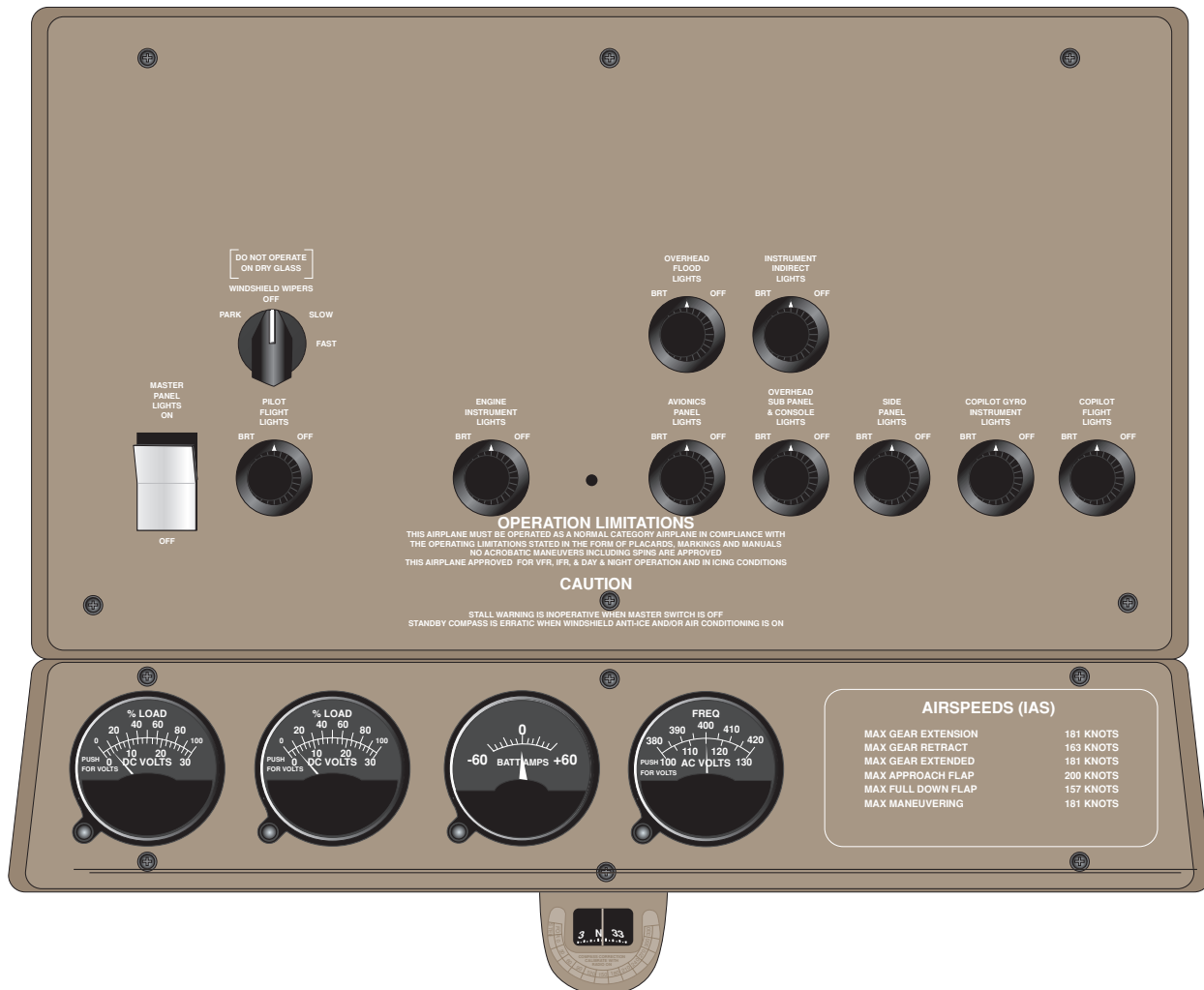
Figure 3-1. Overhead Lighting Controls
