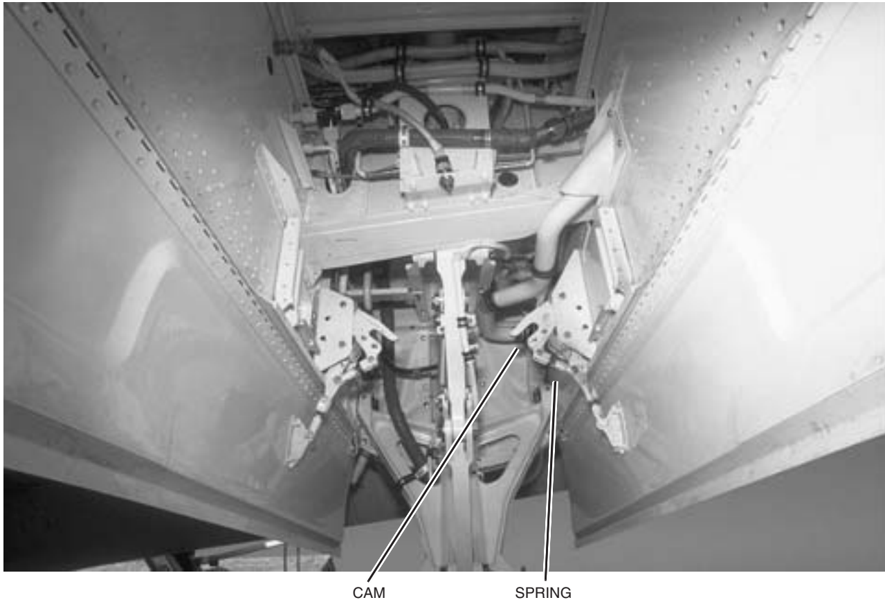
Figure 14-17. Main Gear Door Mechanism (Standard Gear)
