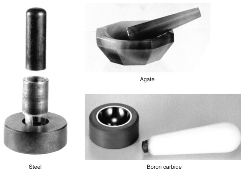
FIGURE 28-5 Steel, agate, and boron carbide mortars and pestles. The mortar is the bowl and the pestle is the grinding tool. The boron carbide mortar is a hemispheric shell enclosed in a plastic or aluminum body. The pestle has a boron carbide button at the tip of a plastic handle. [Courtesy Thomas Scientific, Swedesboro, NJ.]
