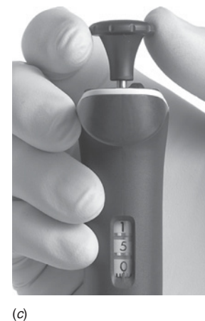
FIGURE 2-14 (a) Micropipet with disposable plastic tip. (b) Enlarged view of disposable tip containing polyethylene filter to prevent aerosol from contaminating the shaft of the pipet. (c) Volume selection dial set to 150 \mu\text{L} . [Courtesy of Rainin Instrument, LLC, Oakland, CA.]
