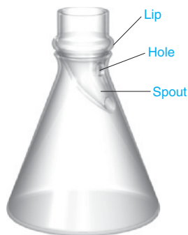
FIGURE 28-11 Reflux cap for wet ashing in an Erlenmeyer flask. The hole allows vapor to escape. The curved spout touches the inside of the flask. [Information from D. D. Siemer and H. G. Brinkley, "Erlenmeyer Flask-Reflux Cap for Acid Sample Decomposition," Anal. Chem. 1981 , 53, 750.]
