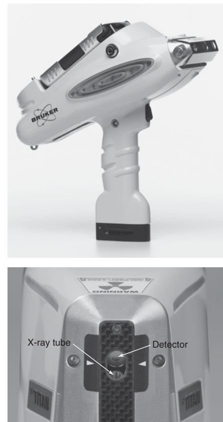
FIGURE 21-33 Handheld X-ray fluorescence analyzer for field analysis. Close-up shows proximity of X-ray tube and fluorescence detector. [Courtesy Bruker Elemental.]
