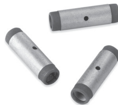
FIGURE 21-6 Pyrocoated graphite tubes family. Electrically heated graphite furnace tubes for atomic spectroscopy, typically 38-mm long. Graphite is coated with a thin layer of pyrolytic carbon to reduce porosity of the surface. [© PerkinElmer, Inc. All rights reserved. Printed with permission.]
