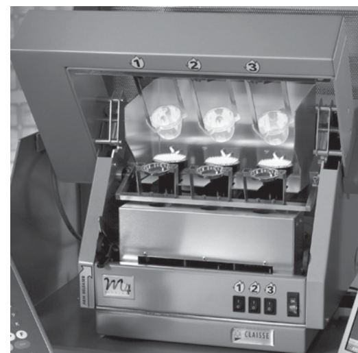
FIGURE 28-8 Automated apparatus that fuses three samples at once over propane burners. The Pt/Au crucibles rotate while they are inclined. [Courtesy Claissé, Quebec.]
