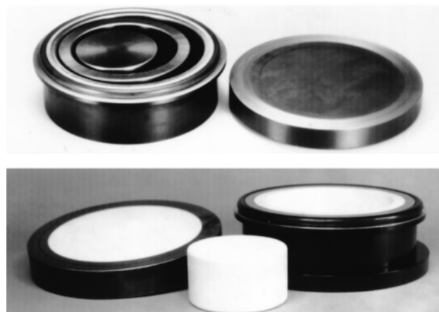
FIGURE 28-6 Shatterbox laboratory mill spins a puck and ring inside a container at high speed to grind up to 100 mL of sample to a fine powder. [SPEX SamplePrep LLC.]
