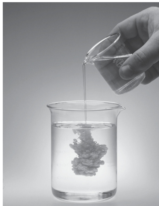
FIGURE 6-2 A yellow solid, lead(II) iodide ( \text{PbI}_2 ), precipitates when a colorless solution of lead nitrate ( \text{Pb}(\text{NO}_3)_2 ) is added to a colorless solution of potassium iodide ( \text{KI} ). [© 1989 Chip Clark – Fundamental Photographs.]
