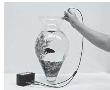
FIGURE 19-25 Fiber-optic sensor measures \text{O}_2 by its ability to quench the luminescence of \text{Ru(II)} at the tip of the fiber. A blue-light-emitting diode provides excitation energy. [© Courtesy Ocean Optics, Dunedin, FL/Ocean Optics, Inc.]
