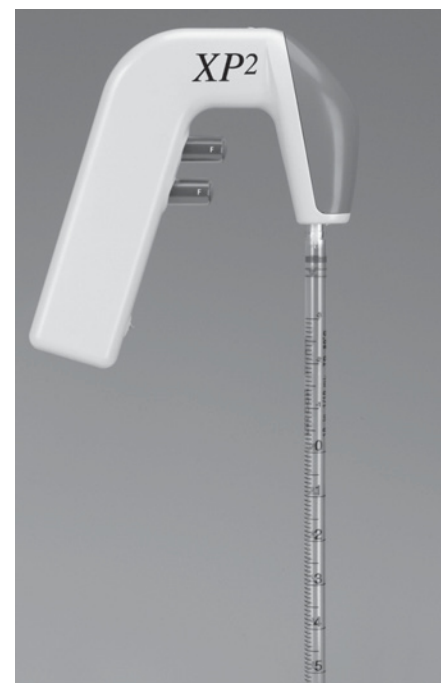
FIGURE 2-13 Electronic Pipet-Aid® allows you to fill the pipet by pressing the top button and to drain the pipet by pressing the lower button. To protect the device and to avoid contamination of solutions, a filter in the nosepiece immediately above the glass pipet ceases to pass air in either direction if the filter gets wet. [Courtesy Drummond Scientific Co., Broomall, PA.]
