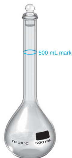
FIGURE 1-4 A volumetric flask contains a specified volume when the liquid level is adjusted to the middle of the mark in the thin neck of the flask. Use of this flask is described in Section 2-5.
