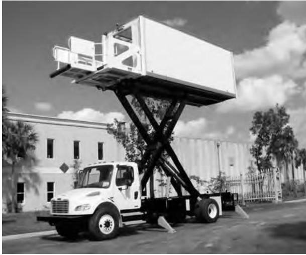
Figure 4.12 High lift to Load Catering Equipment On Board the Aircraft
