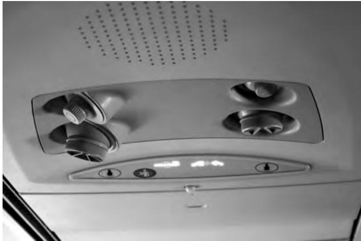
Figure 4.8 Passenger Service Unit (PSU)
