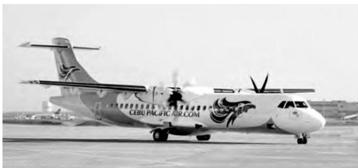
Figure AC.14 ATR 72 Moving Out with One Engine Power
