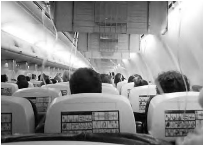
Figure 4.9 Oxygen Masks Dropping Down from PSU
