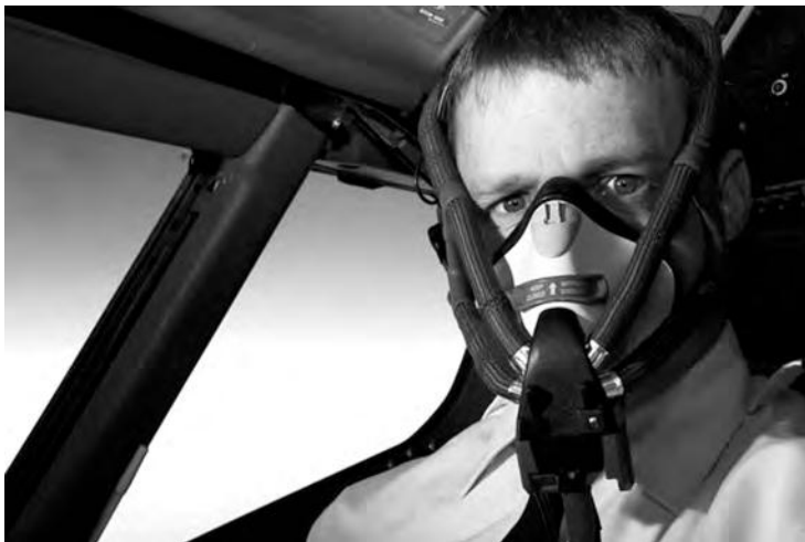
Fig. 7.11 Cockpit crew's quick-donning mask
