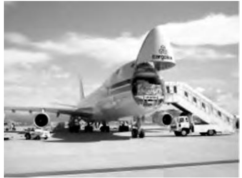
Figure AB.5 Cargolux B747-400F with the Nose Cone Loading Door open
