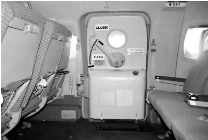
Figure. 4.5 Cabin Door with Chute Pack
