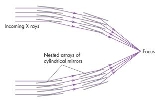
**B** Cross-sectional view of the grazing-incidence mirrors showing how they focus X rays
