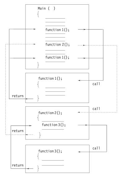
Fig. 8.2 Flow of control in a multi-function program
