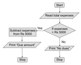
Fig. 2.4 Flow chart representation of an algorithm
