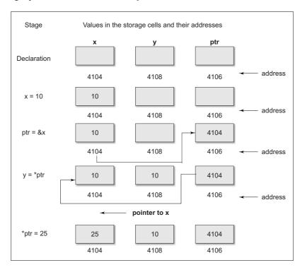
Fig. 12.6 Illustration of pointer assignments
