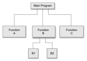
Fig. 8.1 Top-down modular programming using functions
