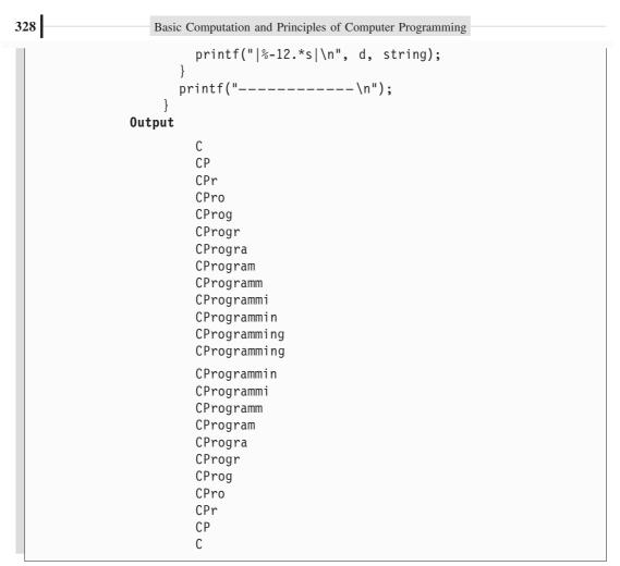
Fig. 11.5 Illustration of variable field specifications by printing sequences of characters
