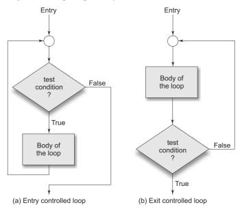
Fig. 7.1 Loop control structures
