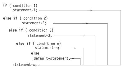
This construct is known as the **else if** ladder. The conditions are evaluated from the top (of the ladder), downwards. As soon as a true condition is found, the statement associated with it is executed and the control is transferred to the statement-x (skipping the rest of the ladder). When all the n conditions become false, then the final **else** containing the *default-statement* will be executed. Figure 6.9 shows the logic of execution of **else if** ladder statements.
