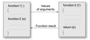
Fig. 8.8 Two-way data communication between functions
