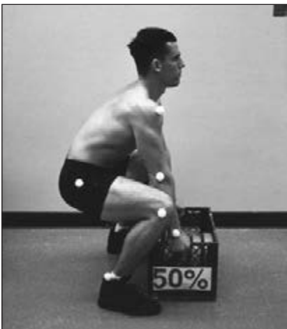
Reflective joint markers can be tracked by a camera for automatic digitizing of the movement.
